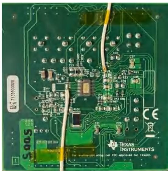
**Figure 3-2. TPS7H5005-SEP SEE Test Board Top View**
