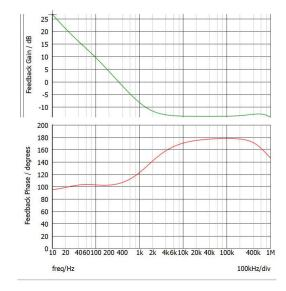
Figure 4-1. Compensator without Amplifier
