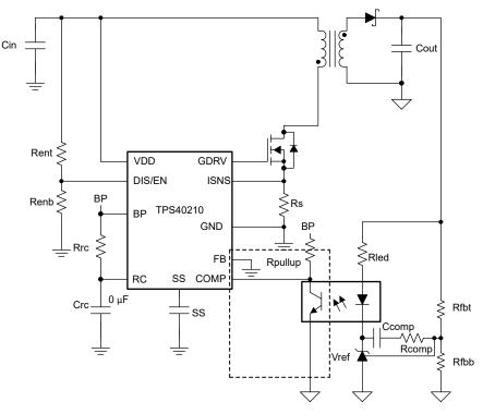
Figure 3-1. Feedback Implementation of Secondary Side Regulation
