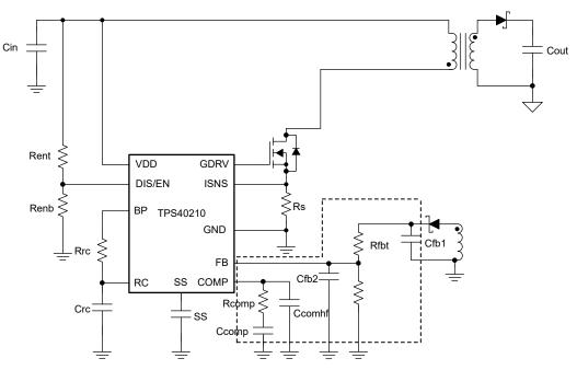
Figure 2-1. Primary Side Regulation Block Diagram
