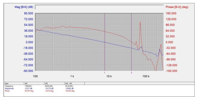
Figure 5-1. Loop Bode Plot without Amplifier
