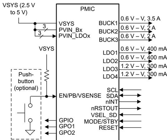
Figure 2-1. TPS65219-Q1 Simplified Schematic
