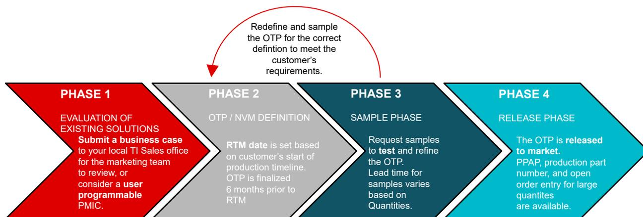
Figure 3-1. Custom Programmed PMIC Design Process
