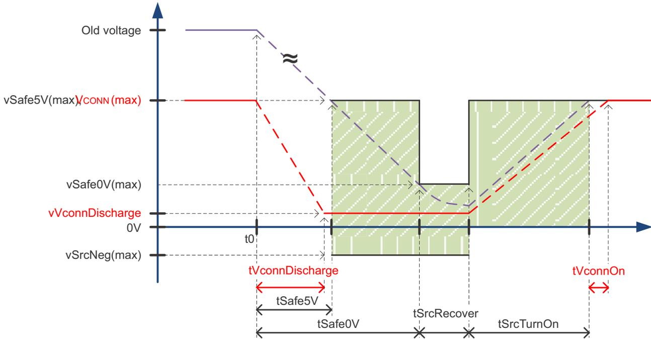
Figure 4-3. Source VBUS and VCONN Response to Hard Reset
