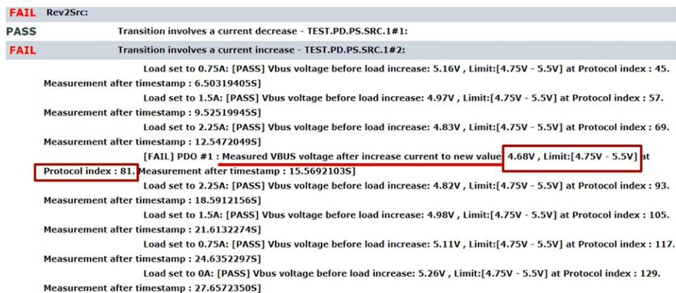
Figure 5-5. XML data log of TEST.PD.PS.SRC.1
