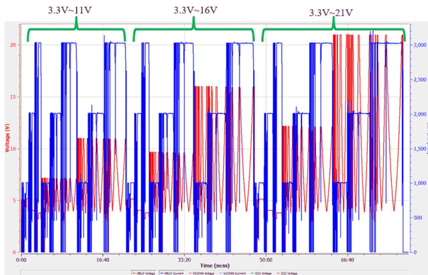
**Figure 4-8. SPT.7 Total-Phase Analyzer Data Log**
