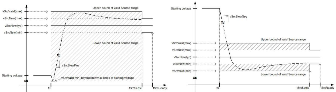
**Figure 4-1. Fixed Supply Voltage Transition**
