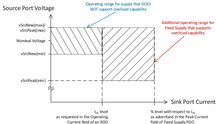
**Figure 4-5. PPS Positive Voltage Transitions**
