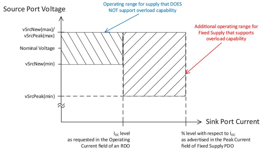
**Figure 4-4. Source Peak Current Overload**
