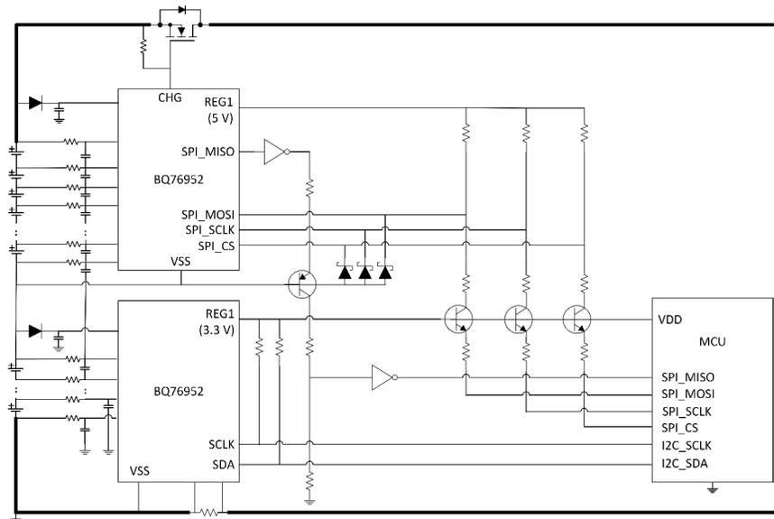
**Figure 5. Serial Communication in a Stacked Design with BQ76952 Battery Monitors**
