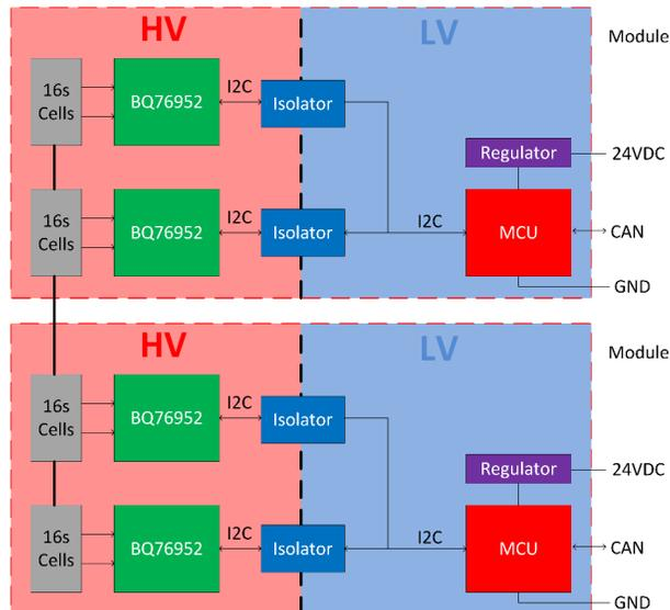
**Figure 2. Stacking Configuration with an Isolated BQ76952 to CAN**
