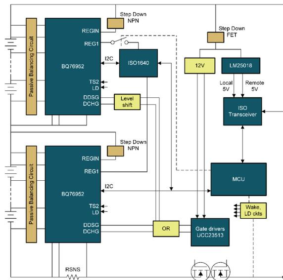
**Figure 3. Stacking Configuration with BQ76952 Battery Monitors**
