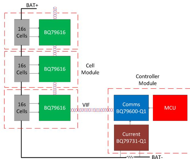
Figure 1. Typical daisy-chain configuration using the BQ79616
