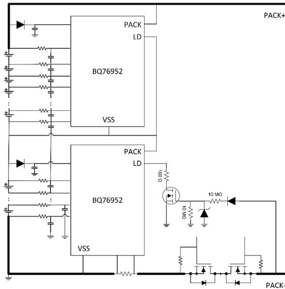
**Figure 6. Load Detection in a Stacked Configuration with BQ76952 Battery Monitors**
