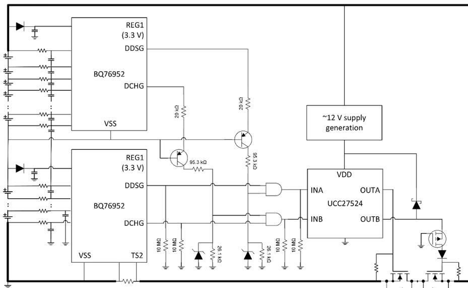
**Figure 4. Combined Protection Design for BQ76952 Battery Monitors**
