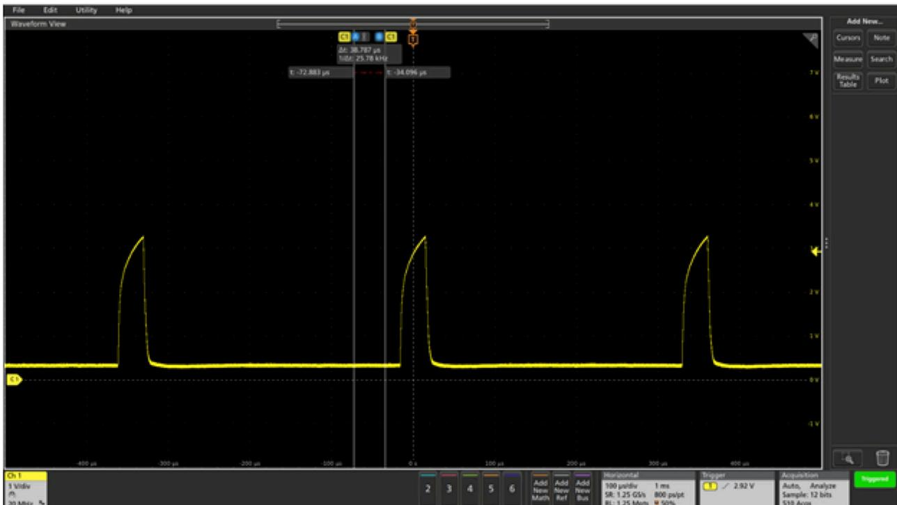
Figure 3-5. Bench Test With 10nF C<sub>sink</sub> and 150 Ω R<sub>sink</sub>
