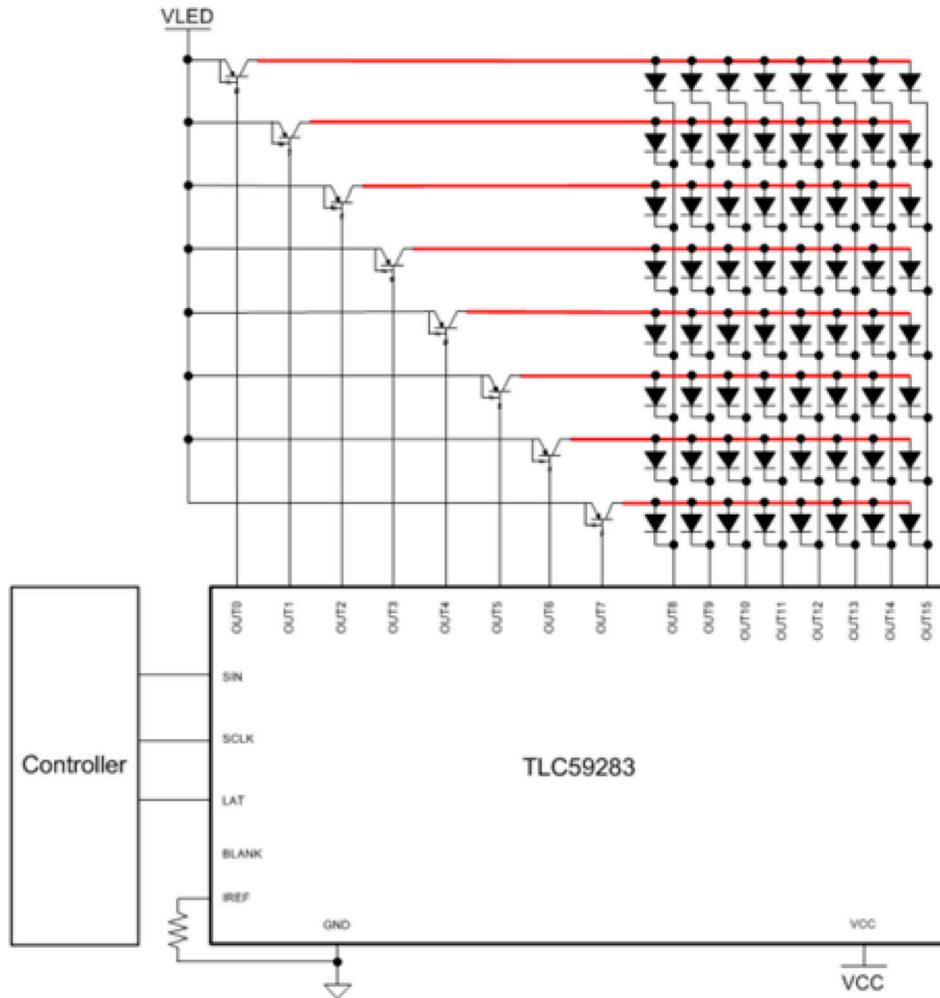
**Figure 1-1. Time-Multiplexing Circuit Using TLC59283 With Less MCU I/Os**
