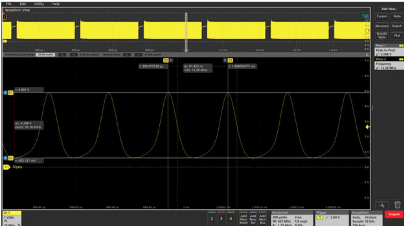
Figure 3-1. Bench Test Without R<sub>sink</sub> and C<sub>sink</sub>
