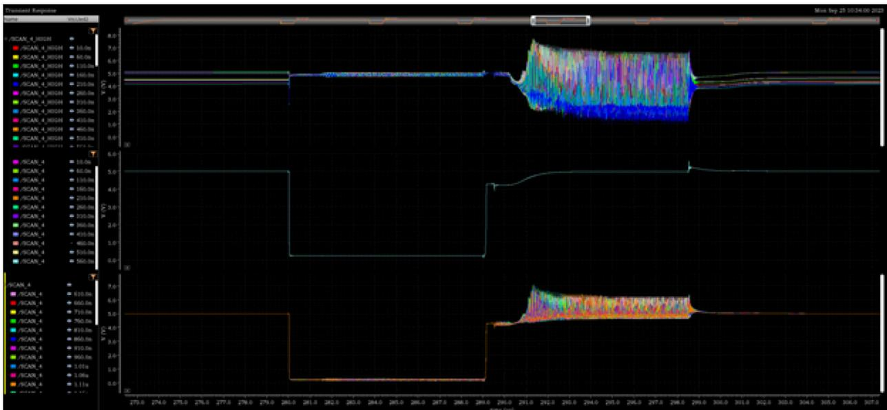
Figure 2-4. Only add L\_LED2 without C\_sink in Parasitic Inductance
