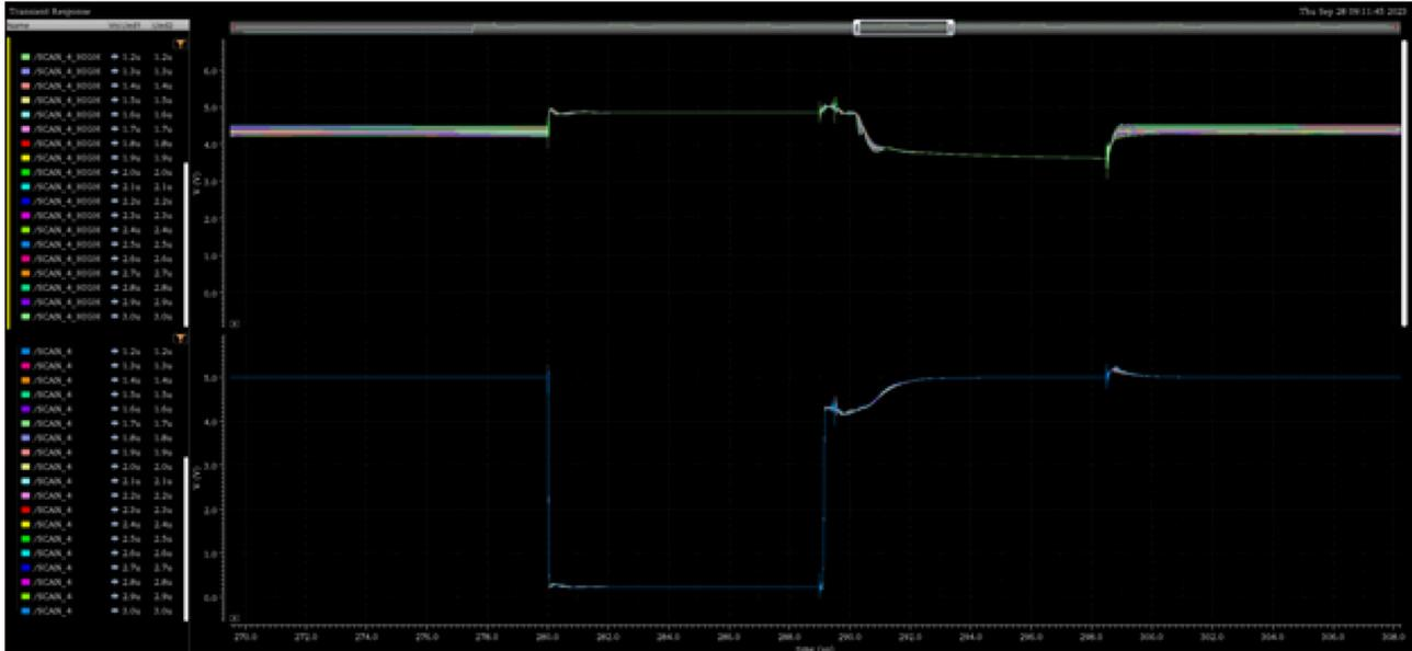
Figure 2-11. Parasitic Inductance of Vin and GND on Customer's Board with C<sub>sink</sub>
