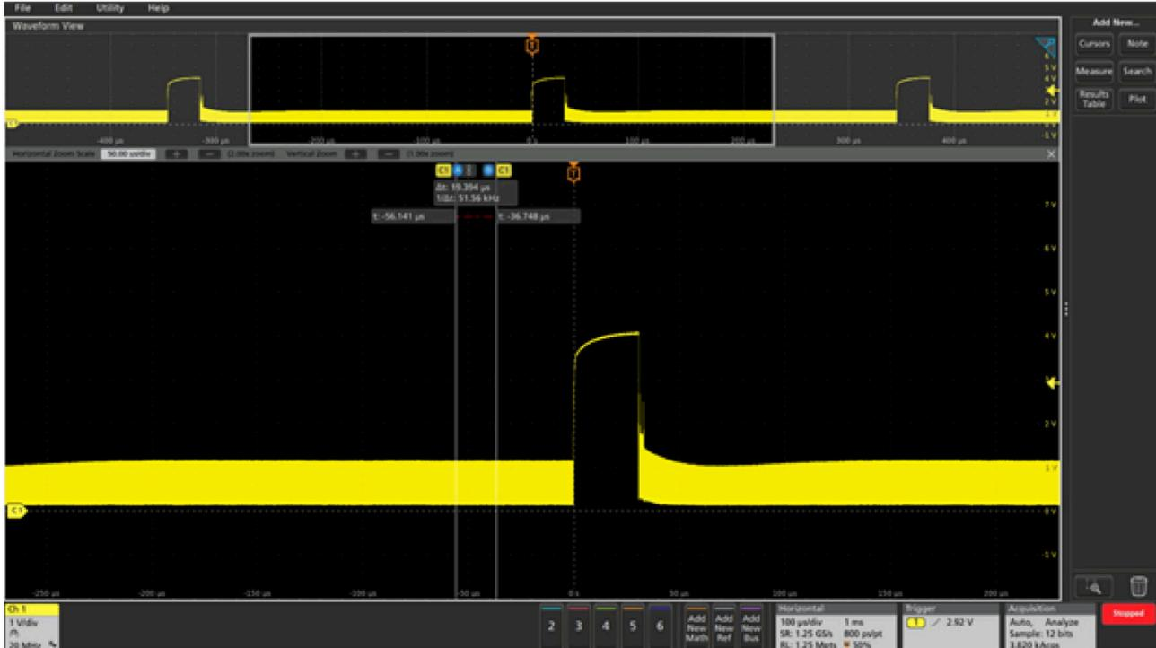
Figure 3-4. Bench Test With 150 Ω R<sub>sink</sub>
