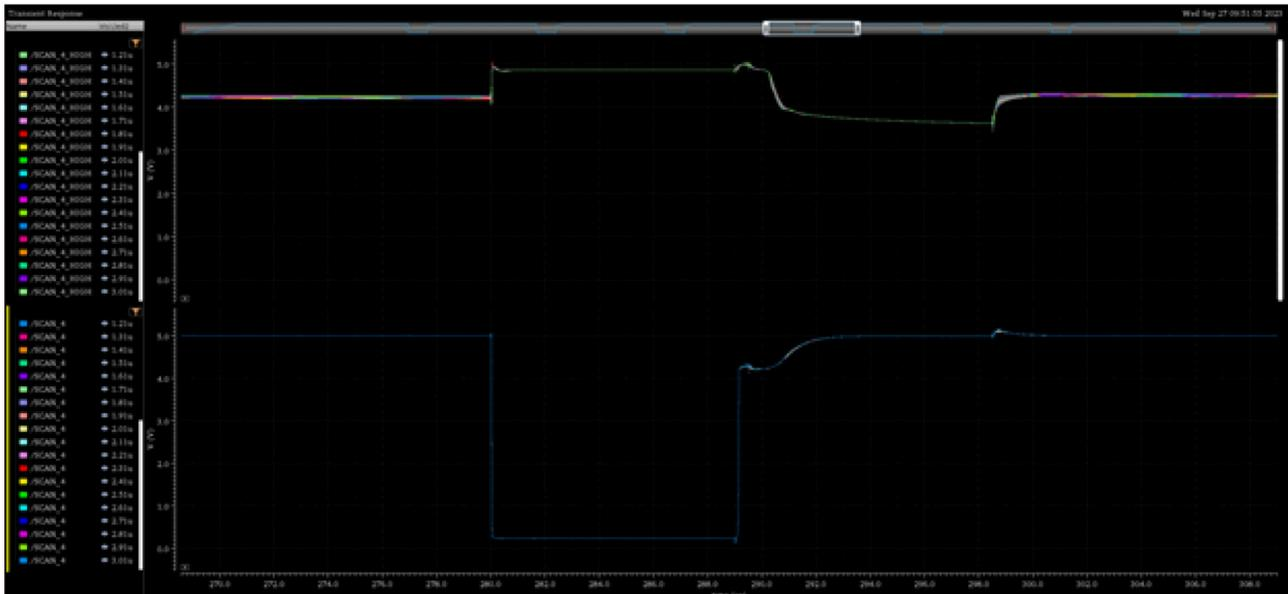
Figure 2-6. Only Add L\_LED2 With C\_sink in Parasitic Inductance
