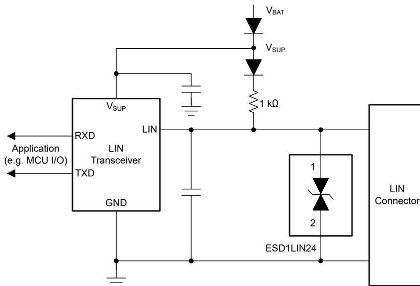
**Figure 3. LIN Placement Diagram**
