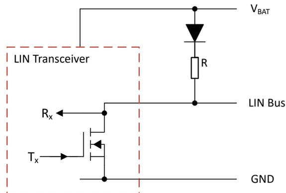
Figure 1. LIN Drive Schematic
