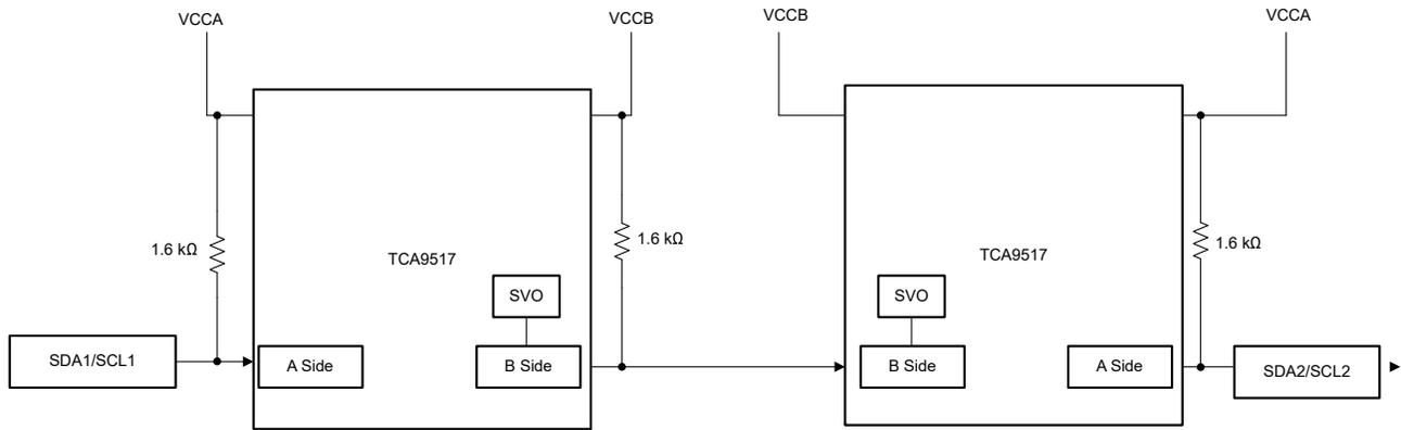
Figure 2-1. Schematic of Improper Implementation of Two TCA9517s
