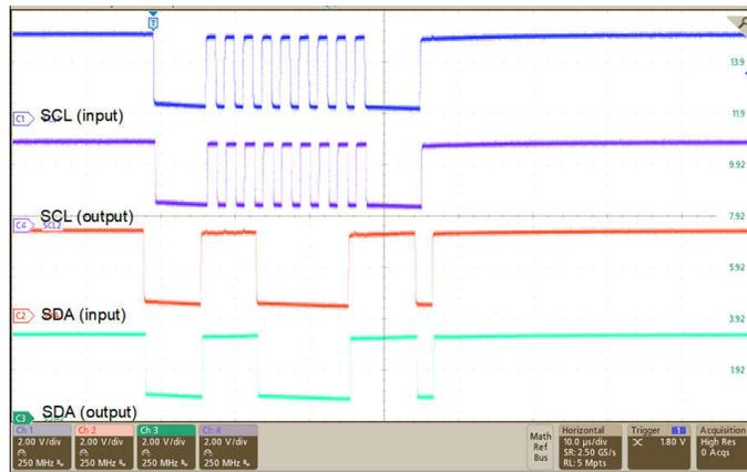
Figure 2-4. Waveforms as a Result of Proper Setup (Address 0x70h Sent)
