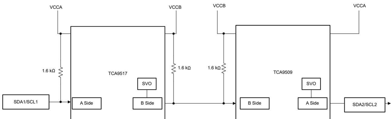
Figure 2-3. Schematic of Proper Implementation of Buffers With SVO
