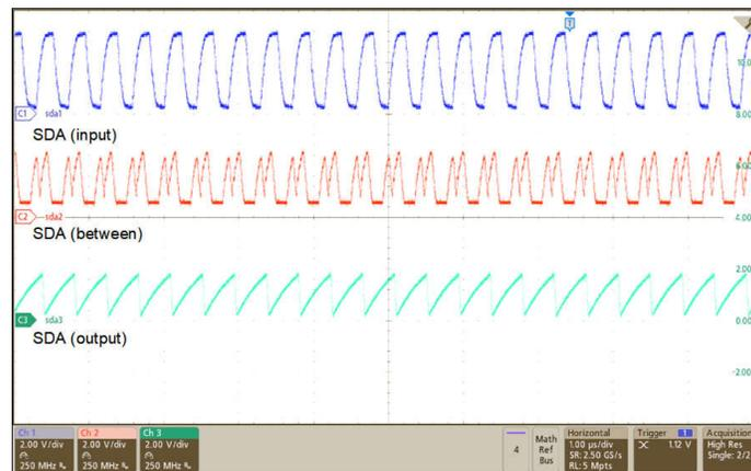
Figure 2-2. Waveforms as a Result of Improper Setup (Address 0x70h Sent)
