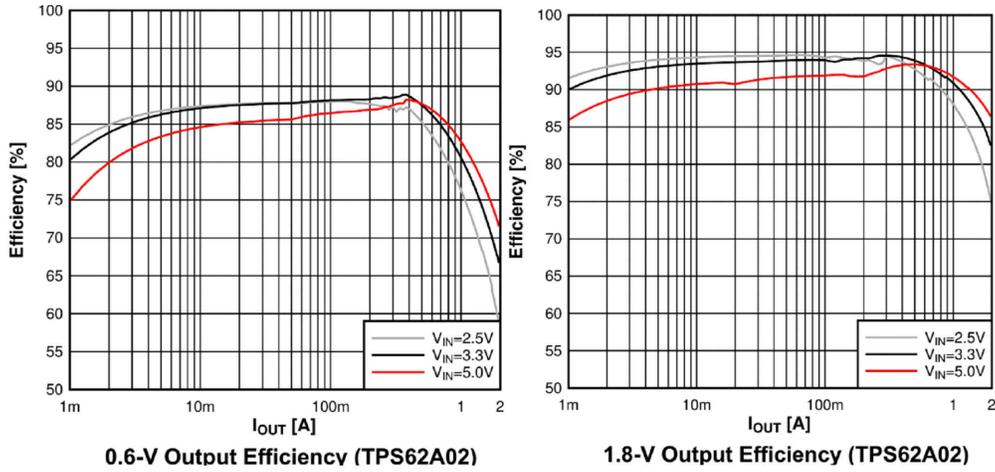
Figure 4-4. TPS62A02 Efficiency
