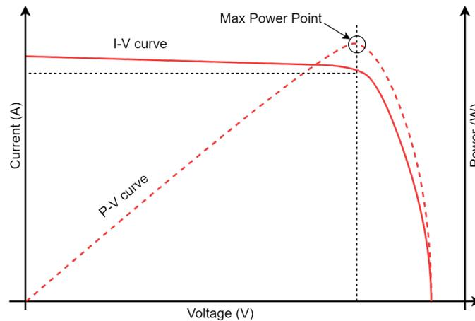
**Figure 3-4. Solar Cell PV/IV Curve**
