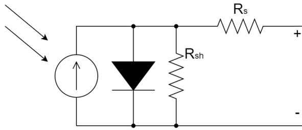
**Figure 3-3. Solar Cell Equivalent Circuit**
