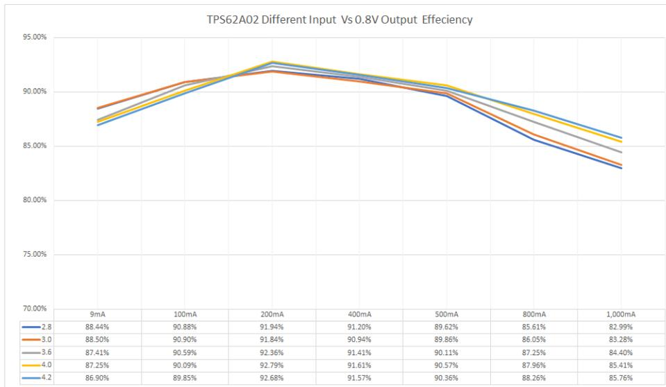
Figure 4-5. TPS62A02 Output 0.8 V Efficiency
