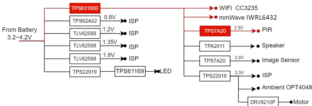
Figure 4-1. Battery Powered Camera Power Tree
