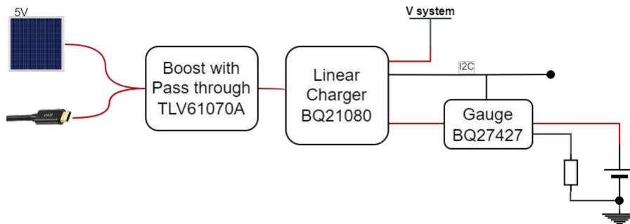
Figure 3-7. Solar Charger Design Function Block
