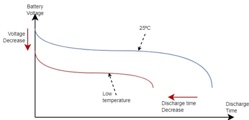
Figure 4-2. Battery Output Voltage and Discharge Time vs Temperature
