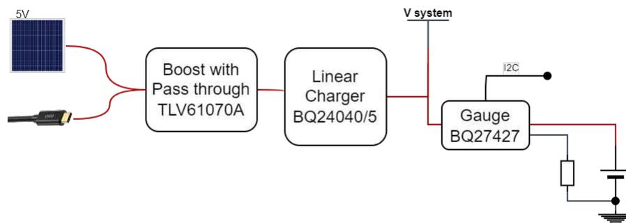
**Figure 3-5. Solar Charger Design Function Block**
