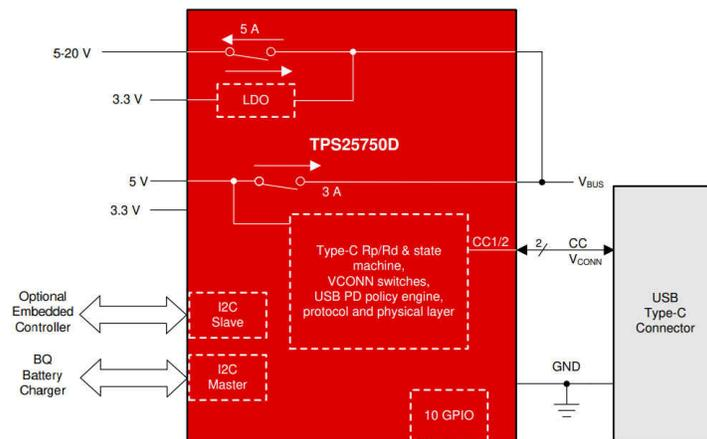
**Figure 3-2. TPS25750D Function Block**
