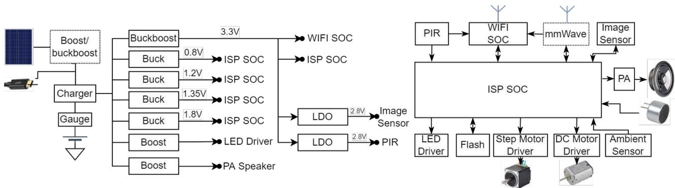
**Figure 2-1. Function Block of Battery Powered Camera**
