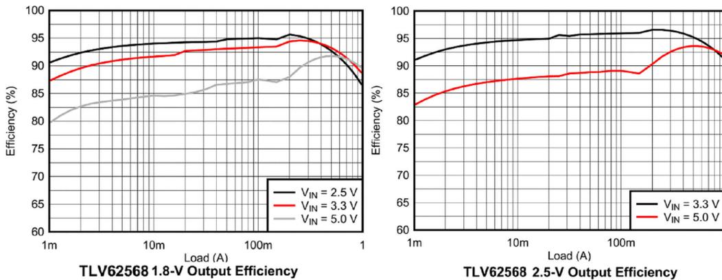
Figure 4-6. TLV62568 Efficiency
