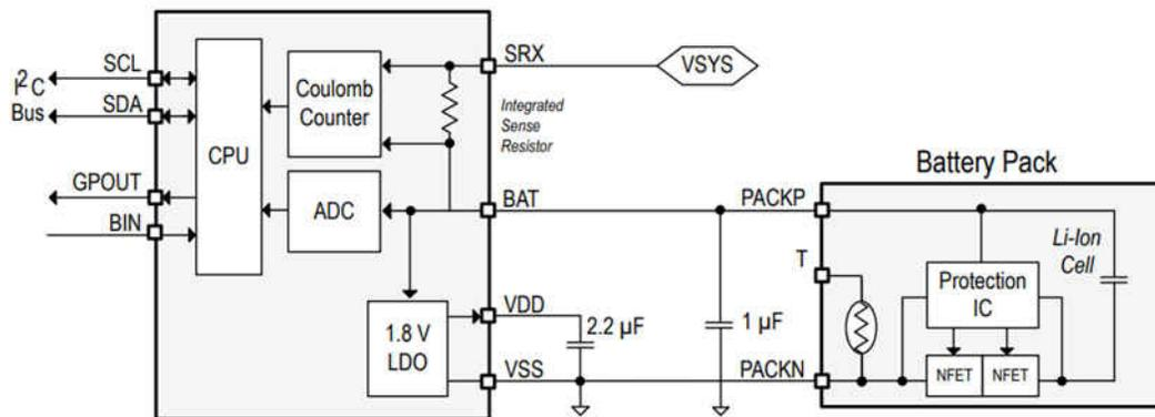
Figure 3-9. BQ27427 Gauge Function Block
