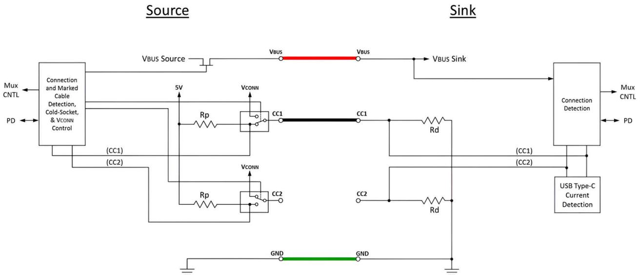
**Figure 3-1. USB Type-C Connection Between Source and Sink**
