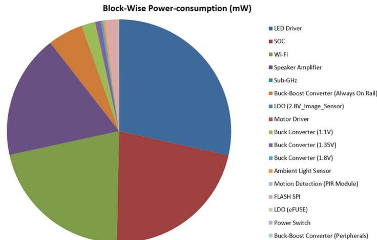
**Figure 4-7. An Example of Battery Powered Camera Energy Consumption Pie Chart**
