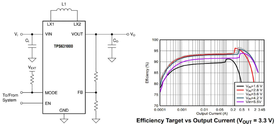
**Figure 4-3. TPS631000 Efficiency**
