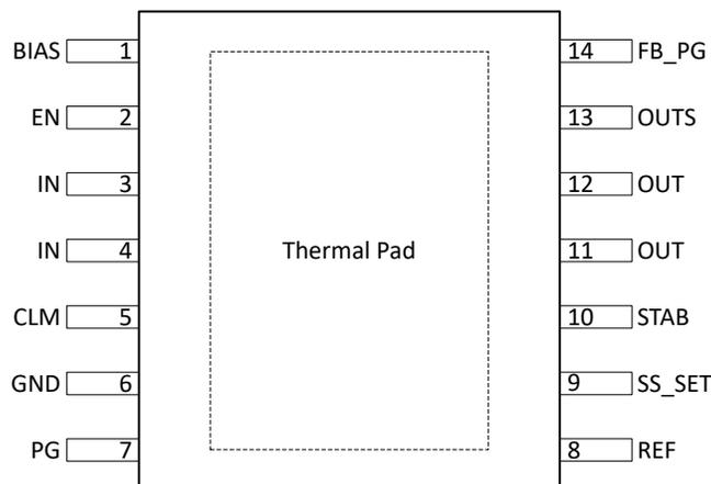
Figure 1. Pin Diagram (CFP) Package
