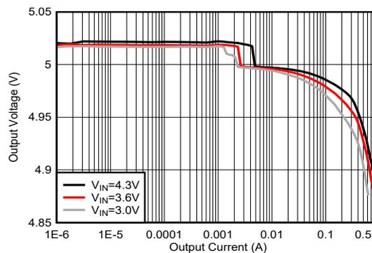
Figure 4-4. TPS61299 Load Regulation ,  $V_{out} = 5\text{ V}$
