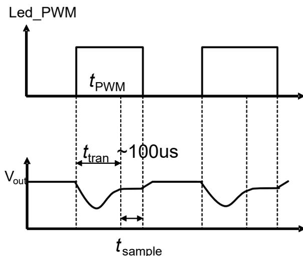
Figure 1-1. Typical Transient Response
