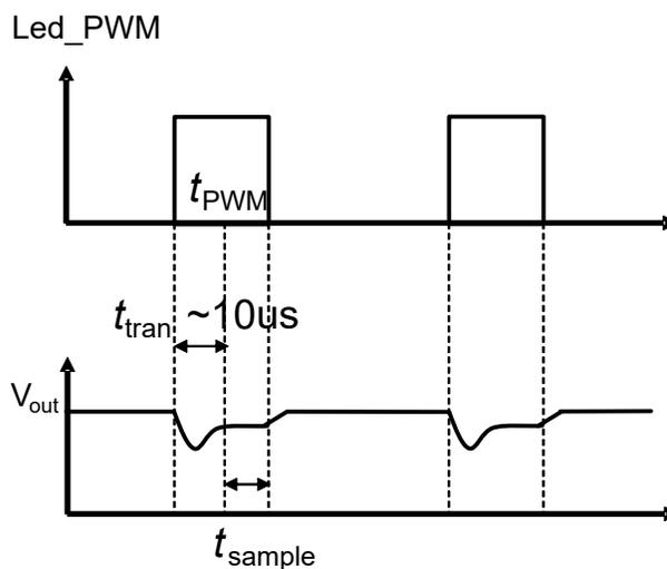
Figure 1-2. Fast Transient Response
