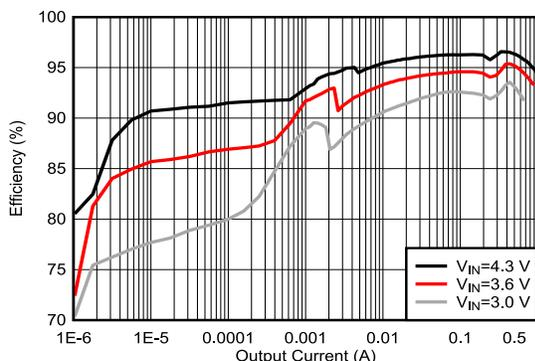
Figure 4-3. TPS61299 Efficiency ,  $V_{out} = 5\text{ V}$
