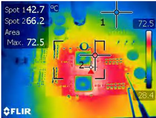
Figure 4-11. Thermal Condition in Boost Region ( $V_{IN}=8\text{ V}$  and 8 A Load)
