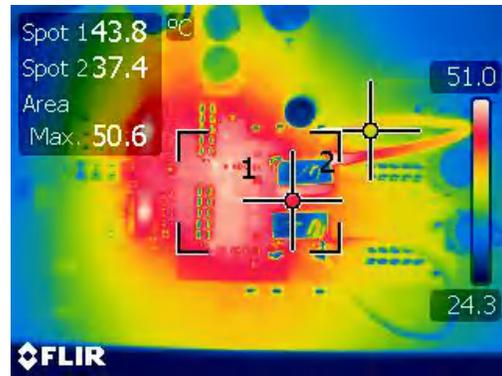
Figure 4-34. Thermal Condition in Dual Phase Buck ( $V_{IN}=24\text{ V}$  and 9 A Load)
