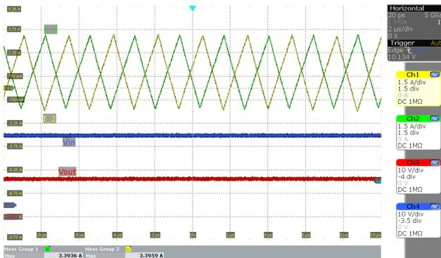
**Figure 4-9. Inductor Current in Buck Region ( $V_{IN}=30\text{ V}$  and 2 A Load)**
