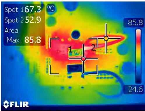
Figure 4-29. Thermal Condition in Single Phase Buck-Boost ( $V_{IN}=16\text{ V}$  and 9 A Load)
