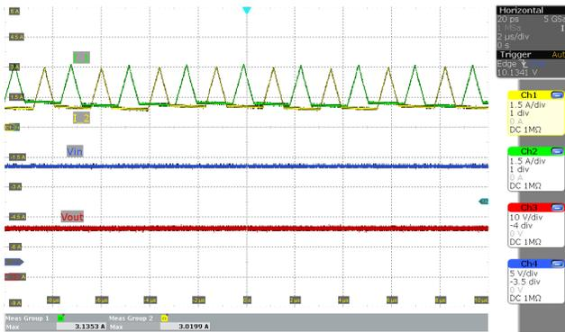
**Figure 4-7. Inductor Current in Buck-Boost Region ( $V_{IN}=16\text{ V}$  and 2 A Load)**
