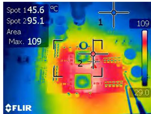
Figure 4-14. Thermal Condition in Boost Region ( $V_{IN}=10\text{ V}$  and 14 A Load)
