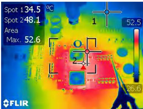
Figure 4-13. Thermal Condition in Boost Region ( $V_{IN}=10\text{ V}$  and 8 A Load)
