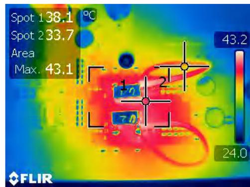
**Figure 4-20. Thermal Condition in Dual Phase Boost ( $V_{IN}=8$  V and 4 A Load)**
