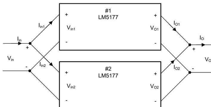
**Figure 2-1. Two Parallel LM5177 Converters as Power Supply**
