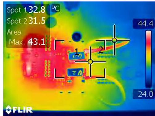
Figure 4-32. Thermal Condition in Dual Phase Buck ( $V_{IN}=24\text{ V}$  and 4 A Load)
