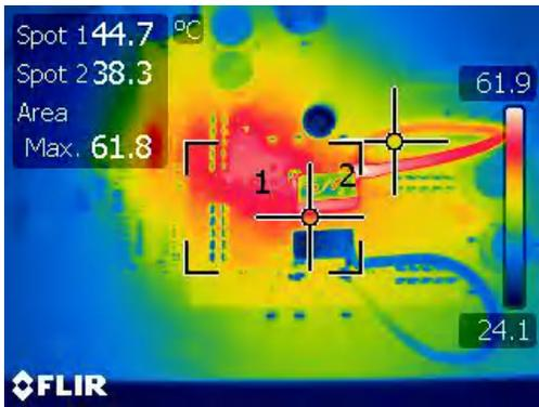
Figure 4-33. Thermal Condition in Single Phase Buck ( $V_{IN}=24\text{ V}$  and 9 A Load)
