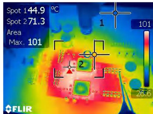
Figure 4-16. Thermal Condition in Buck-Boost Region ( $V_{IN}=16\text{ V}$  and 18 A Load)
