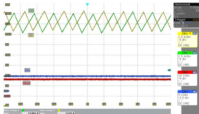
Figure 4-4. Inductor Current in Boost Region ( $V_{IN} = 8\text{ V}$  and 10 A Load)
