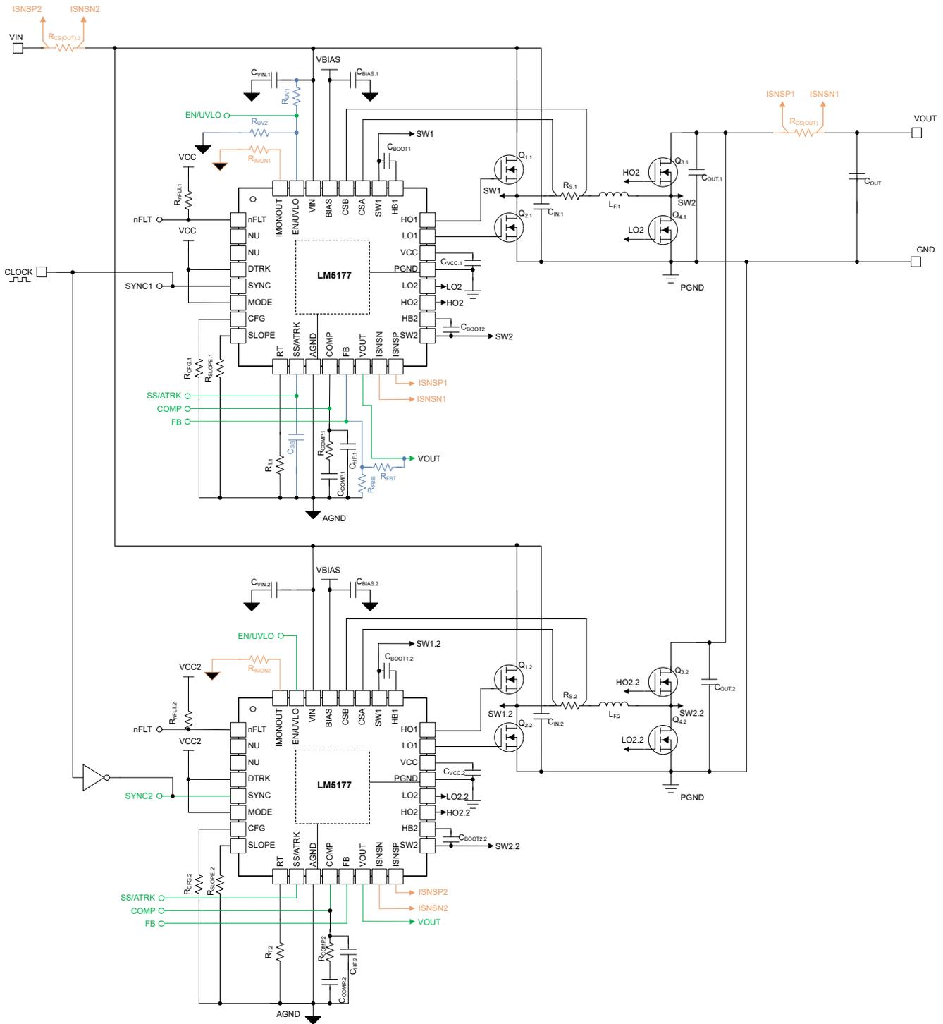
Figure 3-1. Block Diagram of Two LM5177 in Parallel Operation
