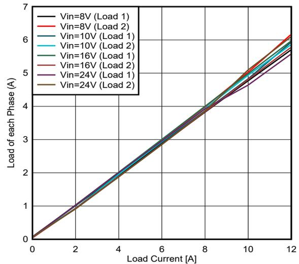
Figure 4-2. Load Distribution of Two Phases
