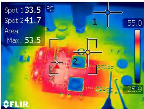
Figure 4-15. Thermal Condition in Buck-Boost Region ( $V_{IN}=16\text{ V}$  and 8 A Load)
