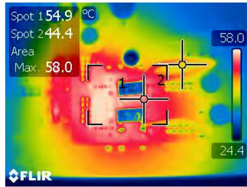
Figure 4-30. Thermal Condition in Dual Phase Buck-Boost ( $V_{IN}=16\text{ V}$  and 9 A Load)
