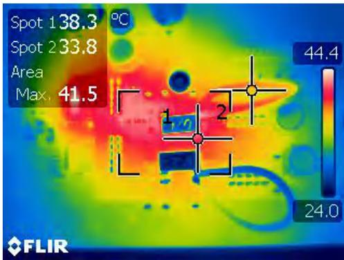
Figure 4-27. Thermal Condition in Single Phase Buck-Boost ( $V_{IN}=16\text{ V}$  and 4 A Load)
