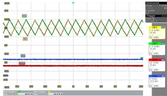
**Figure 4-6. Inductor Current in Boost Region ( $V_{IN}=10\text{ V}$  and 10 A Load)**
