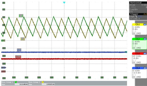
**Figure 4-5. Inductor Current in Boost Region ( $V_{IN}=10\text{ V}$  and 2 A Load)**
