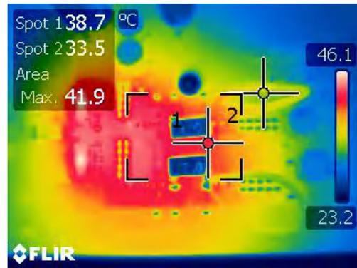
Figure 4-28. Thermal Condition in Dual Phase Buck-Boost ( $V_{IN}=16\text{ V}$  and 4 A Load)
