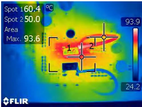
Figure 4-25. Thermal Condition in Single Phase Boost ( $V_{IN}=10\text{ V}$  and 7 A Load)
