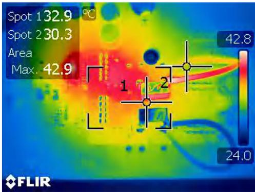
Figure 4-31. Thermal Condition in Single Phase Buck ( $V_{IN}=24\text{ V}$  and 4 A Load)
