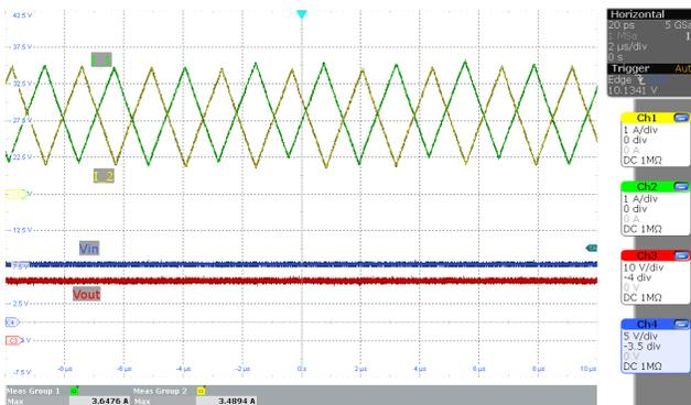
Figure 4-3. Inductor Current in Boost Region ( $V_{IN} = 8\text{ V}$  and 2 A Load)
