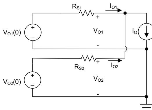
**Figure 2-2. Equivalent Model**
