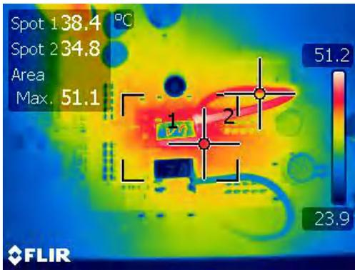
Figure 4-23. Thermal Condition in Single Phase Boost ( $V_{IN}=10\text{ V}$  and 4 A Load)
