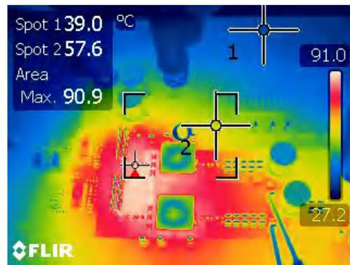
**Figure 4-18. Thermal Condition in Buck Region ( $V_{IN}=24$  V and 18 A Load)**
