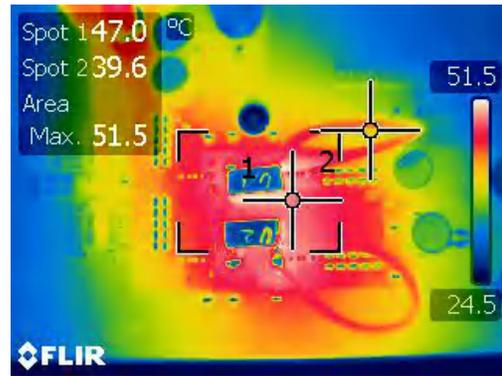
Figure 4-26. Thermal Condition in Dual Phase Boost ( $V_{IN}=10\text{ V}$  and 7 A Load)
