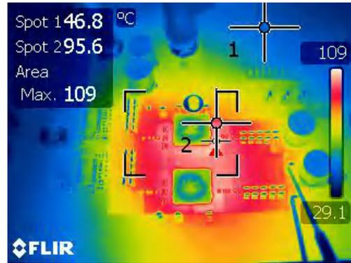
Figure 4-12. Thermal Condition in Boost Region ( $V_{IN}=8\text{ V}$  and 12 A Load)
