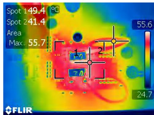
**Figure 4-22. Thermal Condition in Dual Phase Boost ( $V_{IN}=8$  V and 6 A Load)**
