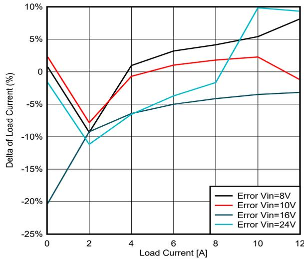
Figure 4-1. Error of Load Currents
