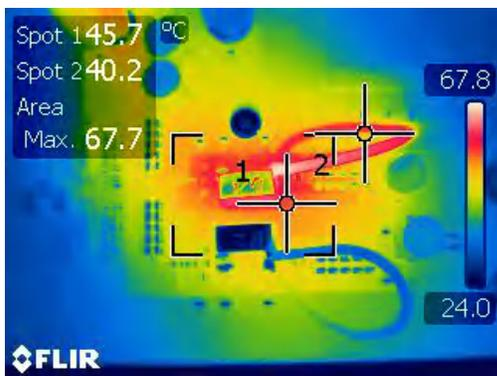
**Figure 4-19. Thermal Condition in Single Phase Boost ( $V_{IN}=8$  V and 4 A Load)**
