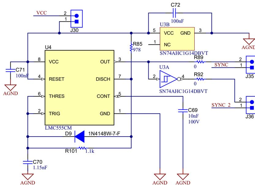
Figure 2-3. 2-Phase Clock Generator
