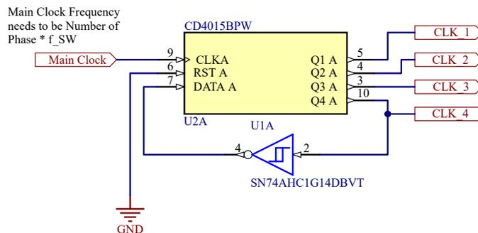
Figure 2-4. Multiphase Clock Generator
