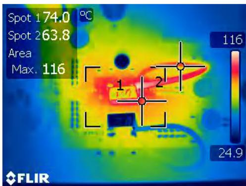
**Figure 4-21. Thermal Condition in Single Phase Boost ( $V_{IN}=8$  V and 6 A Load)**
