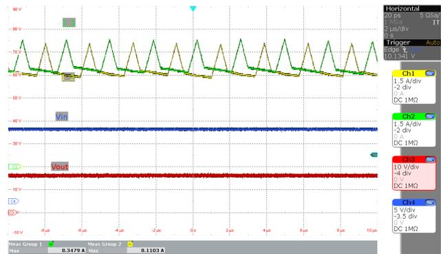
**Figure 4-8. Inductor Current in Buck-Boost Region ( $V_{IN}=16\text{ V}$  and 10 A Load)**
