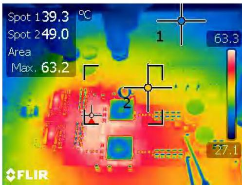
**Figure 4-17. Thermal Condition in Buck Region ( $V_{IN}=24$  V and 8 A Load)**
