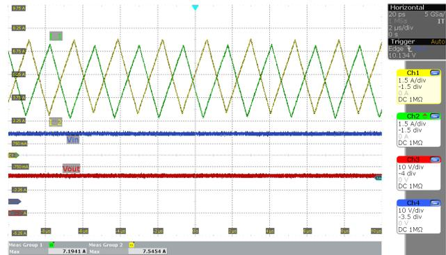
**Figure 4-10. Inductor Current in Buck Region ( $V_{IN}=30\text{ V}$  and 10 A Load)**
