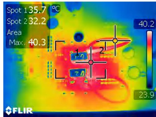
Figure 4-24. Thermal Condition in Dual Phase Boost ( $V_{IN}=10\text{ V}$  and 4 A Load)
