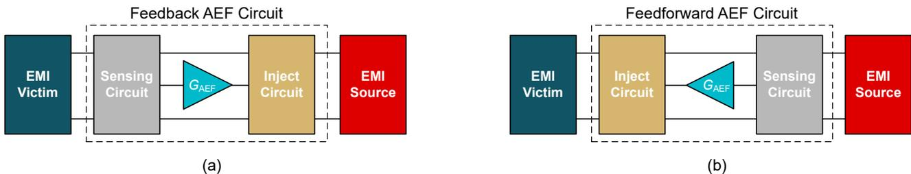
**Figure 4-1. Fundamental Concept of AEF With Sensing, Gain and Injection Stages. The Control Structure can be FB (a) or FF (b)**
