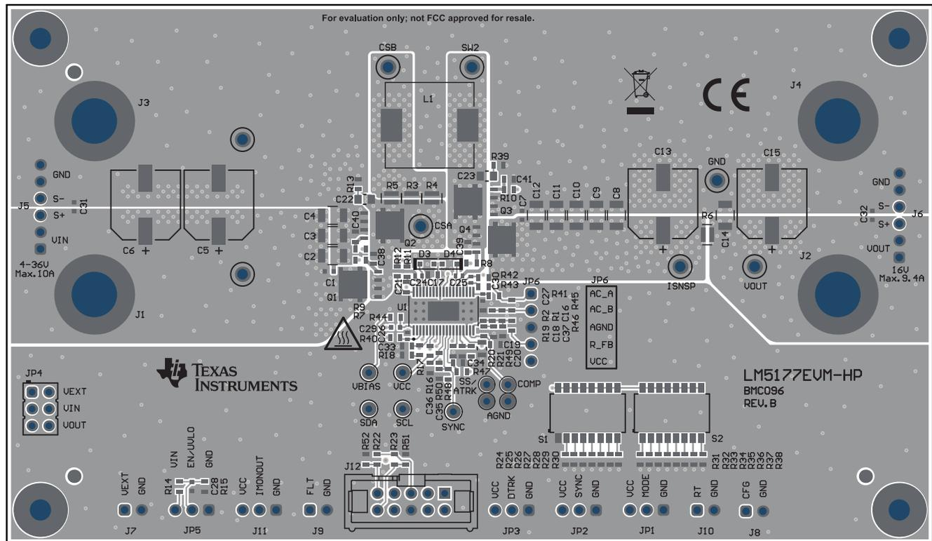
Figure 4-1. LM5177 Top Layer Routing Example
