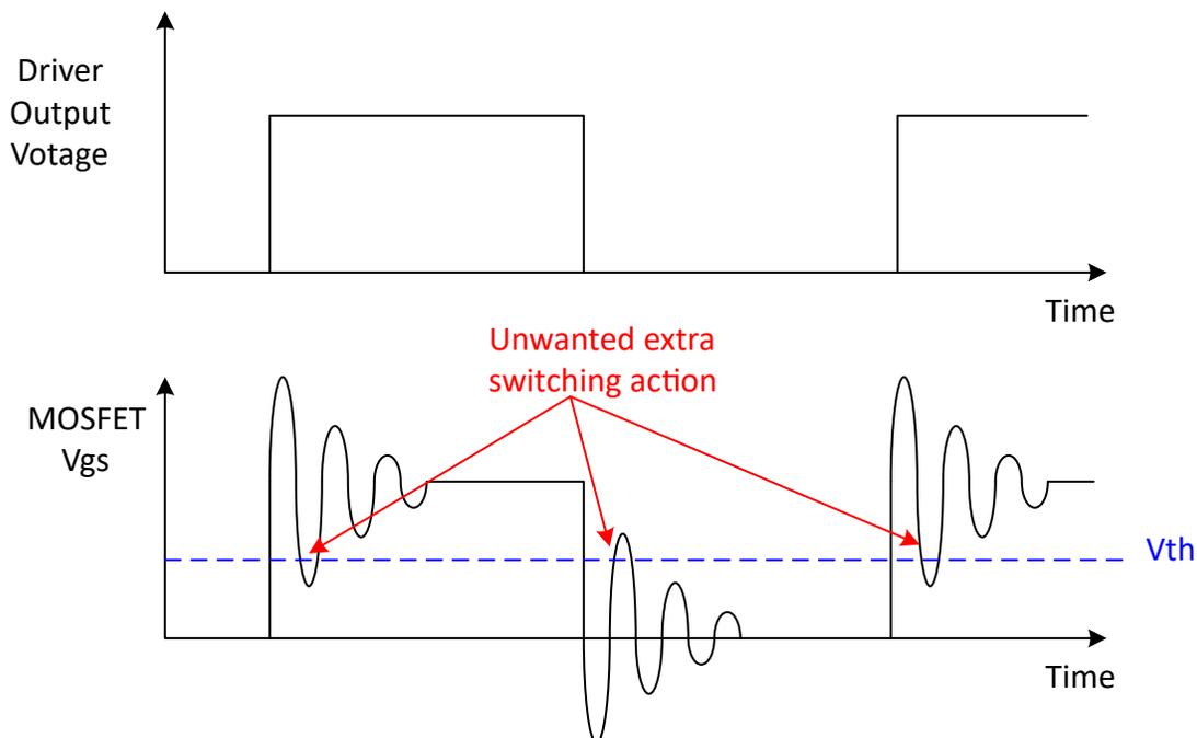
Figure 2-5. Gate Ringing and Unwanted Extra Switching Action
