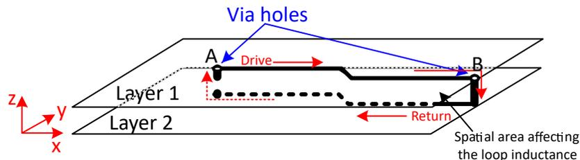
**Figure 2-7. Routing the Return Trace in the Shadow of the Drive Trace on an Adjacent Layer to Minimize Loop Inductance**
