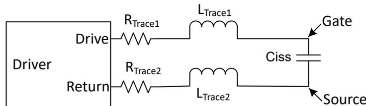
Figure 2-4. Gate – Drive Equivalent Circuit
