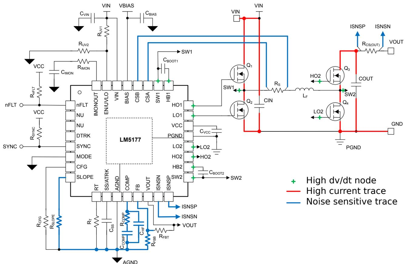
**Figure 2-1. Identifying High  $di/dt$  Loops, High  $dv/dt$  Nodes and Sensitive Traces**
