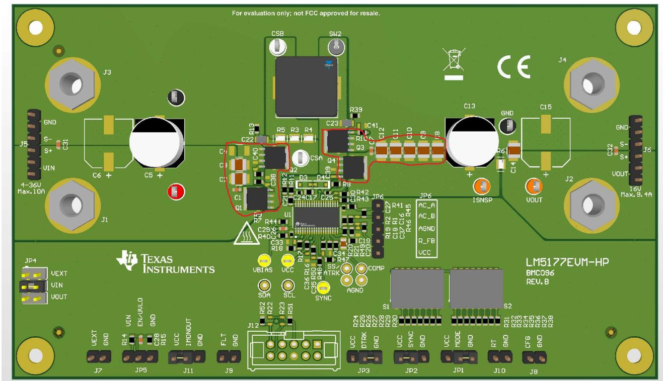
Figure 2-2. Hot Loops in a LM5177 Four Switch Buck - Boost Device
