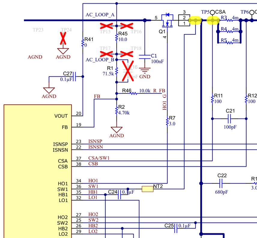
Figure 2-3. Example of Using the Net-Tie to Treat CSA and SW1 as Separate Nodes
