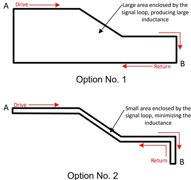
**Figure 2-6. Routing patterns for current loop traces between point A and B on the PCB**
