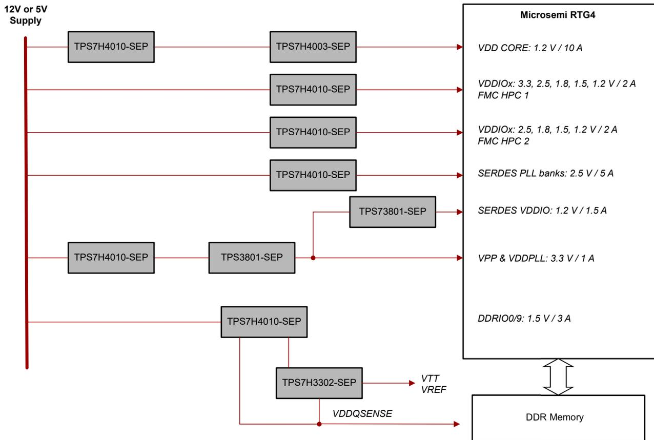
Figure 4-2. Rad-Tolerant Power for RTG4
