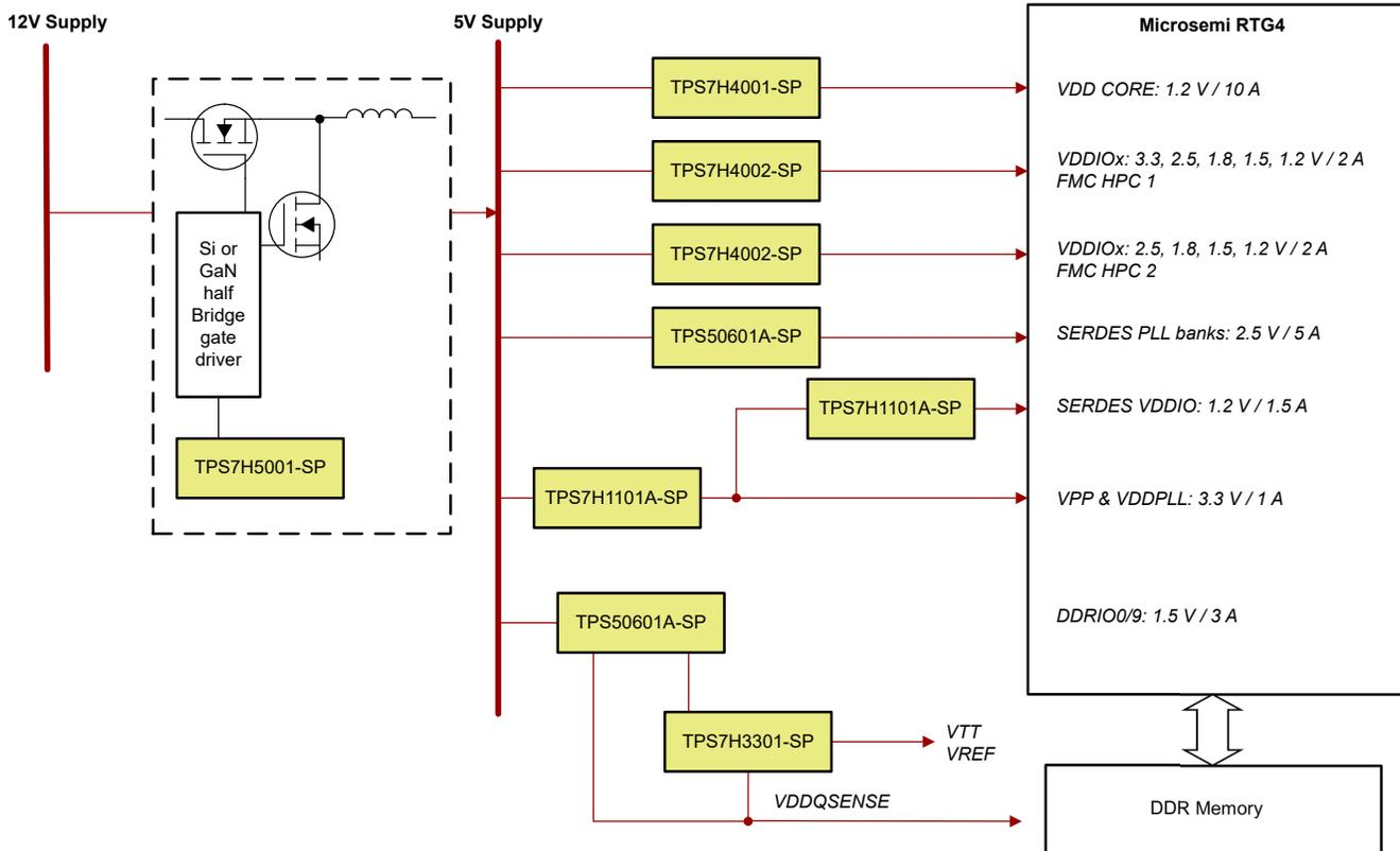
Figure 4-1. Rad-Hard Power for RTG4
