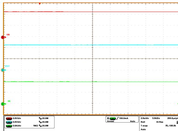
**Figure 7. TPS25981 Running Continuously at 10 A, 70 C**
