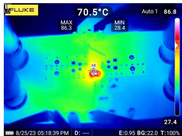
**Figure 5. Competition Device EVM, VIN=12 V, IOU=10 A**
