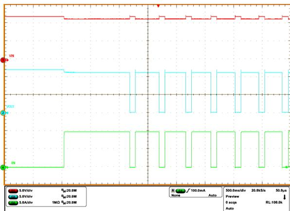
**Figure 6. Competition Device Shutting Down at 10 A, 70 C**
