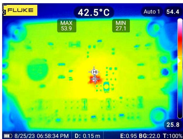
**Figure 4. TPS25981EVM, VIN=12 V, IOU=10 A**
