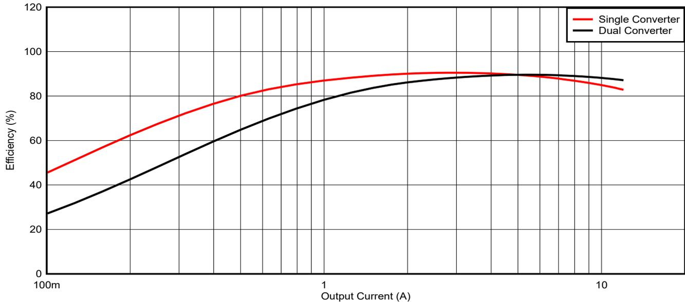
**Figure 3-1. Efficiency of the Single Converter and Dual Converter**
