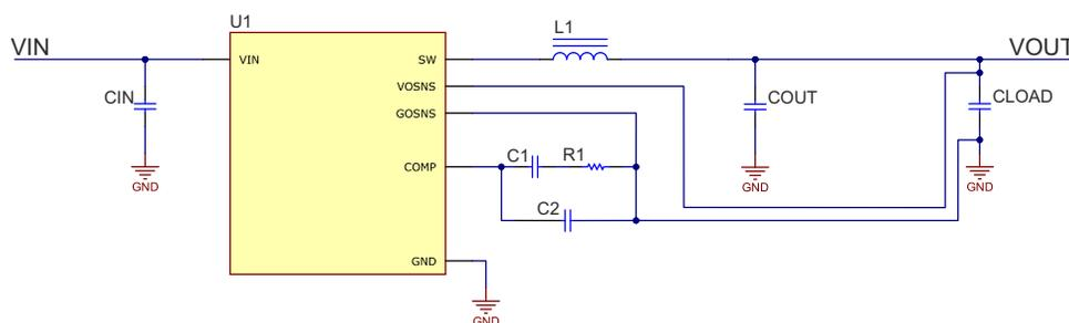
**Figure 2-1. Single Converter Schematic**
