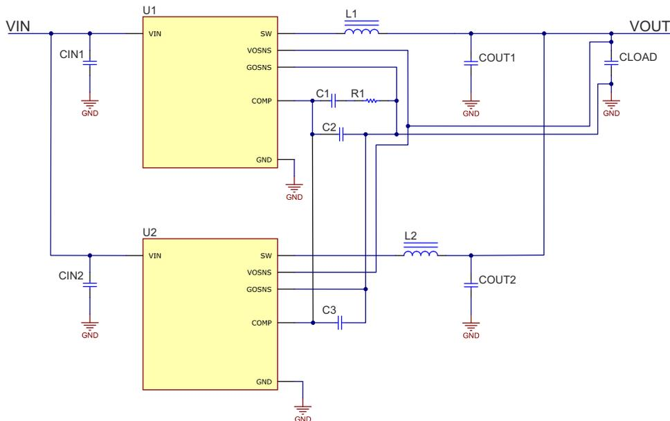
**Figure 2-2. Dual Converter Schematic**
