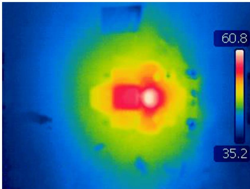
**Figure 3-5. Heat Distribution of Single Converter**
