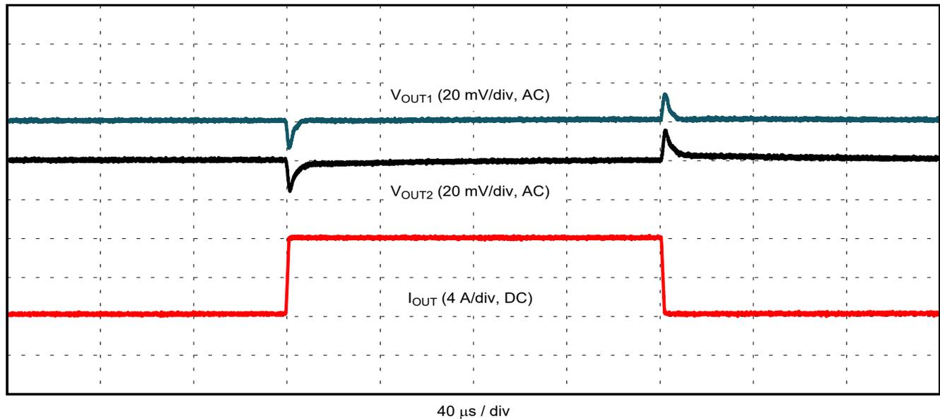
Figure 3-4. Load Transient of the Single Converter and Dual Converter
