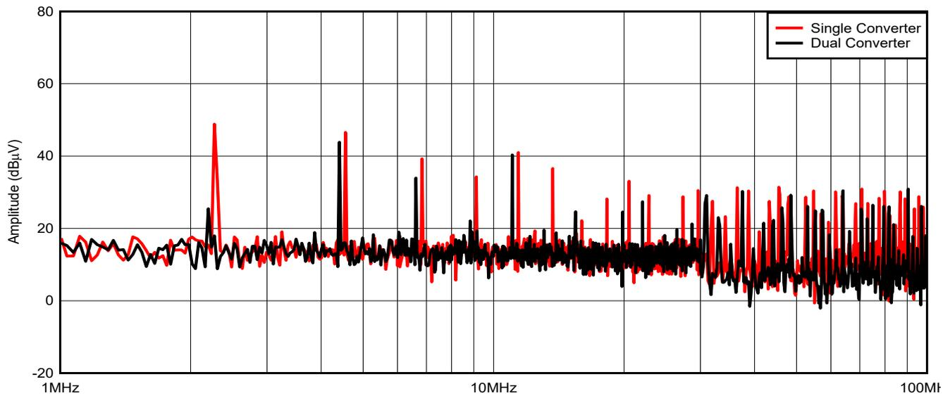
**Figure 3-2. Input Voltage Ripple of the Single Converter and Dual Converter**
