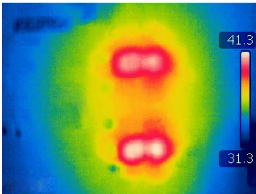
**Figure 3-6. Heat Distribution of Dual Converter**
