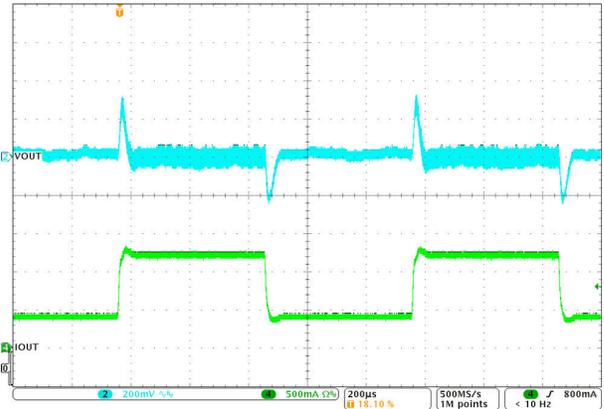
Figure 4-3. Load Transient 0.4 A to 1.2 A With 12 V<sub>IN</sub>
