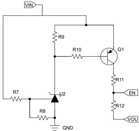
**Figure 3-2. Enabling and Adjusting UVLO Circuit**
