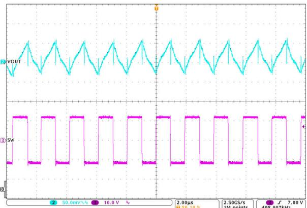
Figure 4-5. V<sub>OUT</sub> Ripple at 1.2 A
