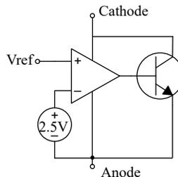
**Figure 3-3. Simplified Block Diagram of the Regulator**
