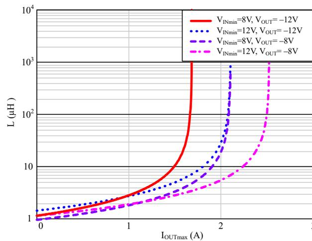
**Figure 2-1. Output Current Range Versus Inductor L**
