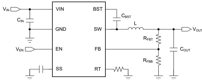
**Figure 1-1. Buck Converter Application**
