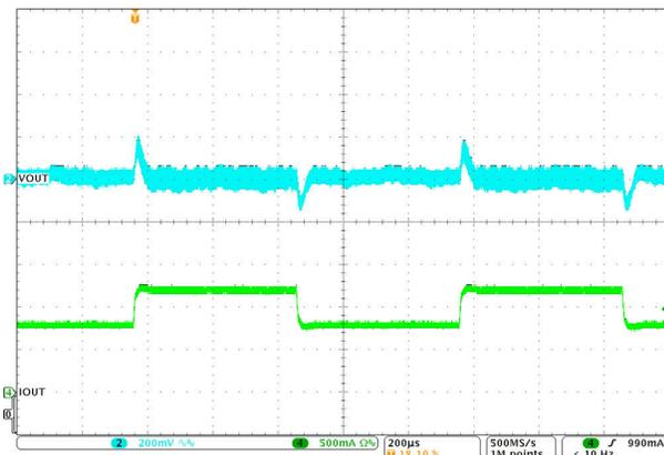
Figure 4-4. Load Transient 0.8 A to 1.2 A With 12 V<sub>IN</sub>
