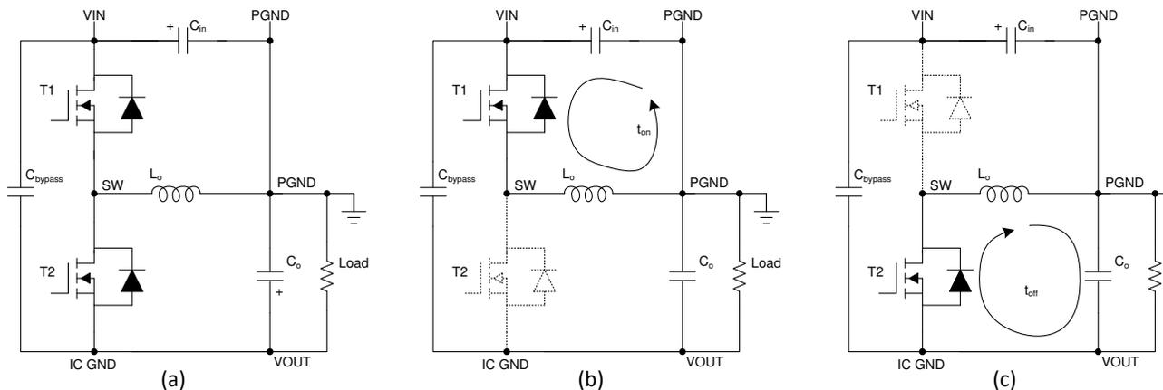
**Figure 1-3. Inverting Buck Boost Configuration**
