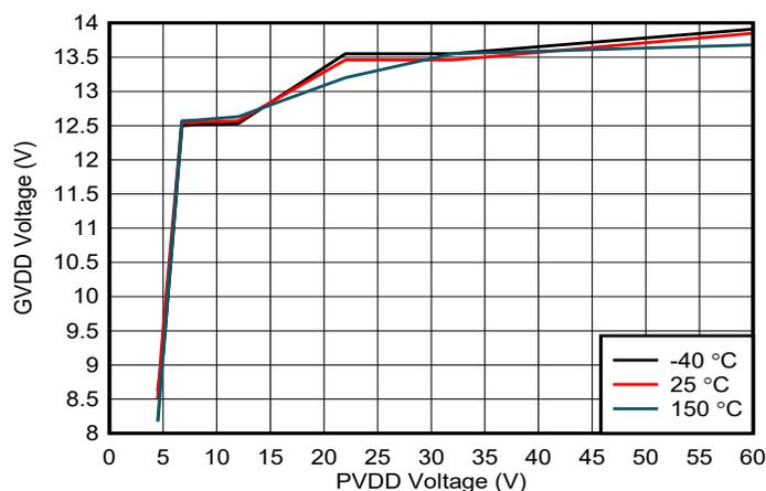
**Figure 2-4. DRV8329 GVDD Voltage Over PVDD Voltage**
