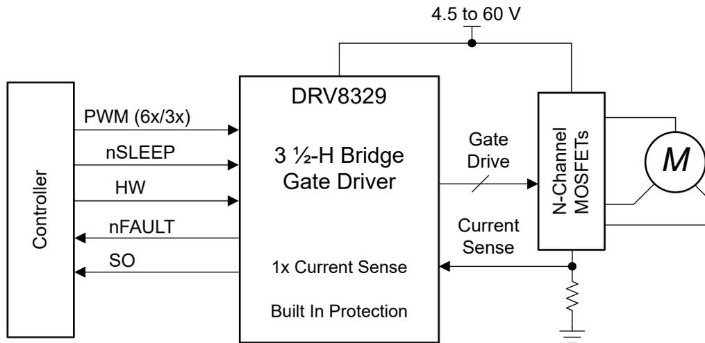
Figure 1-1. Simplified Schematic for DRV8329
