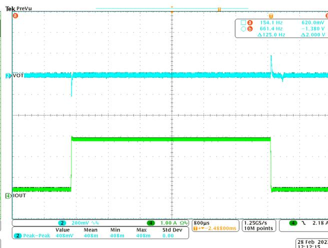
**Figure 2-2. Part1 PCM Transient Response 0.3A-2.7 A**
