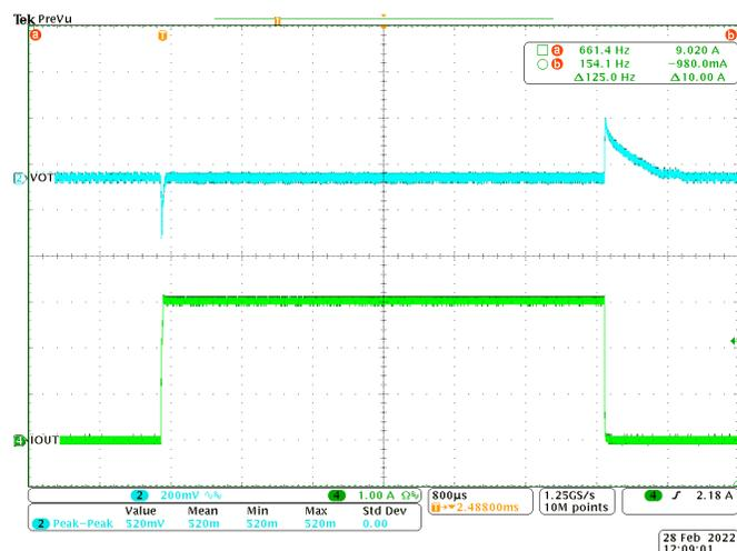
**Figure 2-1. Part1 PCM Transient Response 0A-3 A**
