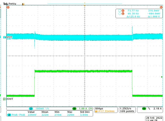
Figure 2-8. TPS563211 AECM Transient Response 0.3A-2.7A
