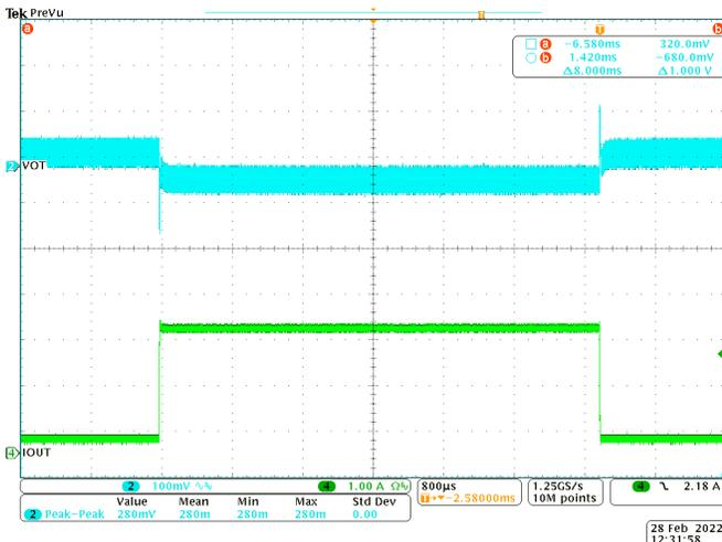
Figure 2-5. Part2 DCAP2 Transient Response 0.3A-2.7A
