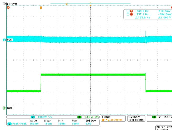
Figure 2-9. TPS563211 AECM Transient Response 1.5A-3A
