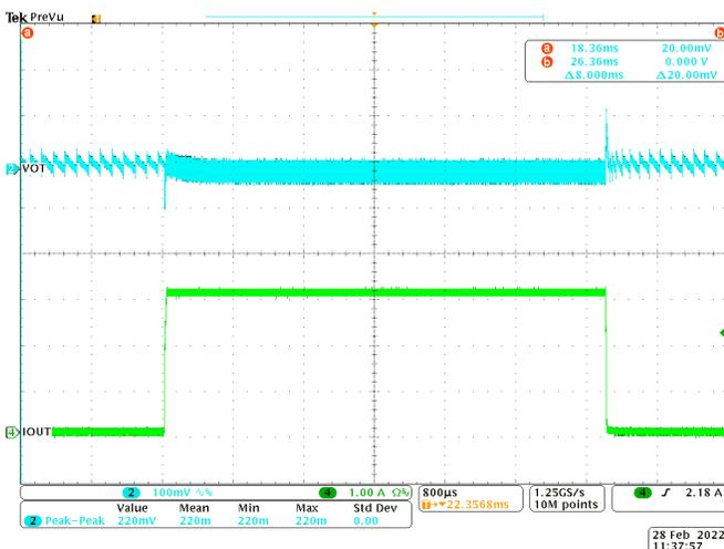
Figure 2-7. TPS563211 AECM Transient Response 0A-3A
