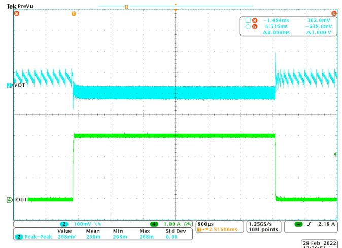
Figure 2-4. Part2 DCAP2 Transient Response 0A-3A
