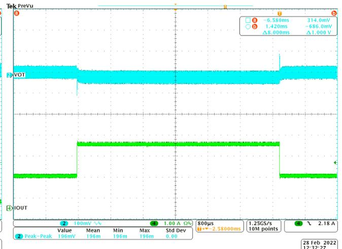
Figure 2-6. Part2 DCAP2 Transient Response 1.5A-3A
