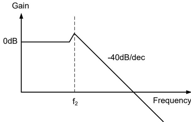
**Figure 2-2. Loop Gain Magnitude Plot of Equation (2)**
