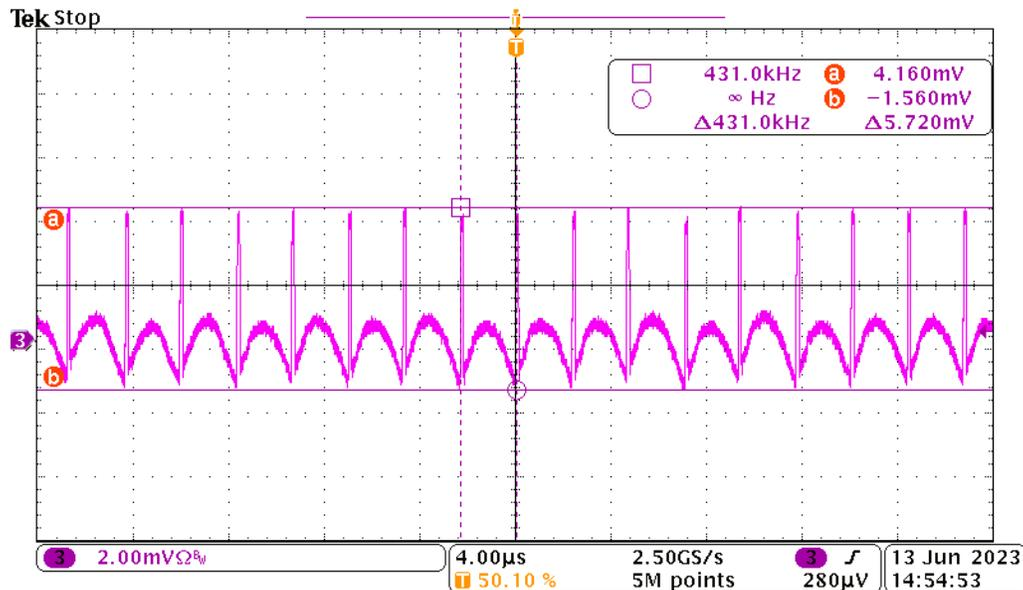
**Figure 3-1. Output Voltage Ripple Without Second Stage Filter**
