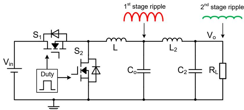
Figure 2-1. Buck Converter with Second Stage Filter
