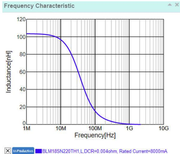
**Figure 4-4. BLM18SN220TH1 Inductance VS Frequency**
