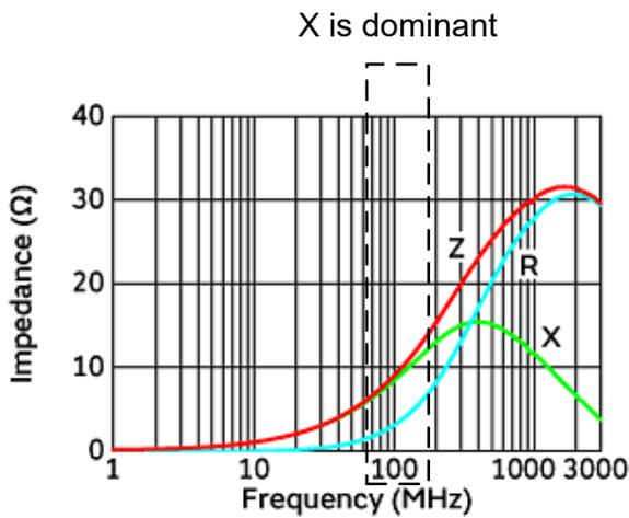
Figure 4-1. BLE18PS080SN1 Impedance VS Frequency
