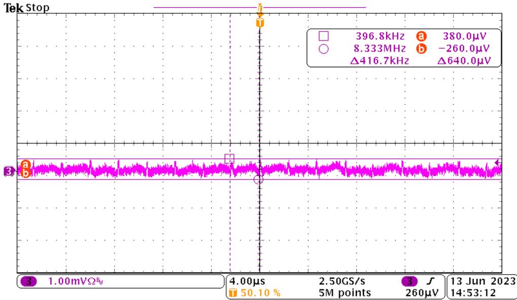
Figure 3-2. Output Voltage Ripple with Second Stage Filter
