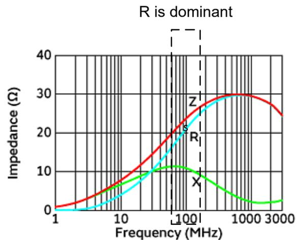
Figure 4-2. BLM18SN220TH1 Impedance VS Frequency
