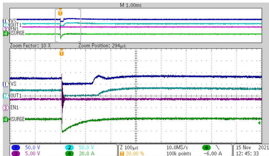
Figure 4-5. Waveform with Negative Surge Applied at VS
