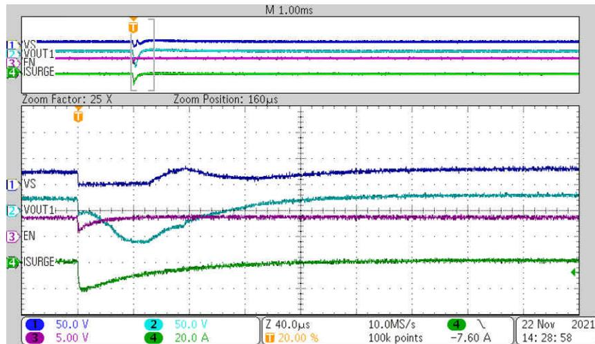
**Figure 4-7. Waveform with Negative Surge Applied at VOUT and EN is High**
