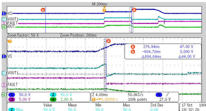
Figure 3-1. Over-Voltage Protection During ON State with Supply Ramping
