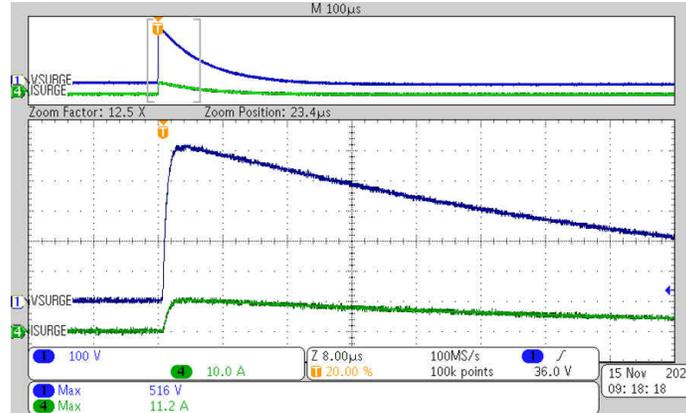
**Figure 4-1. Surge Waveform on Resistive Load**
