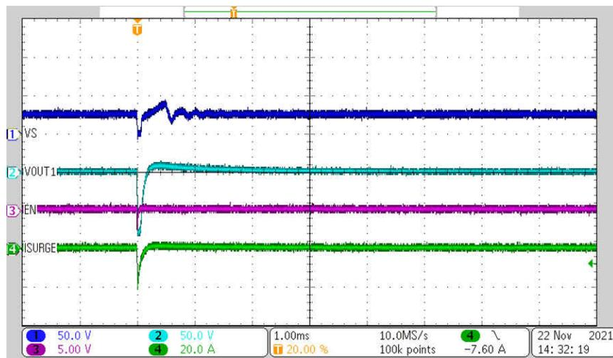
**Figure 4-9. Waveform with Negative Surge Applied at VOUT and EN is Low**
