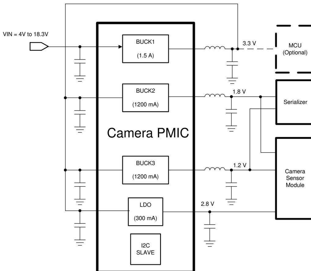
**Figure 2-1. Typical Automotive Camera Application**
