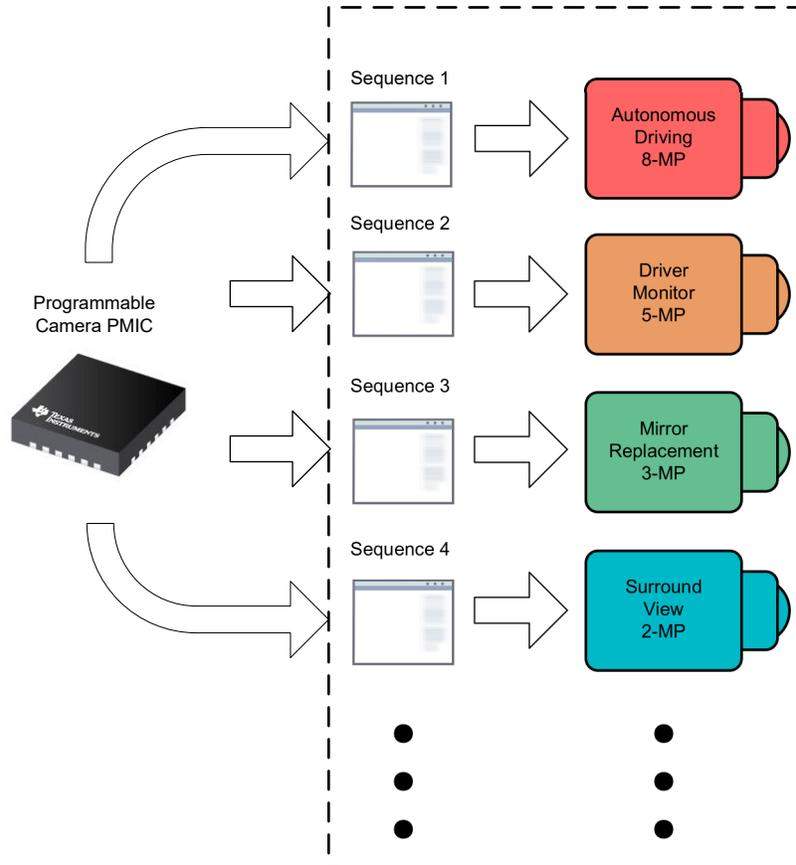
**Figure 2-2. Using One PMIC for Multiple Camera Applications**
