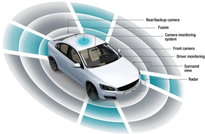
**Figure 1-1. ADAS Camera Applications**
