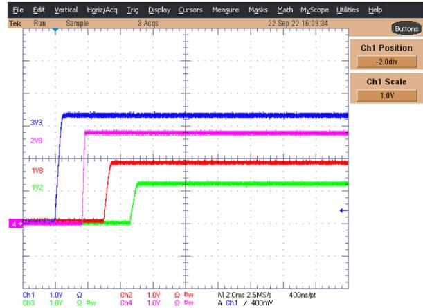
Figure 3-7. TPS65033000 Power Sequence After Reprogramming
