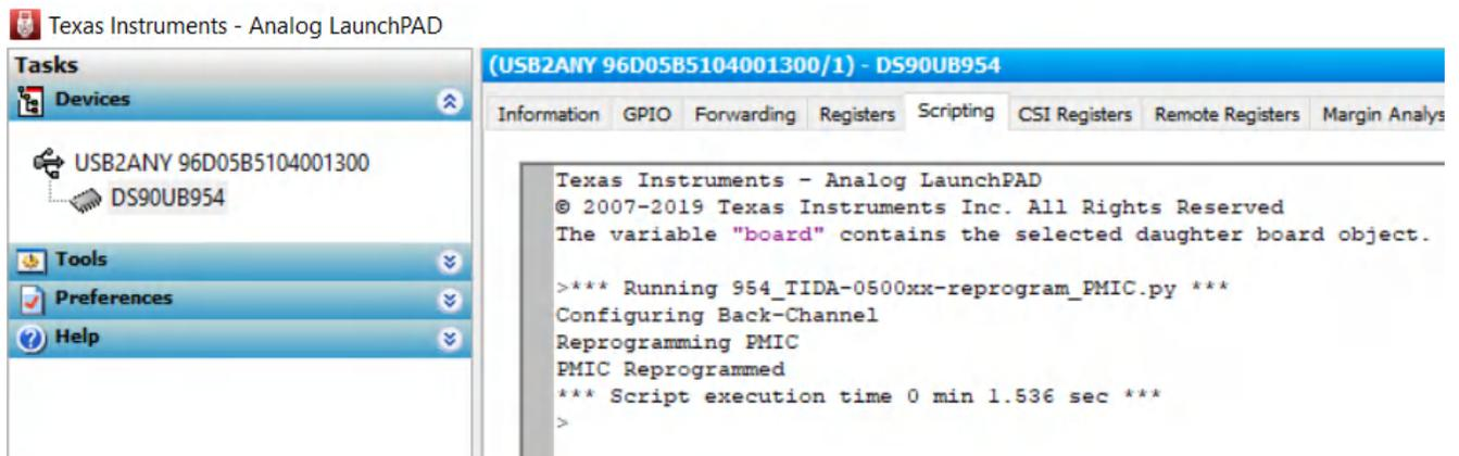
Figure 3-5. Analog LaunchPad Scripting Window
