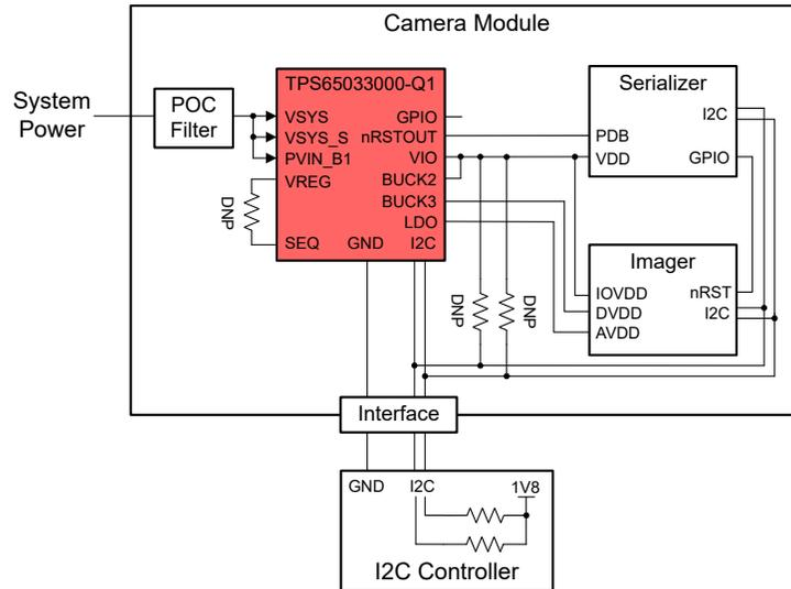
**Figure 3-2. Reprogramming the TPS65033000-Q1 with an External I2C Controller**
