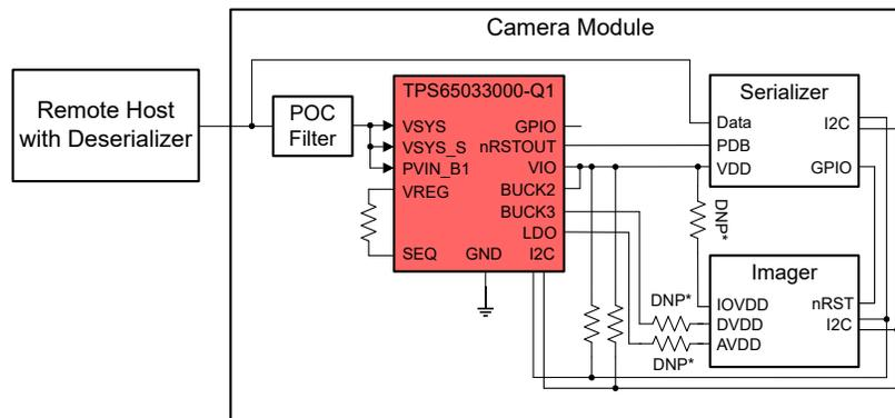
**Figure 3-3. Reprogramming the TPS65033000-Q1 with a Remote Deserializer**
