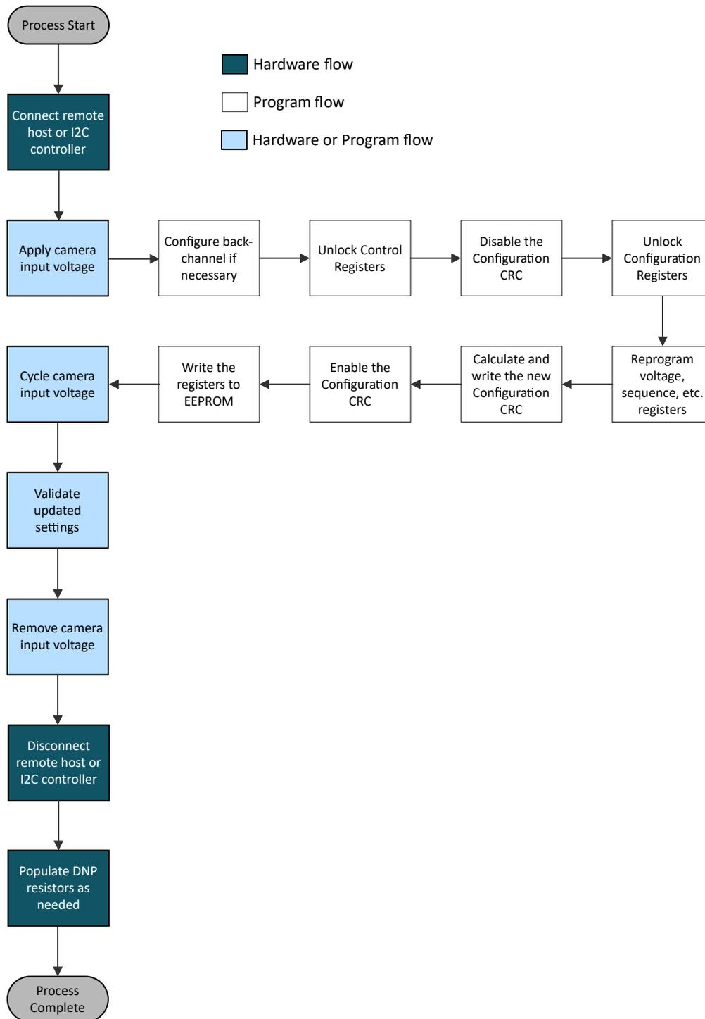
Figure 3-1. TPS6503xx-Q1 Production Programming Flow
