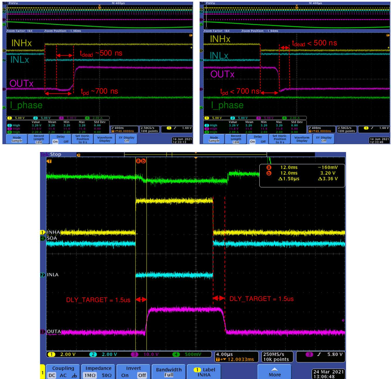
Figure 5-3. Comparison of DRV8316 Output Waveforms With and Without 1.5  $\mu$ s of Delay Compensation
