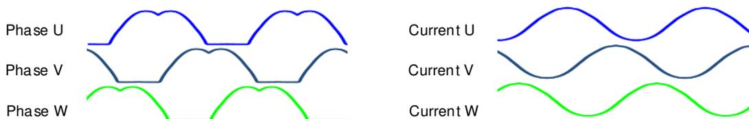
**Figure 2-1. Sinusoidal Current Control Waveforms**
