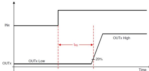
**Figure 1-1. Propagation Delay Timing in Integrated MOSFET Drivers**
