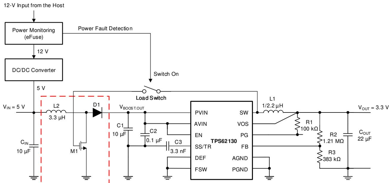
Figure 2-2. Application Example With Load Switch
