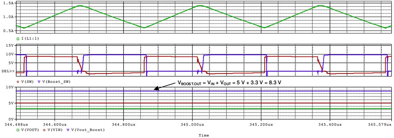
Figure 3-1. PSpice Simulation Results in Steady State
