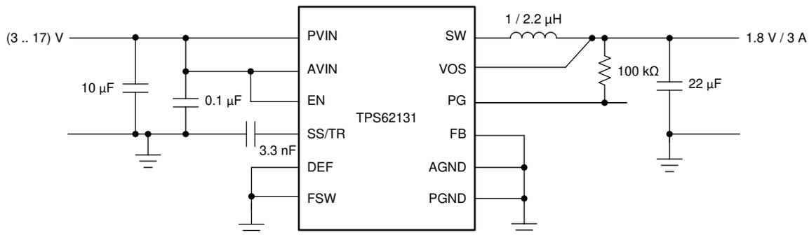
**Figure 1-1. Typical TPS62130 Application Circuit**
