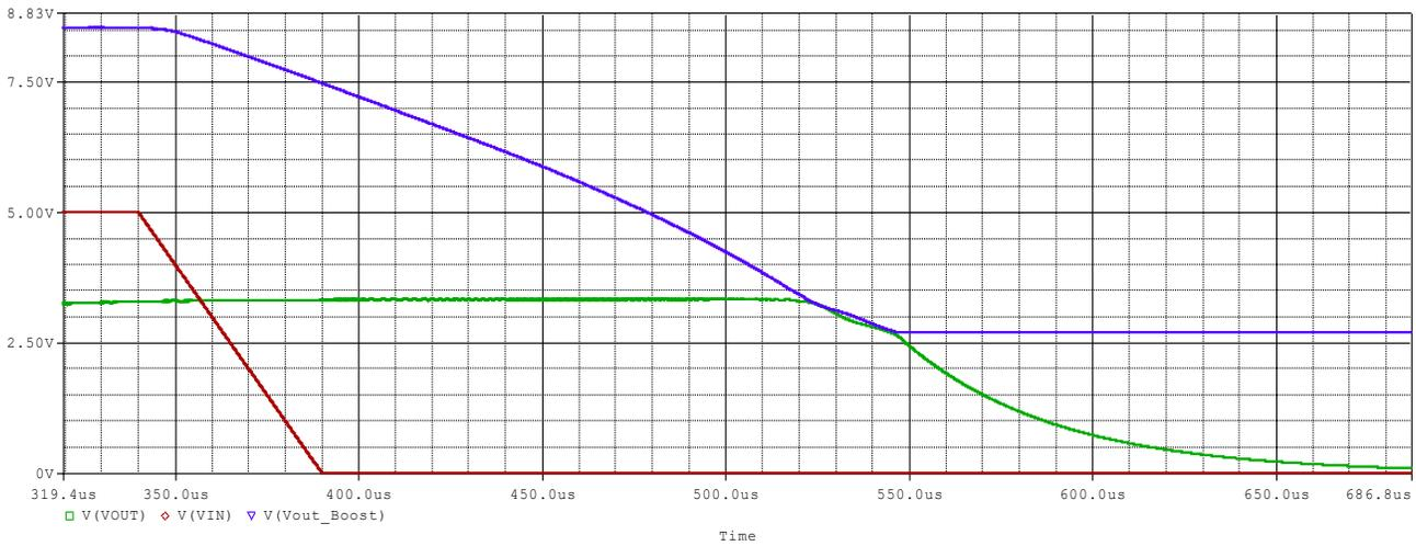
Figure 3-2. PSpice Simulation Results ( $V_{IN}$ ,  $V_{BOOST.OUT}$ ,  $V_{OUT}$ )
