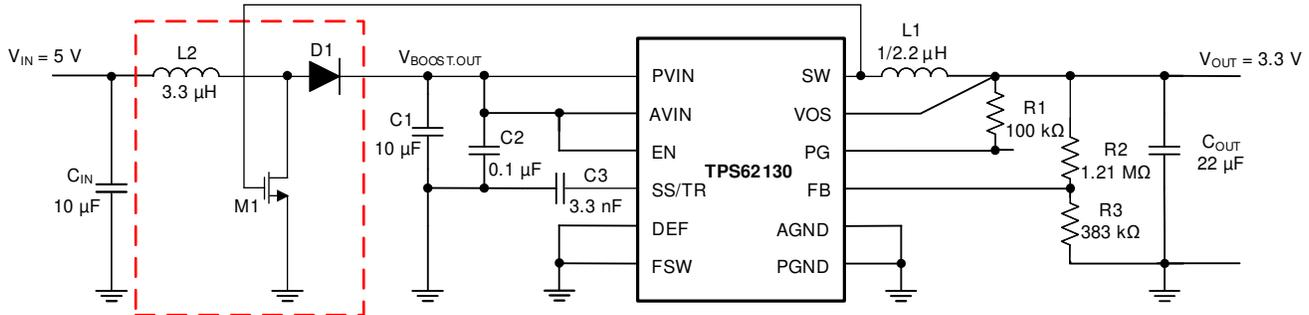
**Figure 2-1. Proposed Application Circuit Using Boost Pre-Regulator**
