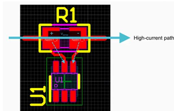
**Figure 8-1. Example of a Good Kelvin Connection**
