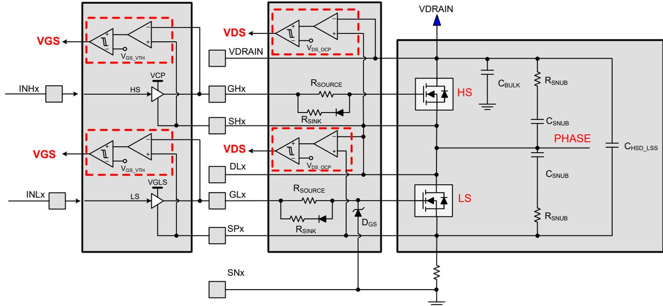
**Figure 6-1. Example Implementation of VDS and VGS Monitors**
