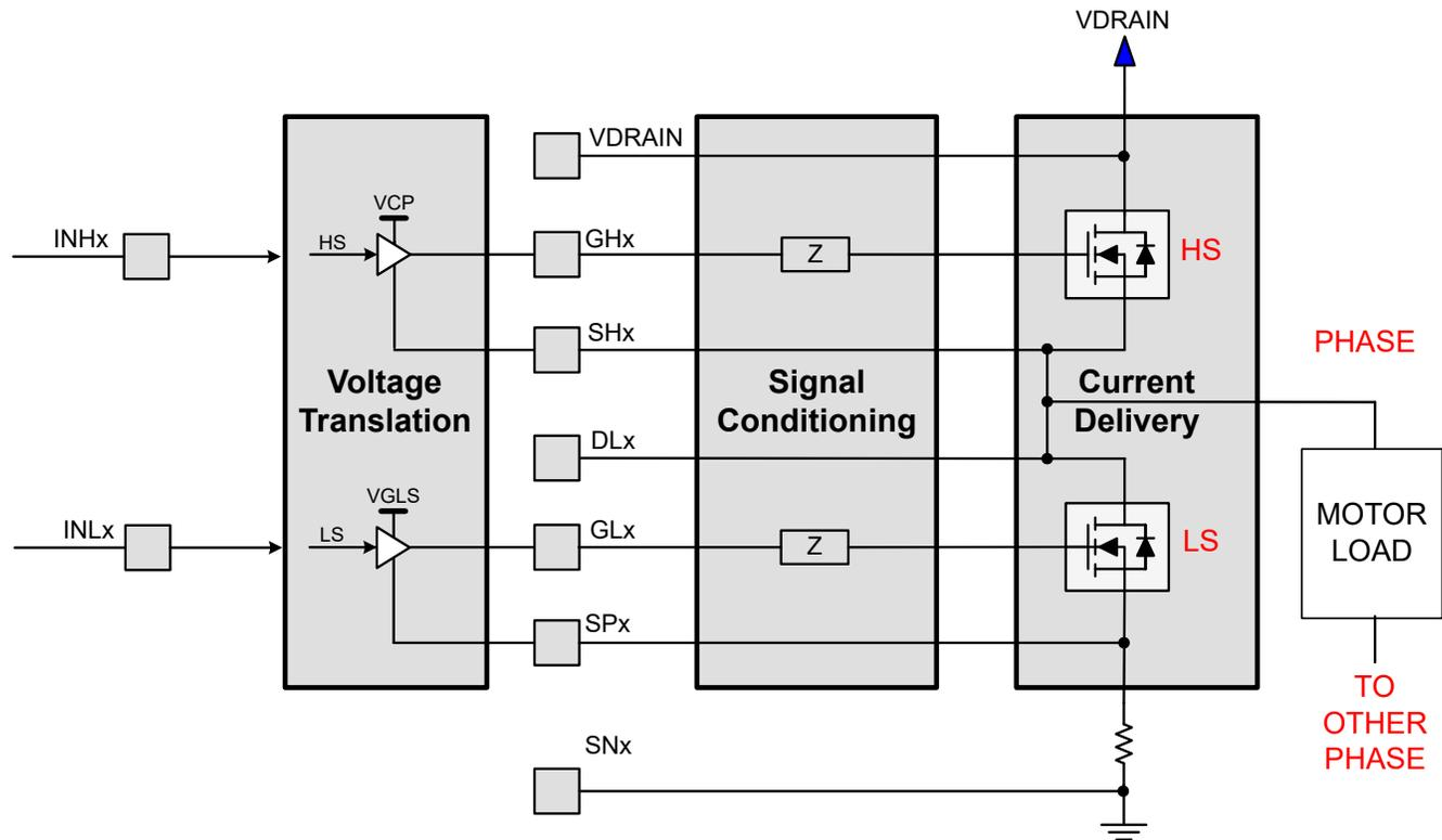
Figure 2-1. High-Level Power Stage
