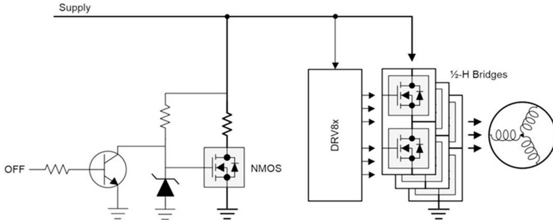
**Figure 7-2. Example Active Brake Circuit**
