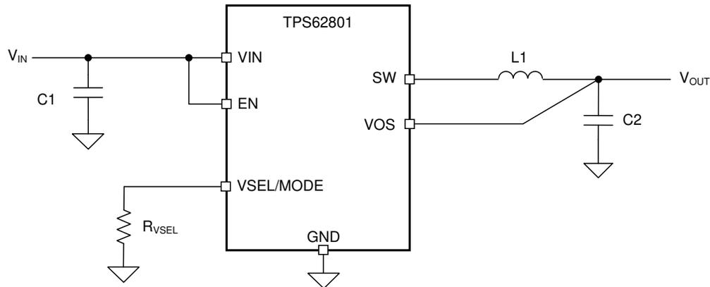
Figure 4-1. TPS62801 Typical Application Schematics
