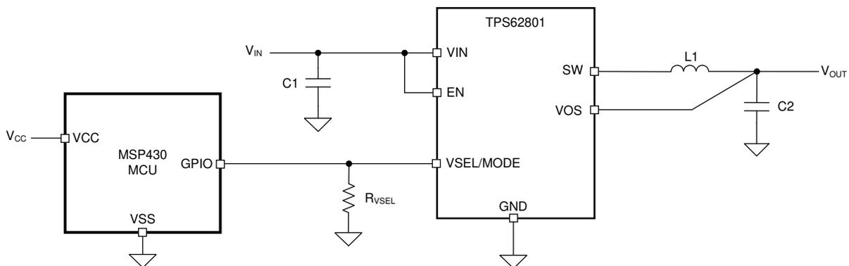
Figure 4-2. Typical Application Schematics, VSEL/MODE Driving Circuit with MCU
