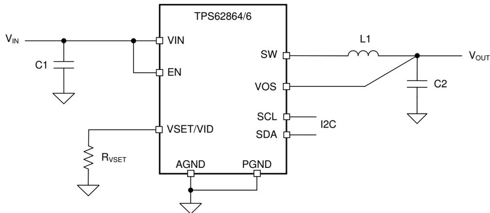
**Figure 1-1. TPS62864/6 Typical Application Schematics**
