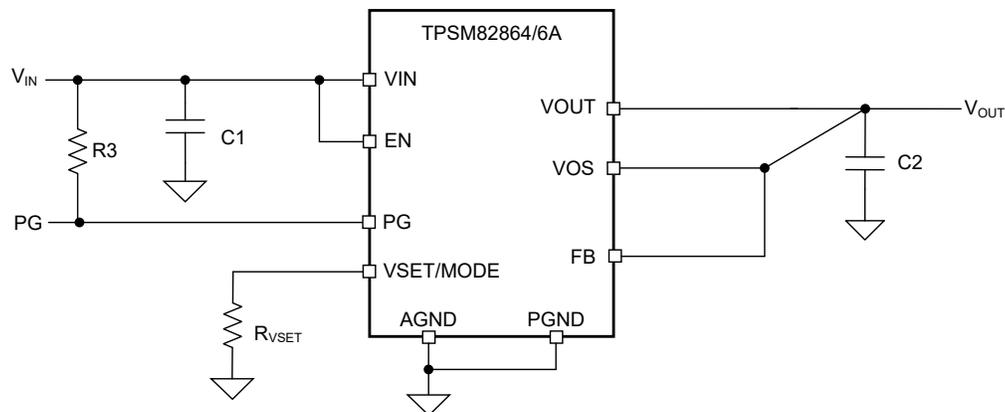
**Figure 5-2. Typical Application Schematic TPSM82864/6A - Fixed Output Voltage**
