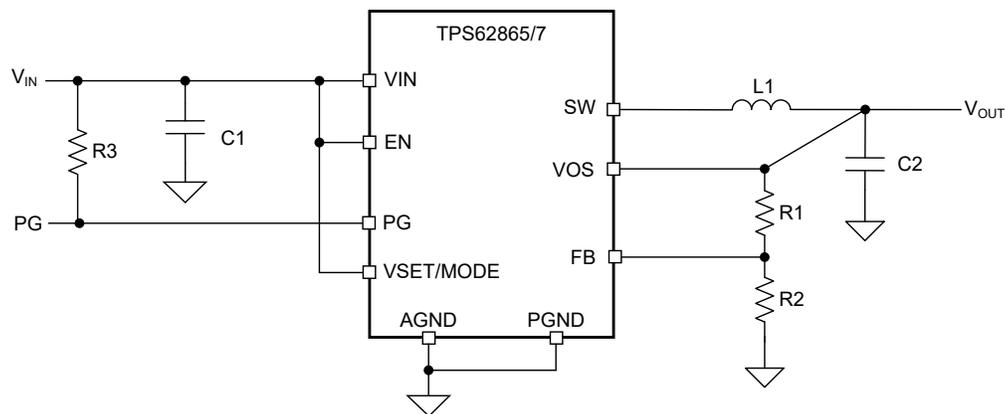
**Figure 5-3. Typical Application Schematics TPS62865/7 – Forced PWM Operation**
