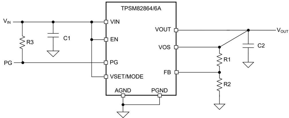
**Figure 5-4. Typical Application Schematics TPSM82864/6A – Forced PWM Operation**
