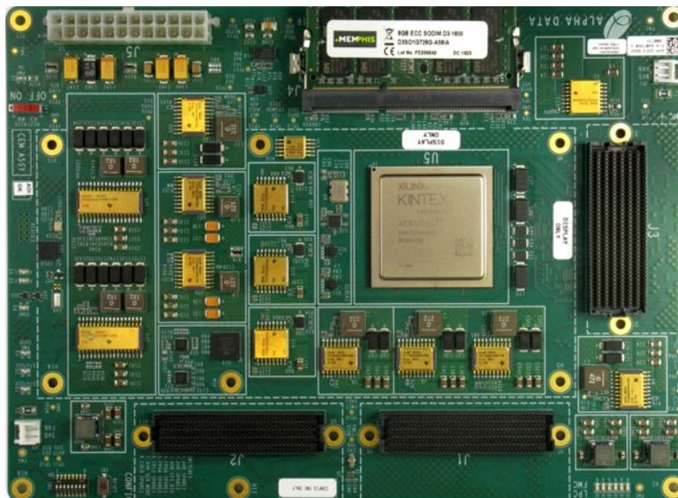
**Figure 5-1. The ADA-SDEV-KIT2 Platform for the KU060**
