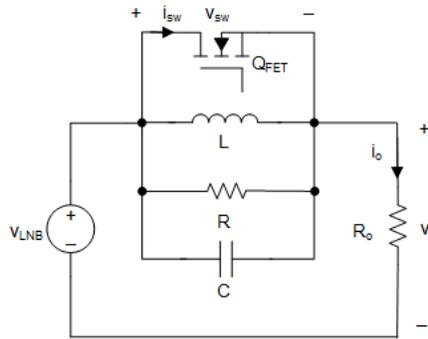
**Figure 3-1. Equivalent Circuit of DiSEqC™ 2.x Implementation**
