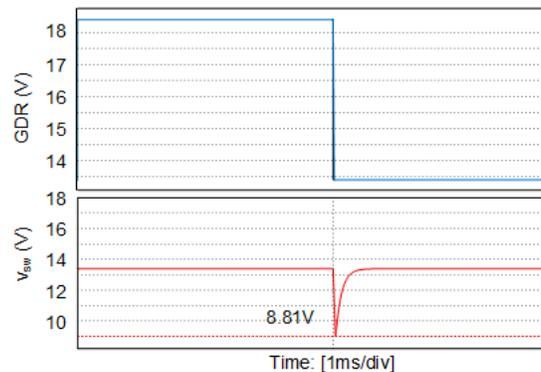
**Figure 3-4. Simulation Waveforms of Voltage Drop in DiSEqC™ 2.x Implementation**
