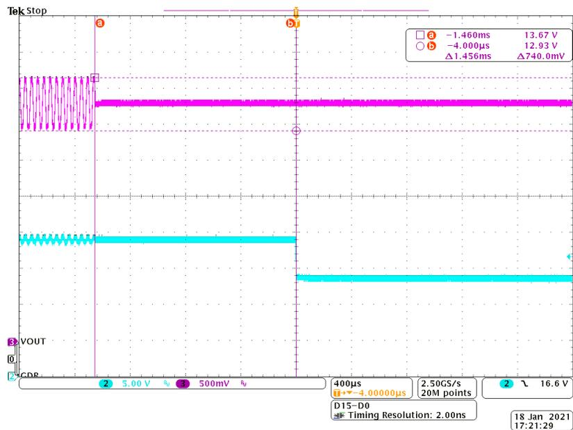
Figure 2-4. Inserting a 22-µF Blocking Capacitor Removes the Negative Spike Entirely
