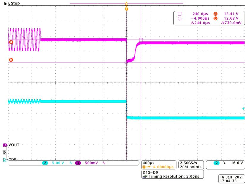
**Figure 1-2. Negative Voltage Spike Clamped to Approximately 700 mV by FET Body Diode**
