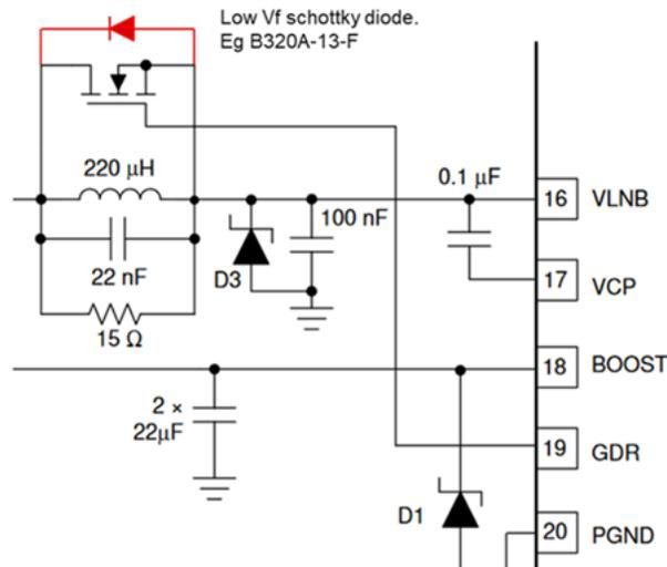
Figure 2-1. Schottky Diode Added to Clamp Negative Spike
