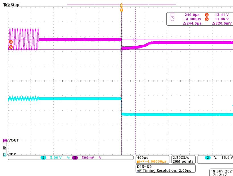
Figure 2-2. Spike Clamped to Approximately 330 mV by Adding Schottky Diode Across the FET
