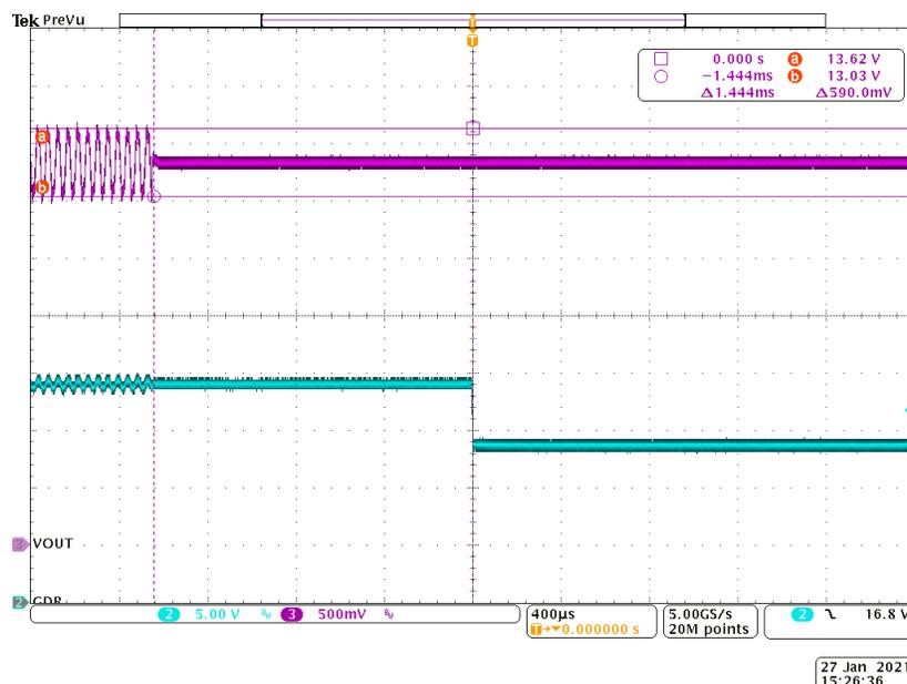
Figure 3-6. Experimental Results of DiSEqC™ 2.x Implementation With  $C_{add}$
