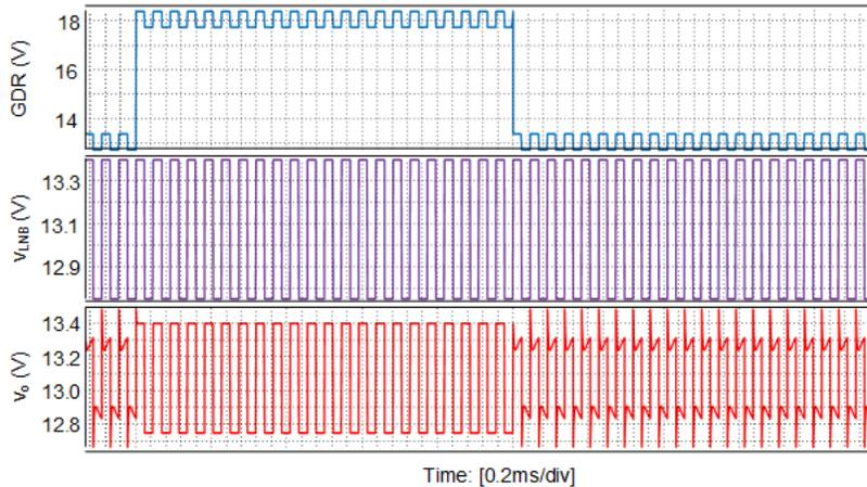
Figure 3-2. Simulation Waveforms of DiSEqC™ 2.x Implementation
