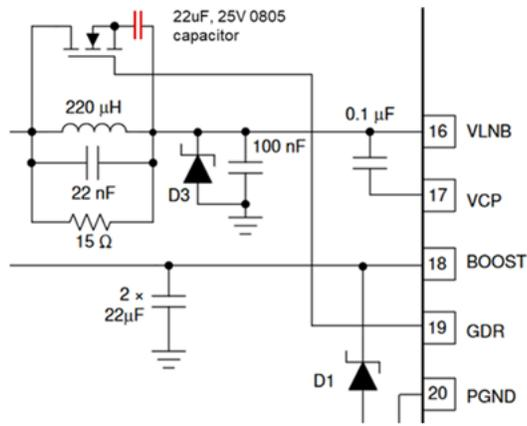
Figure 2-3. DC Blocking Capacitor Added in Series With FET
