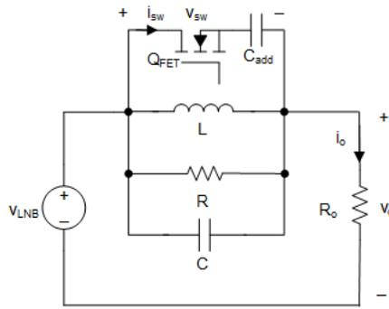
Figure 3-5. Equivalent Circuit of DiSEqC™ 2.x Implementation With  $C_{add}$
