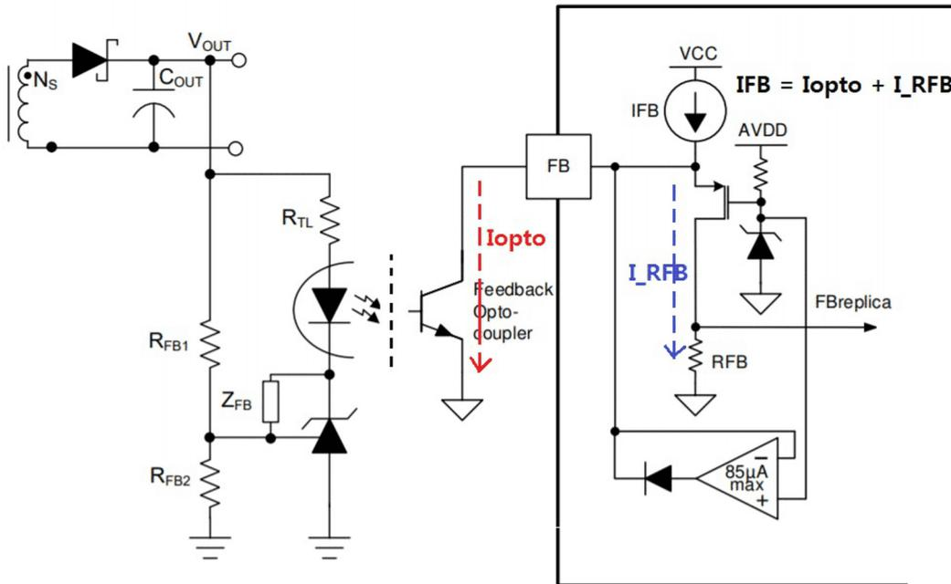
**Figure 2-2. Example of UCC25640x (High Side Current Sourcing)**
