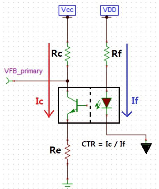
Figure 2-3. One Example of Biasing Optocoupler
