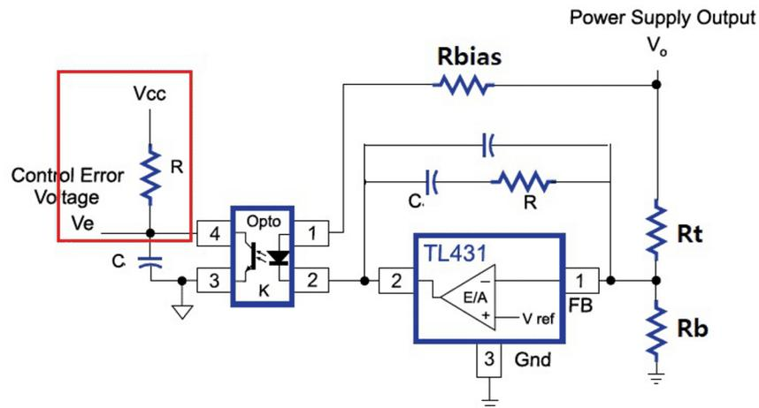
Figure 1-4. TL431 In Conjunction with Optocoupler for Isolated Feedback
