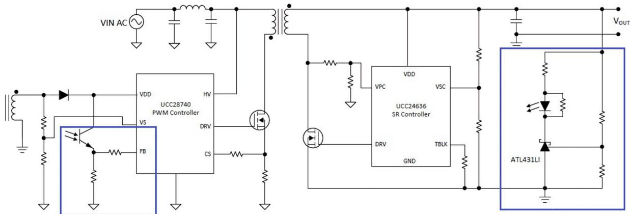
Figure 1-3. Flyback with Optocoupler Isolation with TL431
