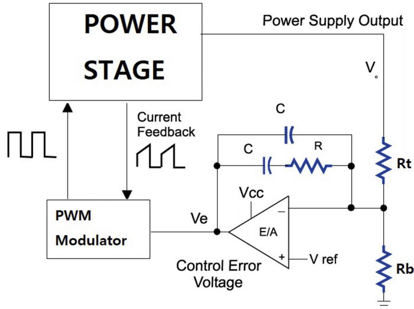
Figure 1-1. Feedback Loop in Non-Isolated Current-Mode Control Converter
