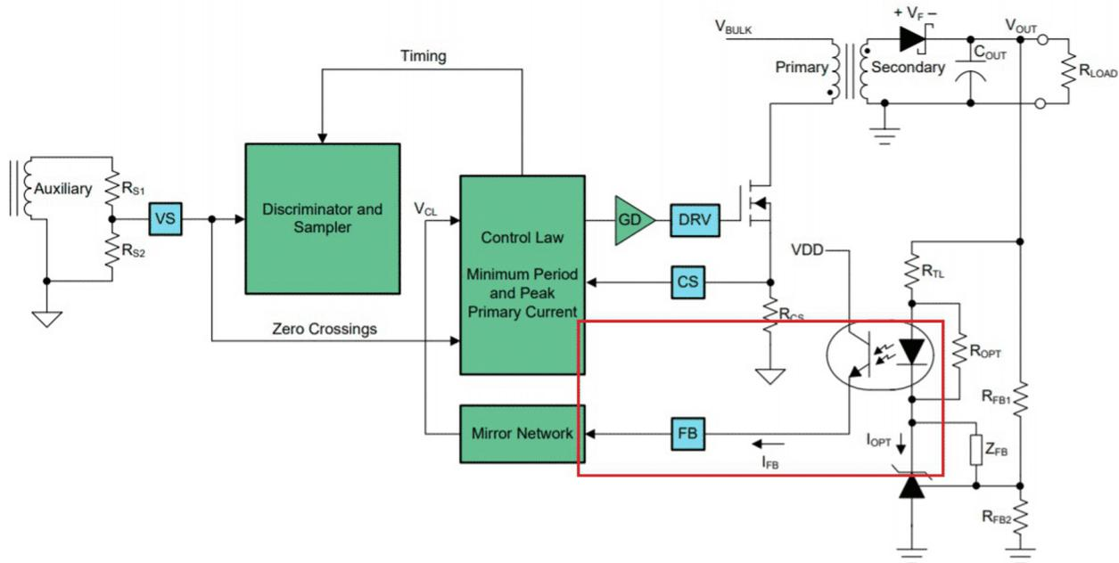
Figure 2-1. Example of UCC28740 (Low Side Current Sinking)
