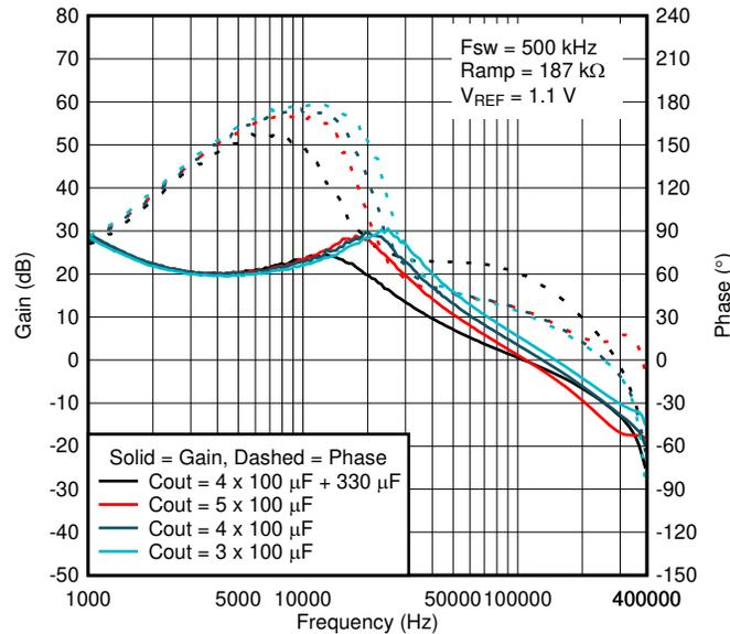
Figure 2-1. Bode plot for different  $C_{out}$  (12-V input, 1.8-V output)
