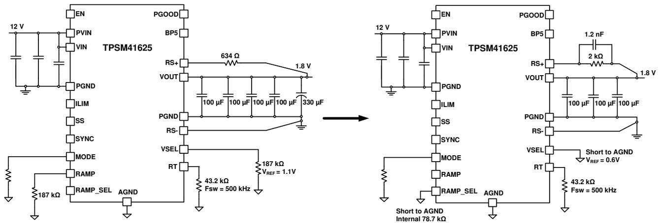
Figure 5-4. Original and Optimized 12-V input, 1.8-V output, 25-A, 500-kHz design with 3 x 100 µF of ceramic output capacitance
