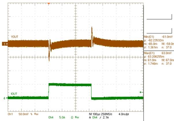
Figure 5-5. Load transient 0 to 5 A at 10 A/µs without  $C_{FF}$
