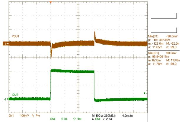
**Figure 5-7. Load transient 0 to 10 A at 10 A/μs with 1.2-nF C<sub>FF</sub>**
