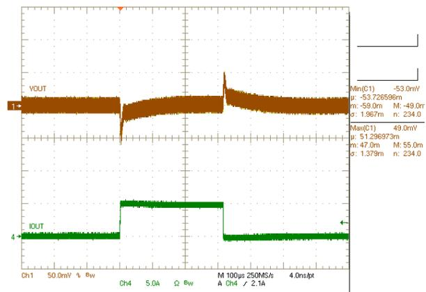
Figure 5-6. Load transient 0 to 5 A at 10 A/µs with 1.2-nF  $C_{FF}$
