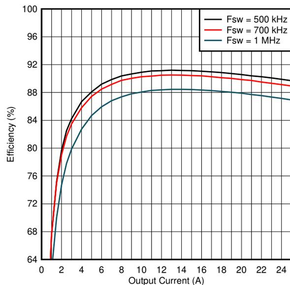
Figure 4-2. Efficiency for different switching frequency (12-V input, 1.8-V output)
