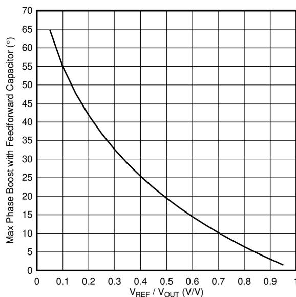
**Figure 5-1. Maximum phase boost with feedforward capacitor**
