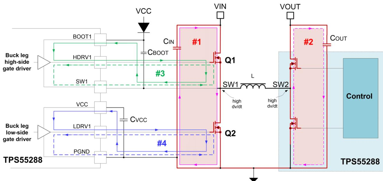
**Figure 2-2. Buck-boost Converter Schematic with Critical Loops**
