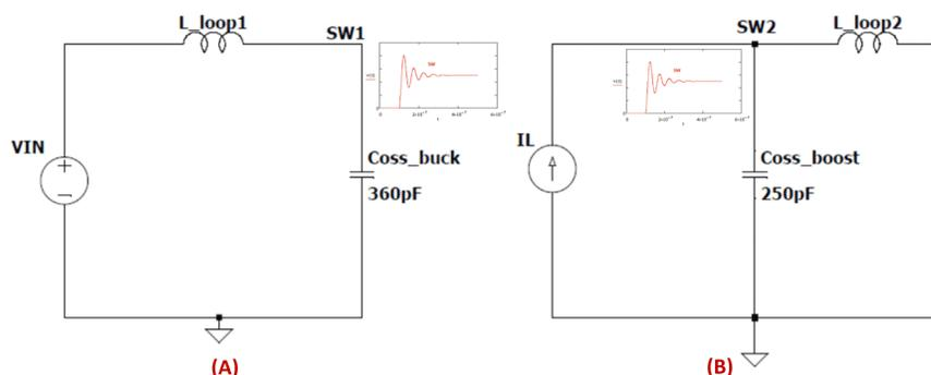
**Figure 2-10. Equivalent Model of the Switching Loop**
