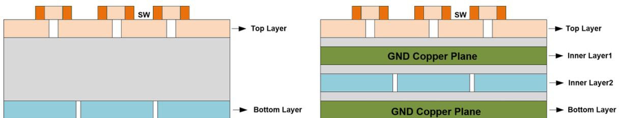
**Figure 2-3. Cross Section of Two-Layer Board and Four-Layer Board**
