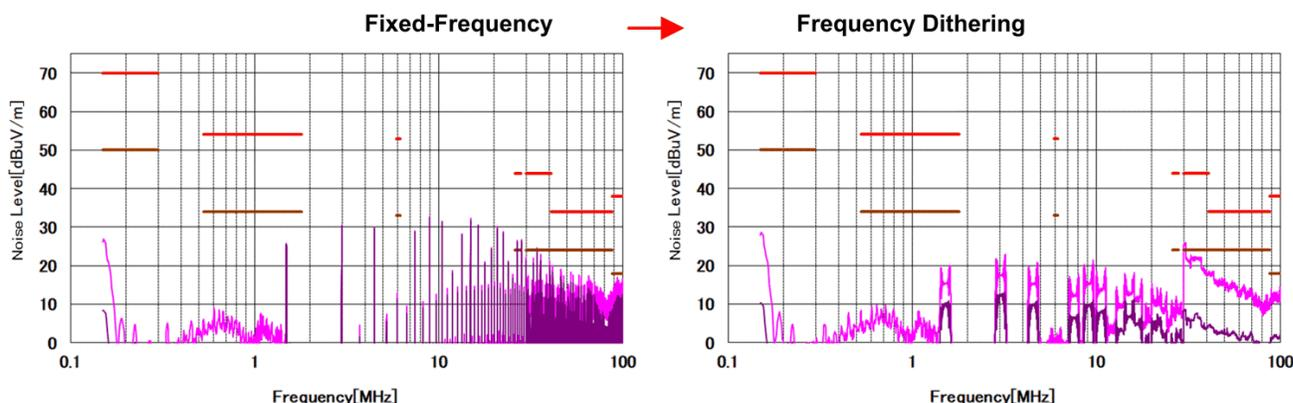
**Figure 2-9. Conduction EMI Comparison with Frequency Dithering**
