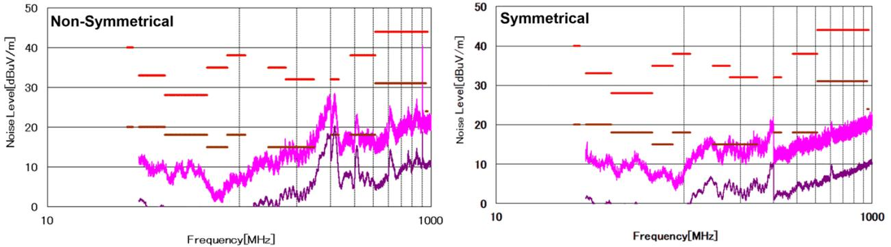
Figure 2-7. Radiated EMI Comparison with Symmetrical Placement
