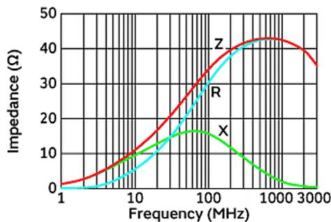
Figure 2-13. Impedance Characteristics of BLM21PG300SN1
