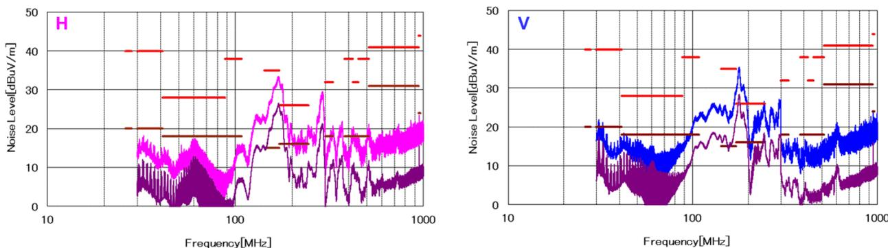
Figure 2-4. Radiated EMI Result of a 2-Layer PCB
