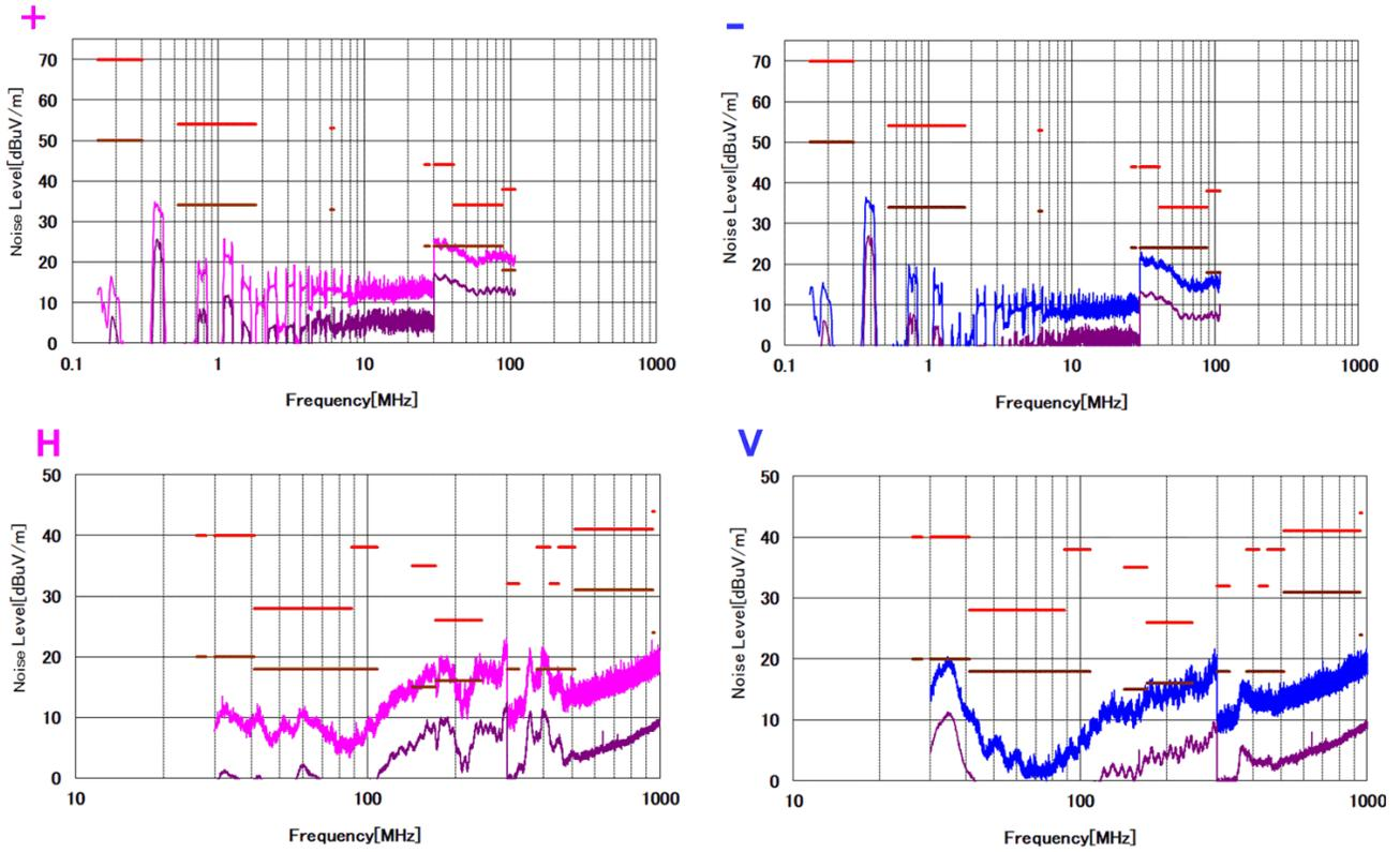
Figure 3-3. Boost Mode EMI Result (VIN = 12 V, VOUT = 20V / IOU = 3A)
