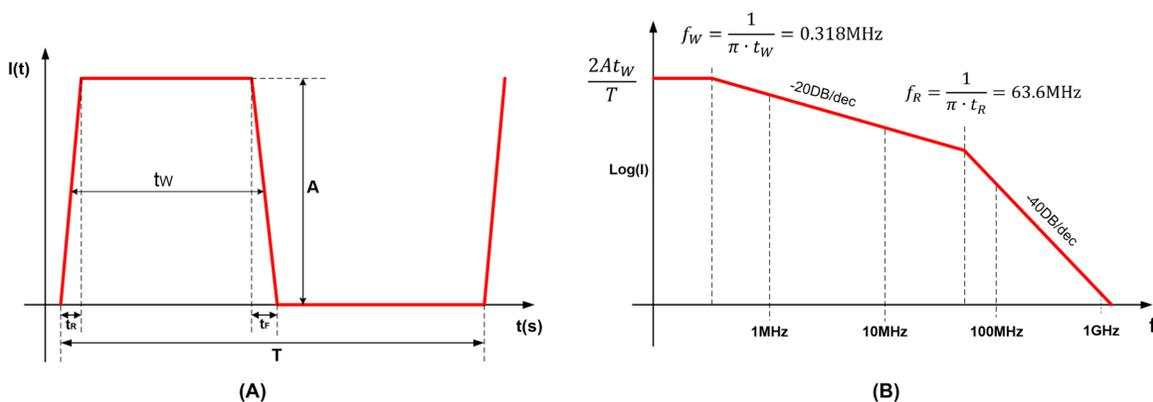
Figure 2-1. Harmonic Content of a Pulsed Current Waveform
