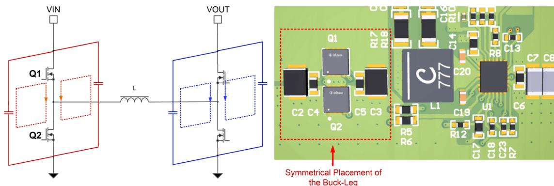
Figure 2-6. Symmetrical PCB Layout of TPS55288 Buck-Boost Converter
