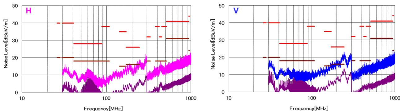
Figure 2-5. Radiated EMI Result of a 4-Layer PCB
