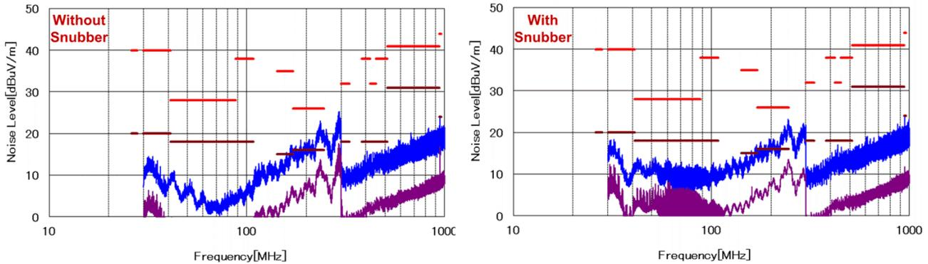
Figure 2-11. Radiation EMI Comparison with and without RC snubber
