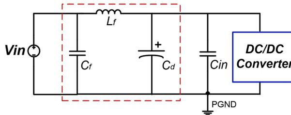
Figure 2-12. Simplified Input EMI Filter
