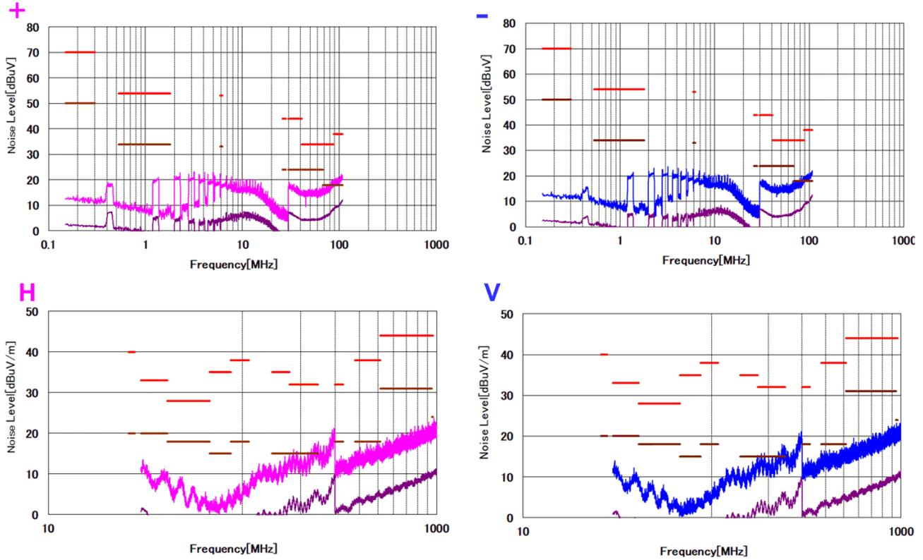
**Figure 3-2. Buck Mode EMI Result (VIN = 12 V, VOUT = 5V / IOUT = 3A)**
