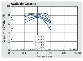
Figure 1. Tadiran SL-2870 Capacity
