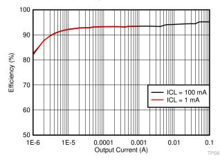
Figure 4. TPS63900 Efficiency With ICL Active
