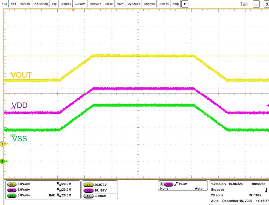
Figure 3.  $V_{in}$  9-V to 16-V Line Transient Waveform
