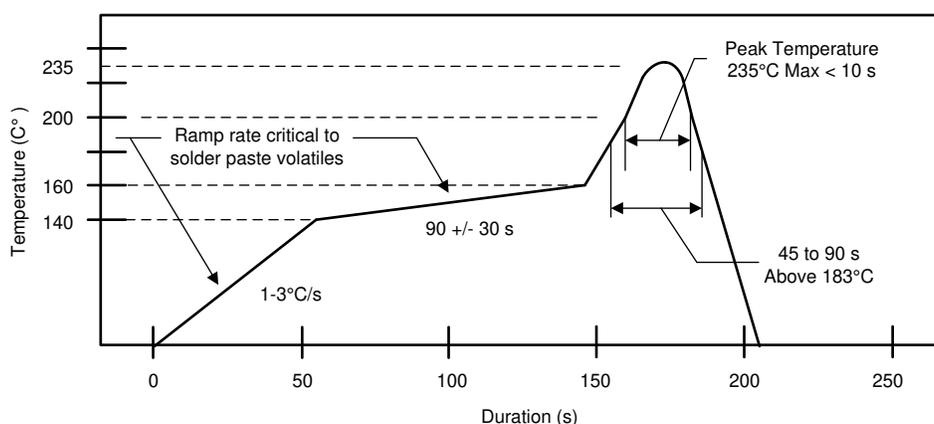
**Figure 1-1. Starting Profile for Typical Pb/Sn Solder Paste**
