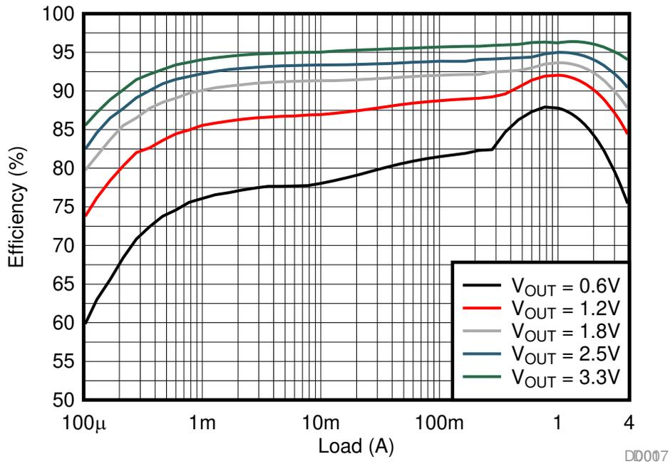
Figure 2. Efficiency vs. Load at VIN=5V
