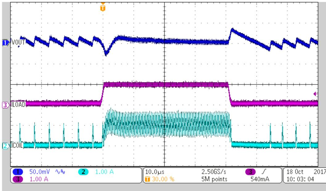
Figure 3. Load transient Performance with  $I_{out} = 0.05A$  to  $1A$
