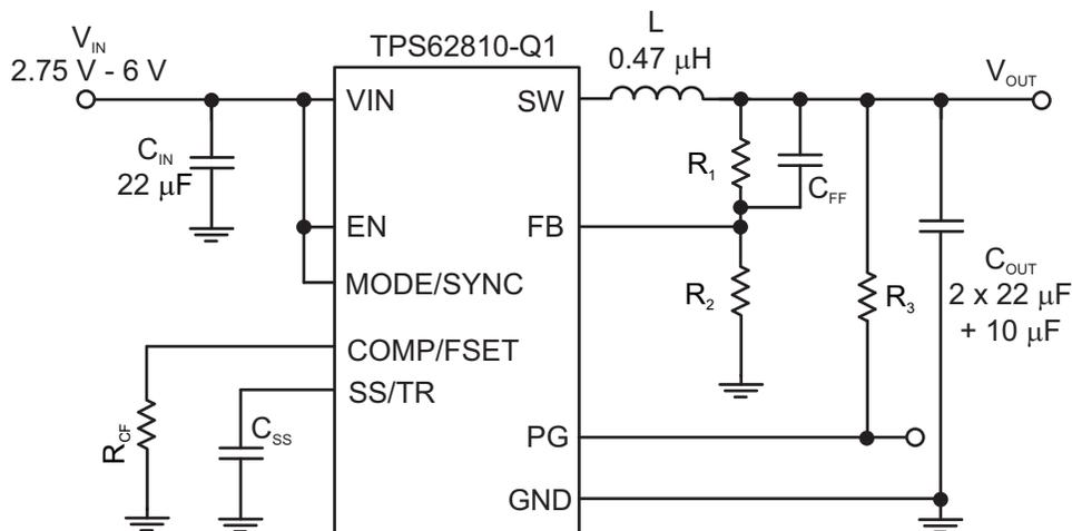
**Figure 1. Typical TPS6282X Application Circuit**
