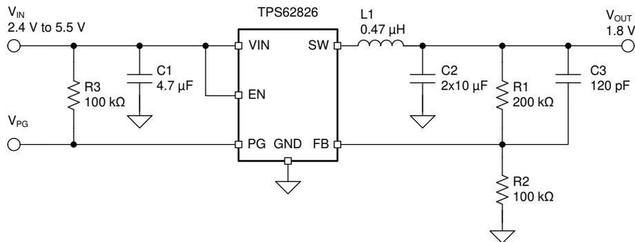
Figure 4. Typical TPS6281X Application Circuit
