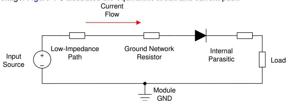
**Figure 1-5. Equivalent Current Path**
