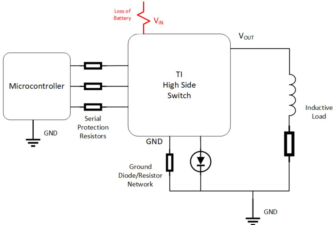
**Figure 2-3. Series Resistor Protection**
