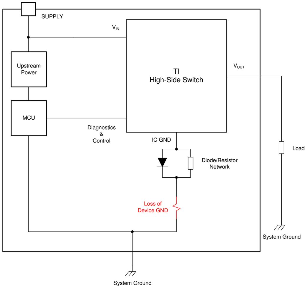
**Figure 1-1. Loss of Device Ground**
