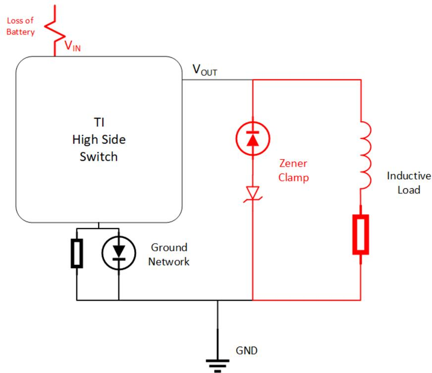
Figure 2-2. Zener Diode for Inductive Loading
