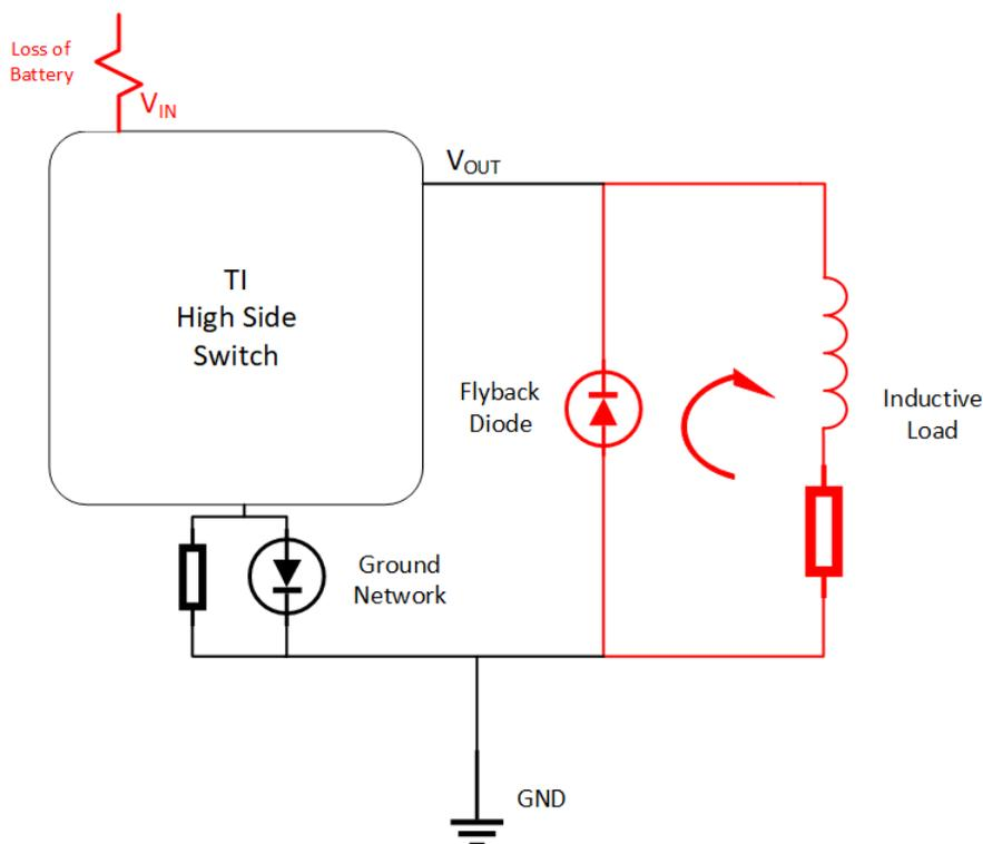
**Figure 2-1. Current Path for Flyback Diode**
