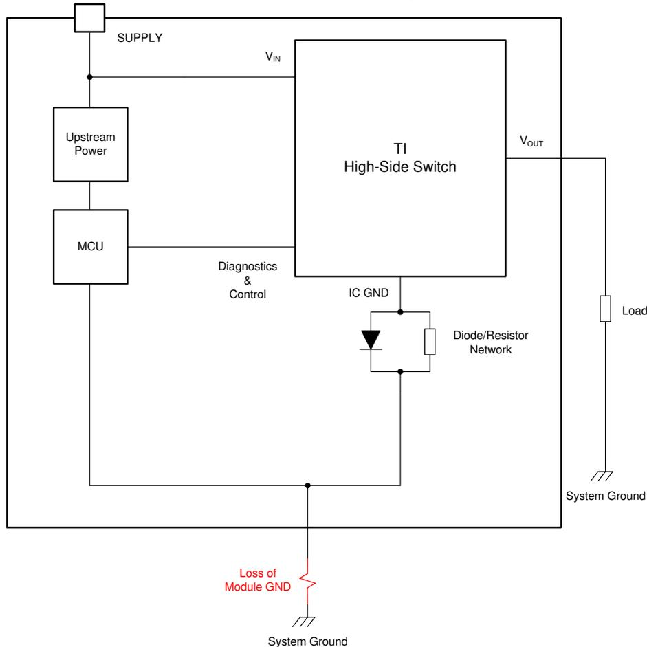
**Figure 1-2. Loss of Module Ground**
