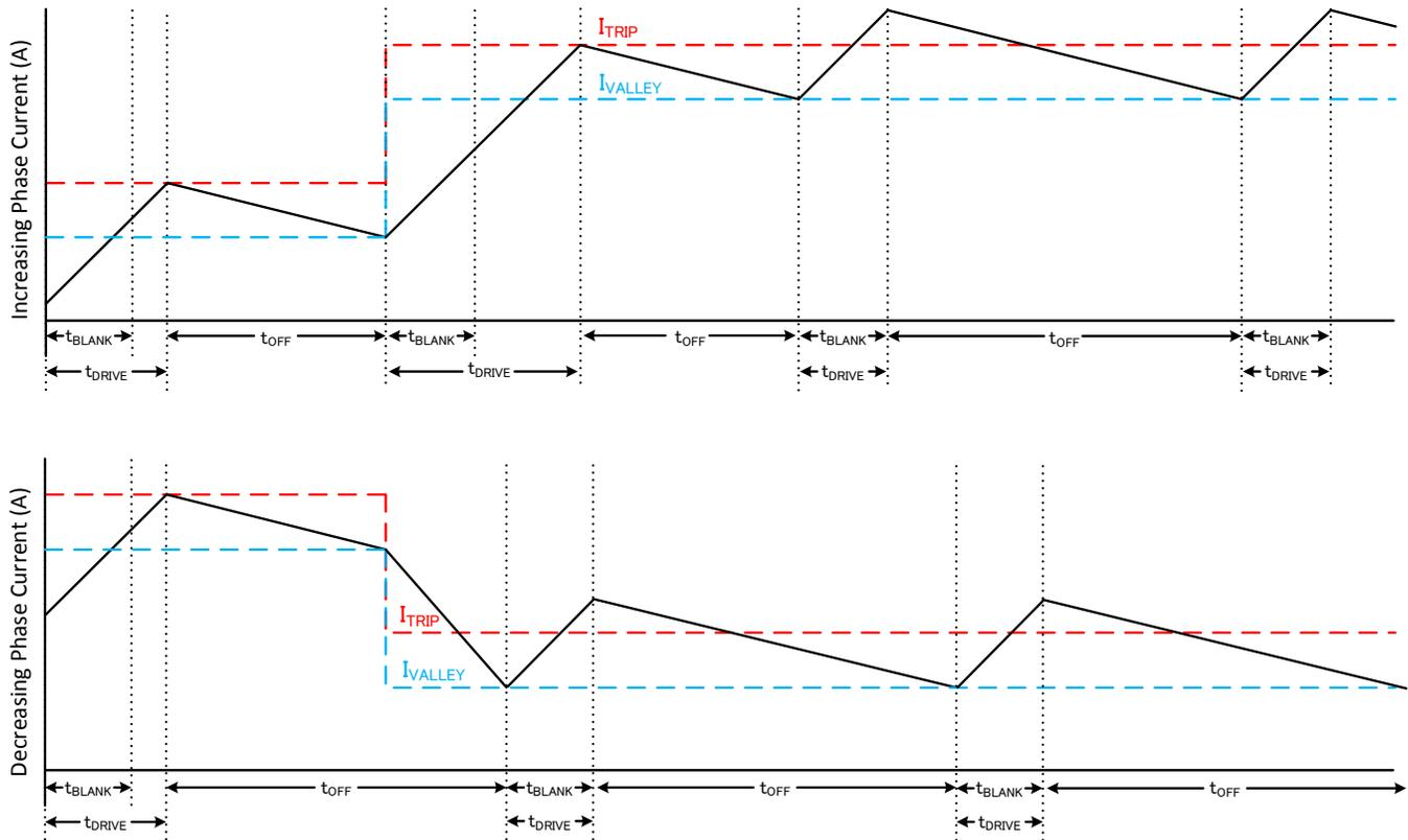
Figure 9. Smart tune Ripple Control Decay Mode
