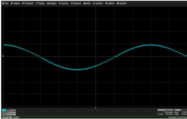
**Figure 18. Smoothness of Zero-Cross at 1/16 Microstepping**
