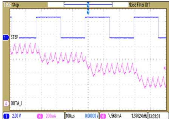
Figure 6. Microstepping Current vs STEP Input, Mixed Decay
