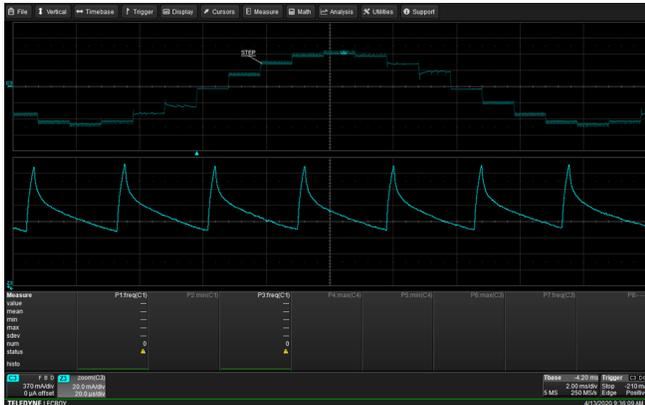
Figure 14. PWM at 100% Level, PWM Frequency is 35 kHz
