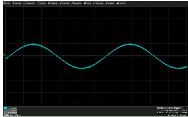
**Figure 19. Smoothness of Zero-Cross at 1/64 Microstepping**
