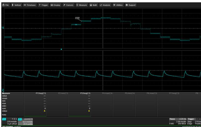
Figure 12. PWM at 38% Level, PWM Frequency is 55 kHz
