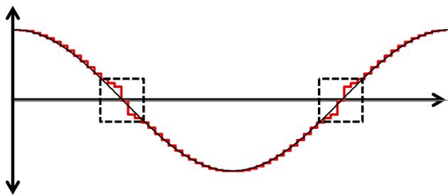
Figure 16. Current Distortion Due to High Blanking Time
