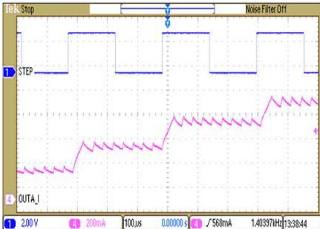
Figure 5. Microstepping Current vs STEP Input, Slow Decay
