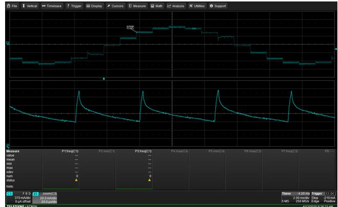
Figure 15. PWM at 92% Level (decreasing), PWM Frequency is 25 kHz
