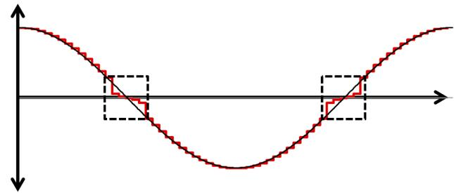
Figure 17. Current Distortion Due to High OFF Time
