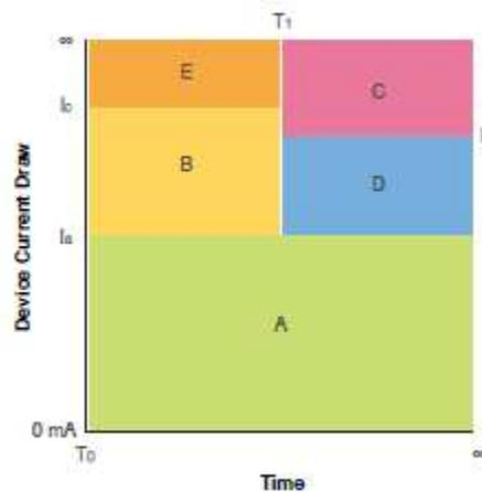
**Figure 1. Overcurrent and Short Circuit Protection**
