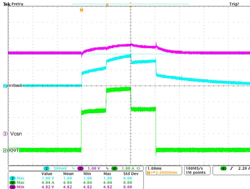
Figure 16. Set 2.88A Current Limit for 2.4A Port Without External FET
