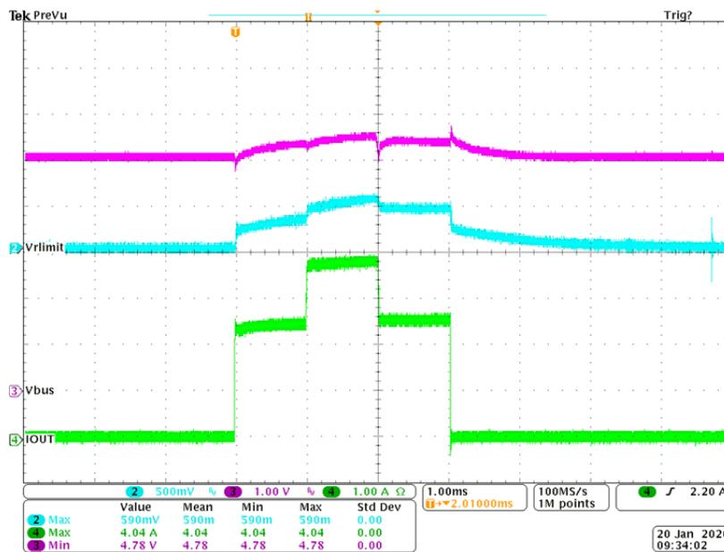
Figure 15. Set 2.88A Current Limit for 2.4A Port With External FET
