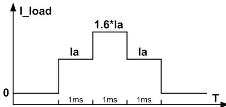
**Figure 2. Load Waveform of MFi OCP Test**
