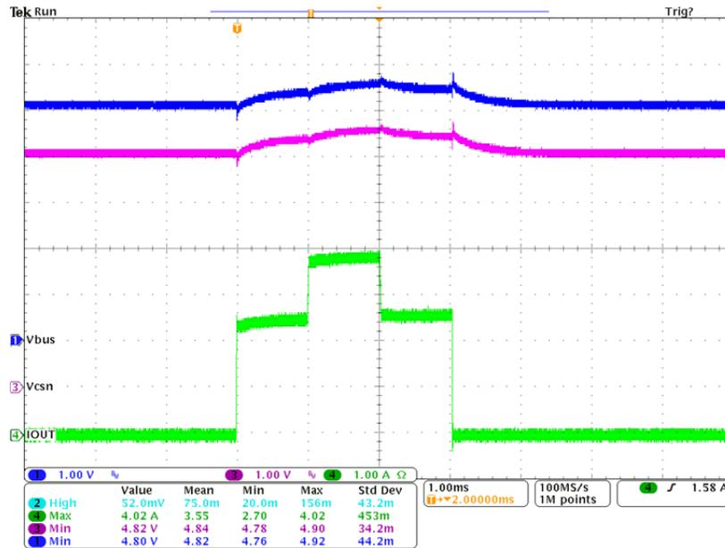
Figure 7. Set 3.96A Current Limit for 2.4A Port
