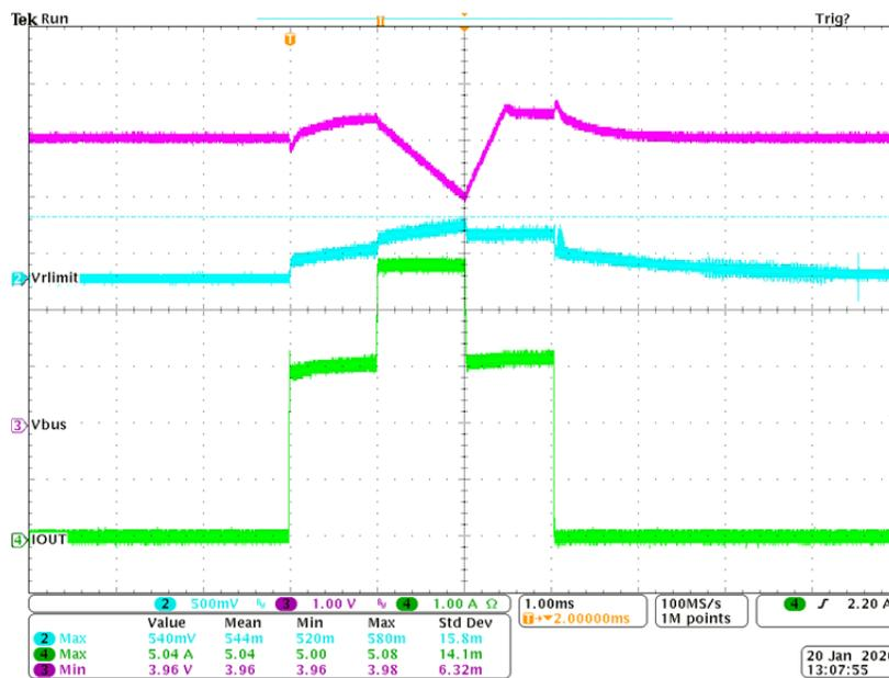
Figure 17. Set 3.5A Current Limit for 3A Port With External FET
