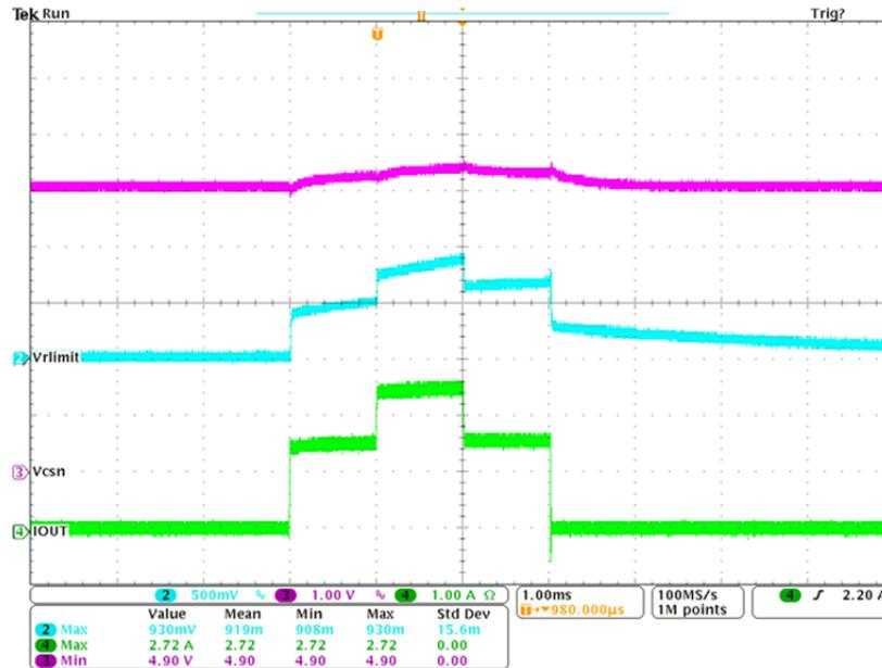
Figure 12. Set 1.8A Current Limit for 1.5A Port Without External FET
