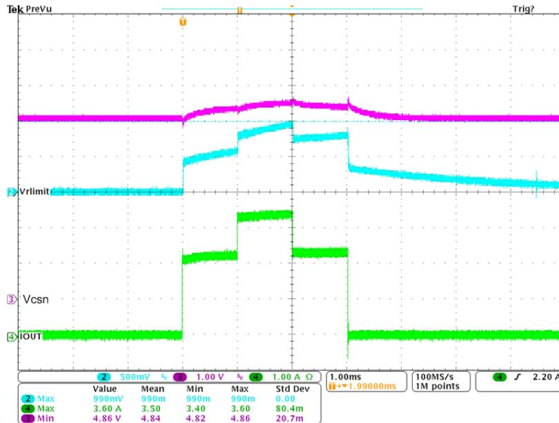
Figure 14. Set 2.52A Current Limit for 2.1A Port Without External FET
