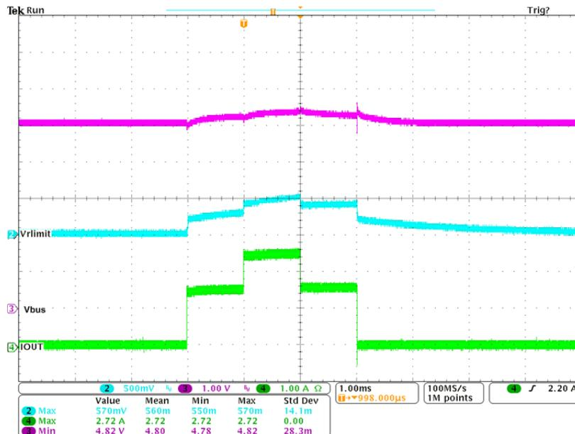
Figure 11. Set 1.8A Current Limit for 1.5A Port With External
