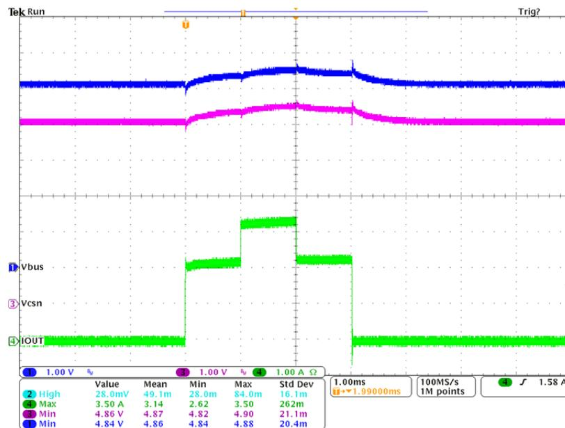
Figure 6. Set 3.45A Current Limit for 2.1A Port
