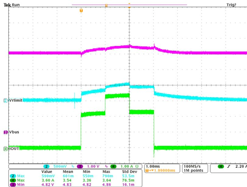
Figure 13. Set 2.52A Current Limit for 2.1A Port With External
