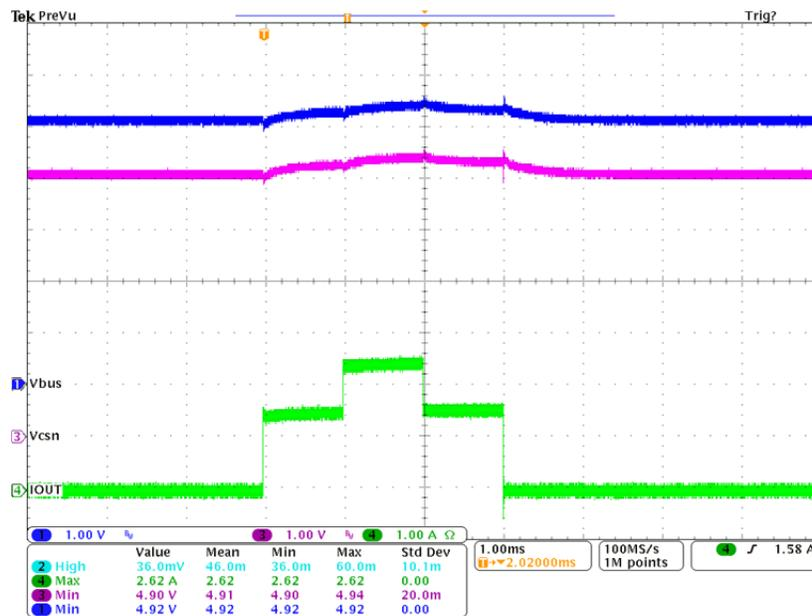
Figure 5. Set 2.45A Current Limit for 1.5A Port
