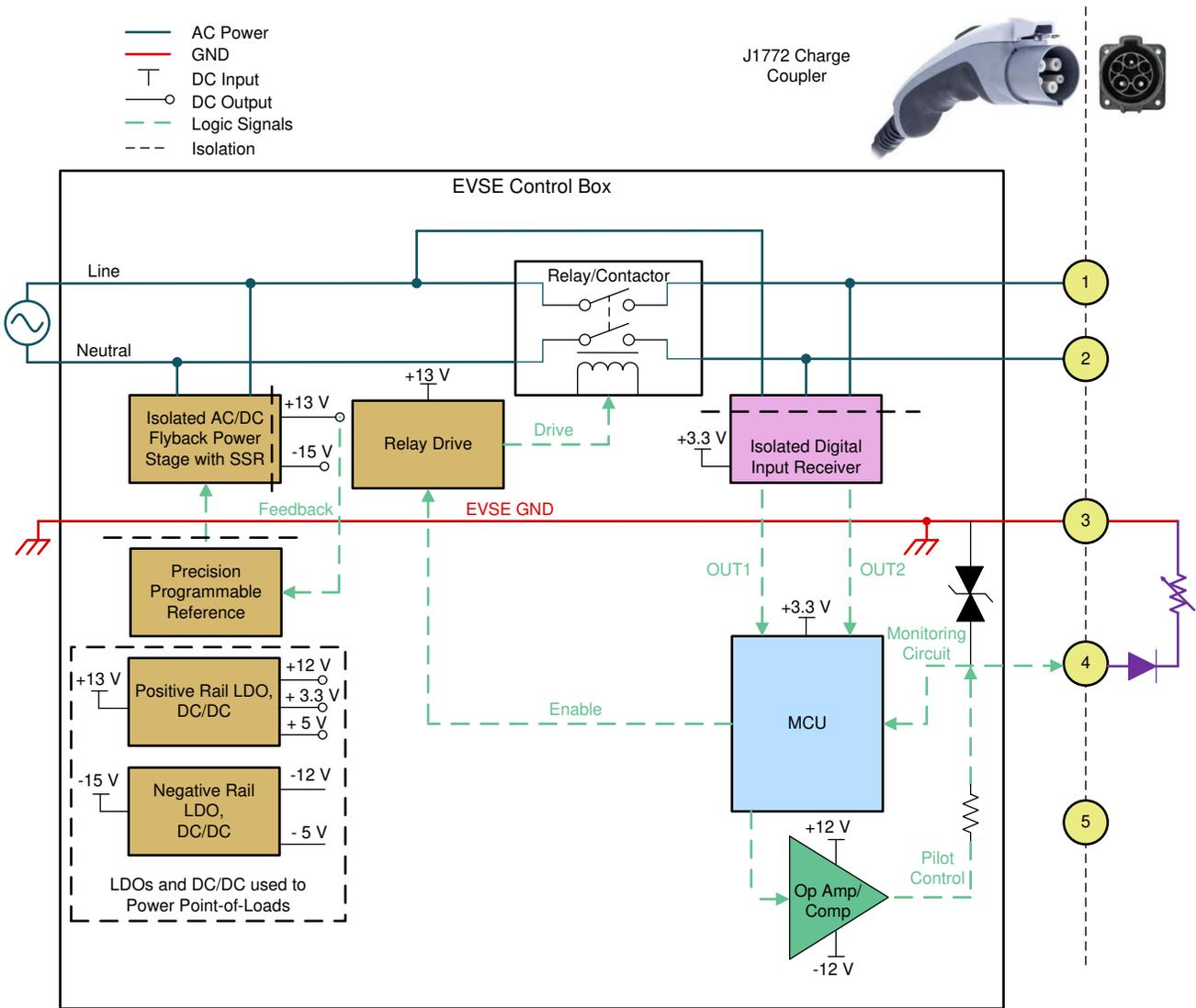
AC/DC leakage current detection sub-systems are not shown in this implementation.
