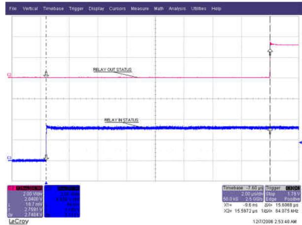
Figure 4-3. Delay Between Digital Outputs of ISO1212
