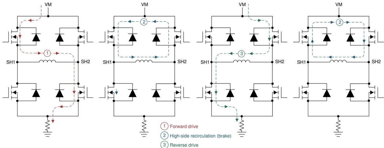
**Figure 3-1. H-Bridge Configuration Utilized to Drive a Solenoid**
