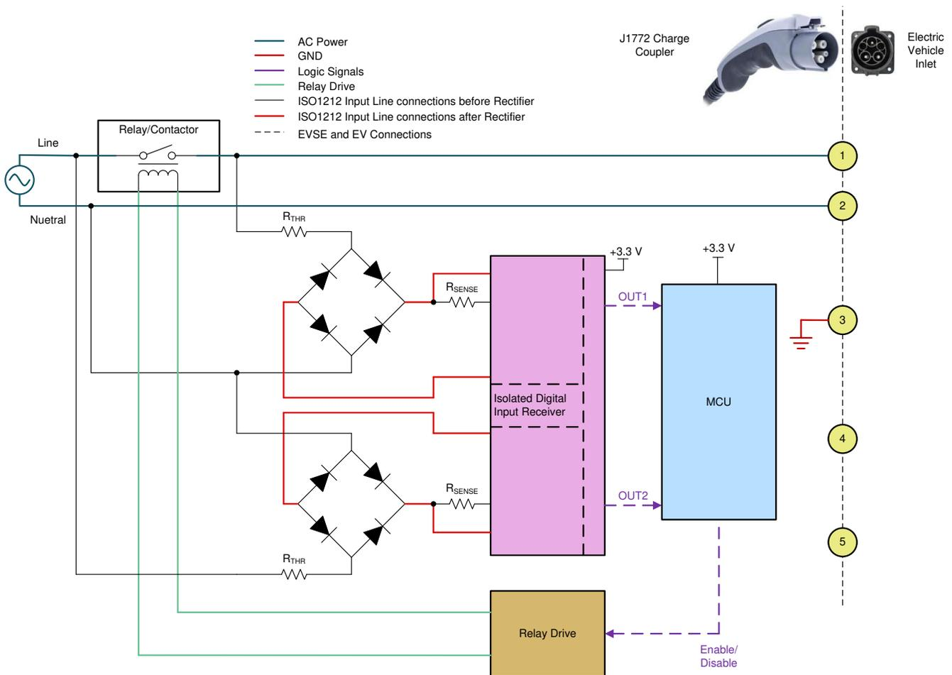
Control pilot interface, auxiliary power tree, and AC/DC leakage current detection sub-system are not shown in this implementation.
