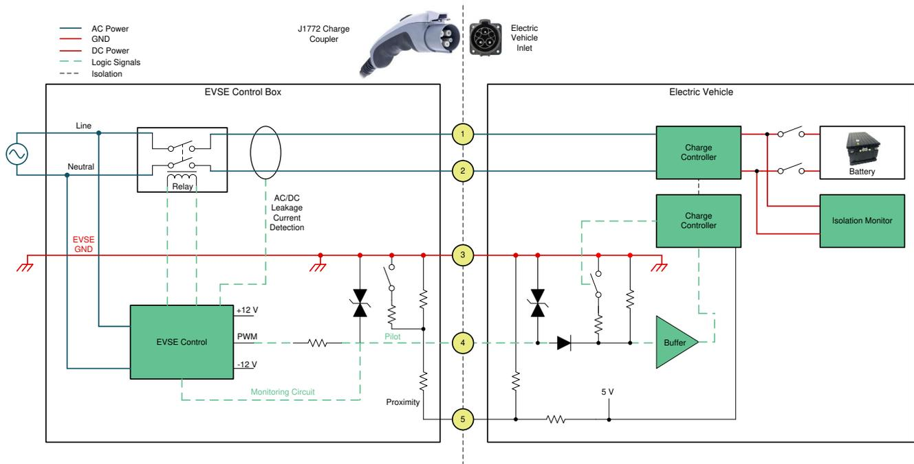
**Figure 1-1. AC Level 1 and Level 2 System Configuration**
