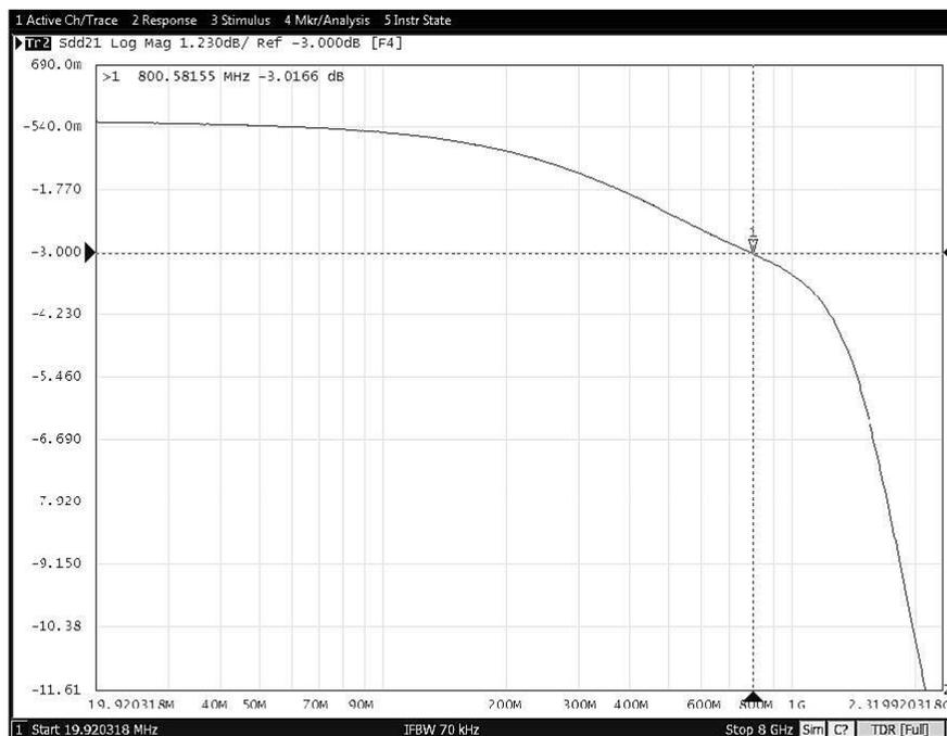
Figure 1. Data Transmission Characteristics vs Frequency
