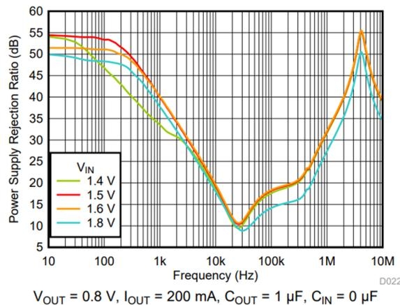
**Figure 3-2. PSRR Curve of TPS7A05 at 200 mA Load Current and 0.8 V Output Voltage**
