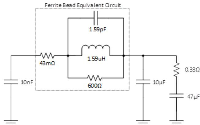
**Figure 3-5. PI Filter Circuit Diagram**
