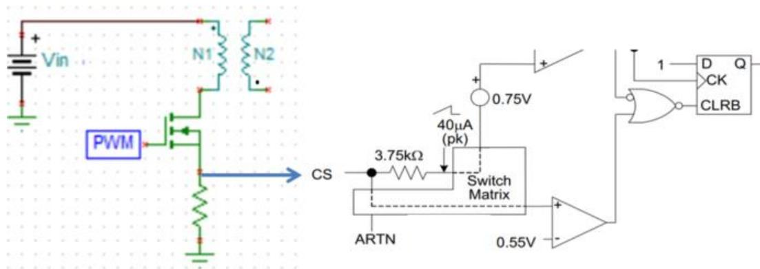
**Figure 1. Traditional Flyback Current Limit Scheme**
