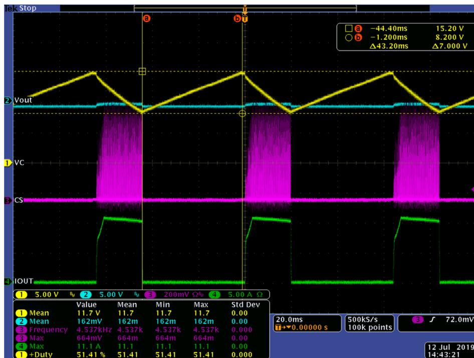
Figure 5. The original hiccup OCP waveform
