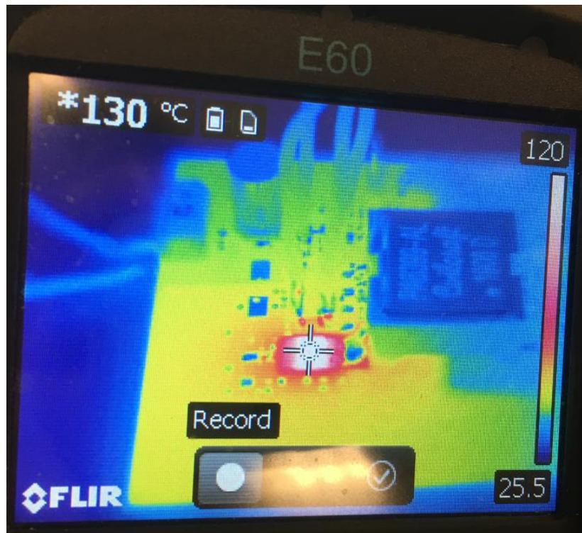
Figure 6. IR thermal photo with original hiccup OCP mode
