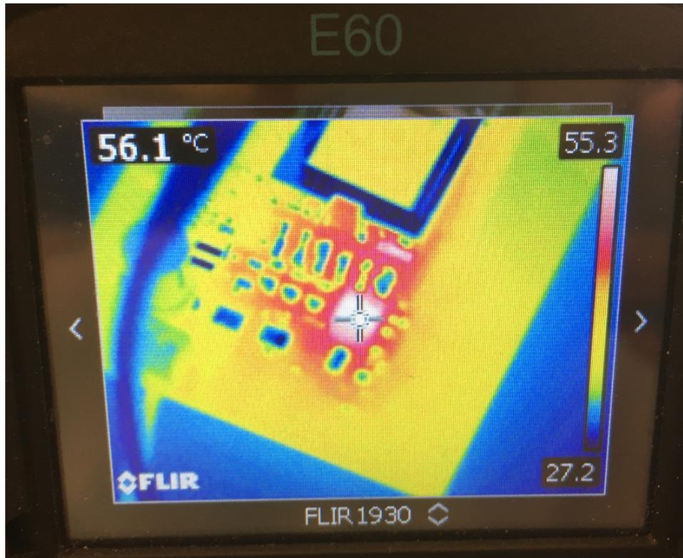
Figure 9. IR Thermal Photo with External Hiccup OCP Circuit
