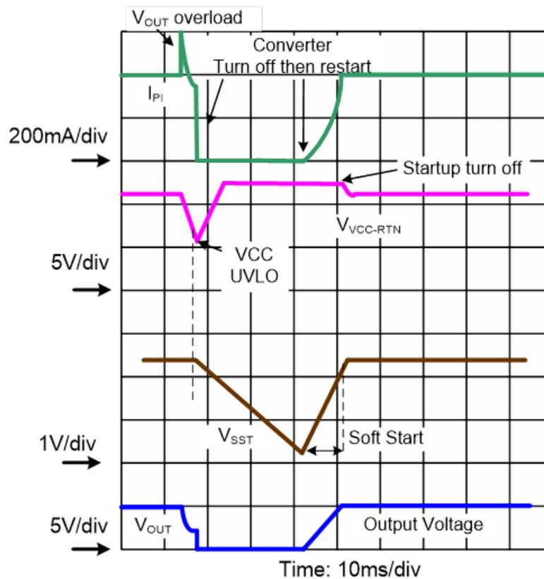
Figure 11. TPS2373x Restart Following Severe Overload at Main Output of PSR Flyback DC-DC Converter
