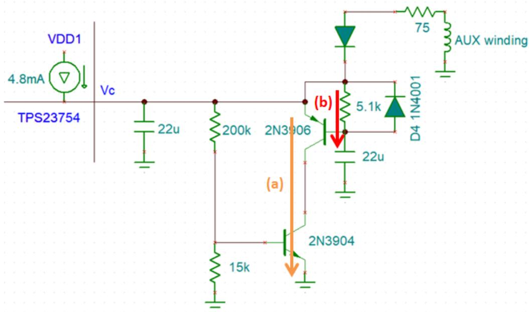
Figure 7. The External Discrete Hiccup Circuit
