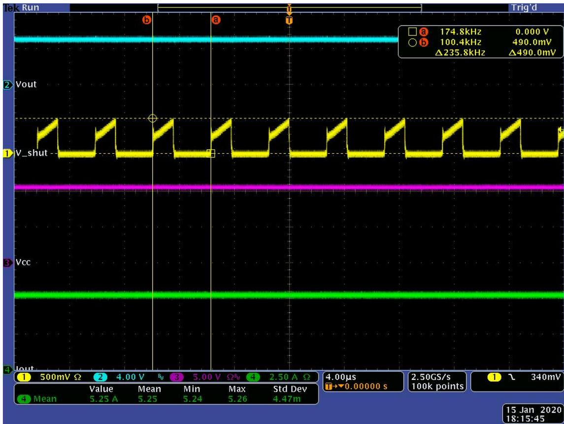
Figure 2. Peak current signal on current shunt resistor
