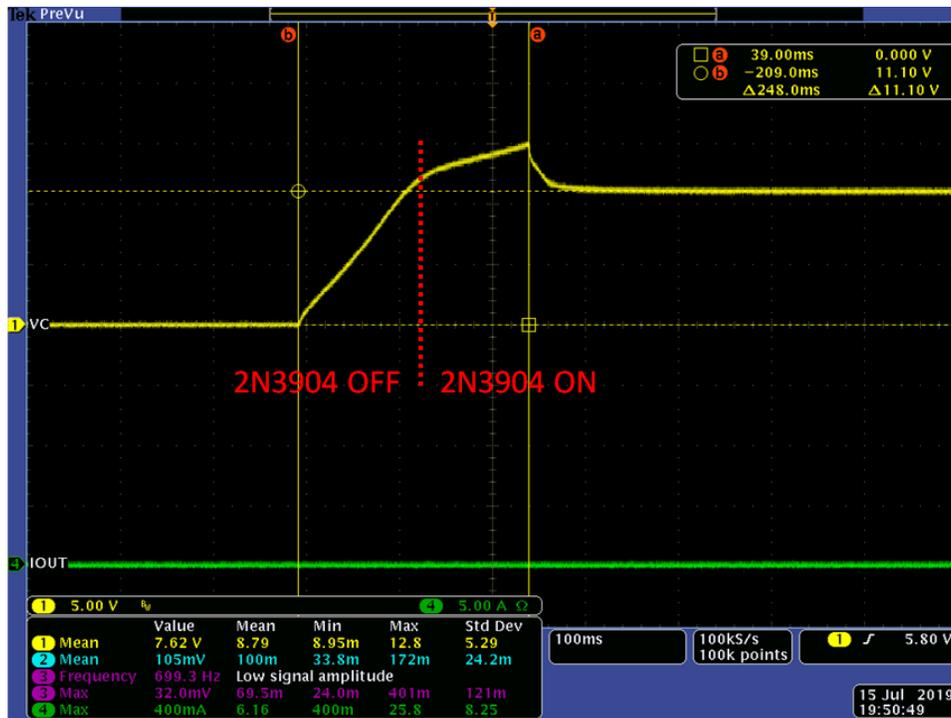
Figure 10. Startup Waveform with External Discrete Hiccup Circuit
