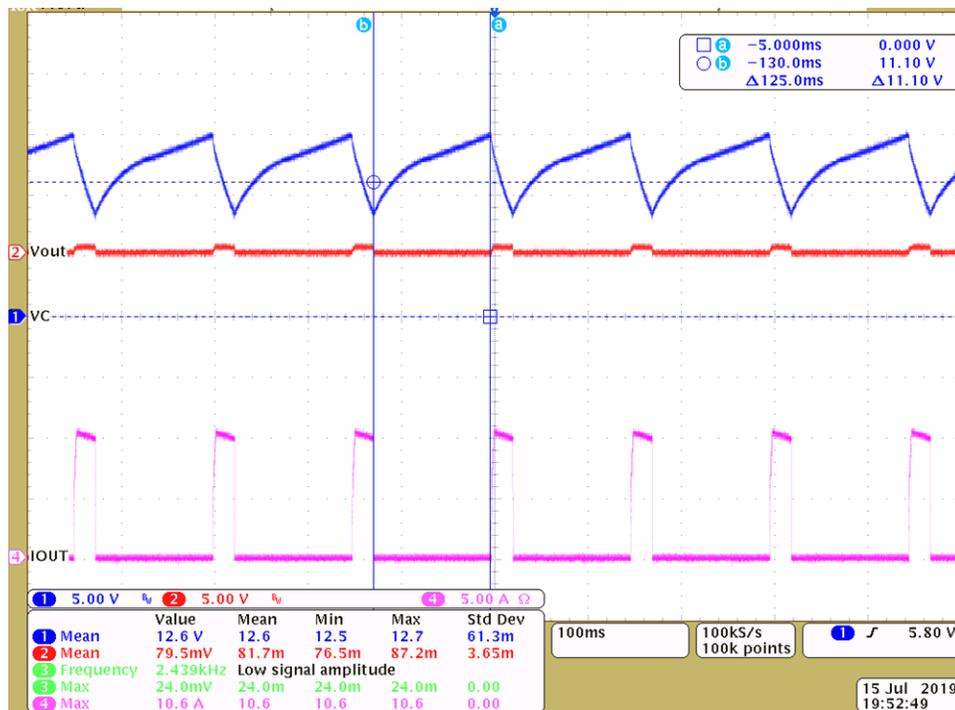
Figure 8. The Hiccup OCP Waveform with External Hiccup Circuit
