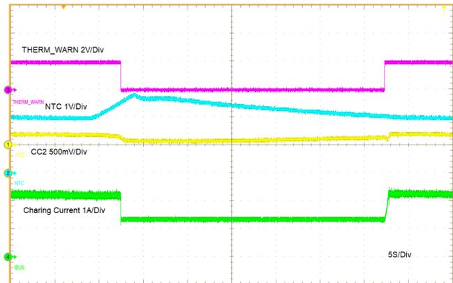
Figure 13. Active Current Limit In Type-C Port
