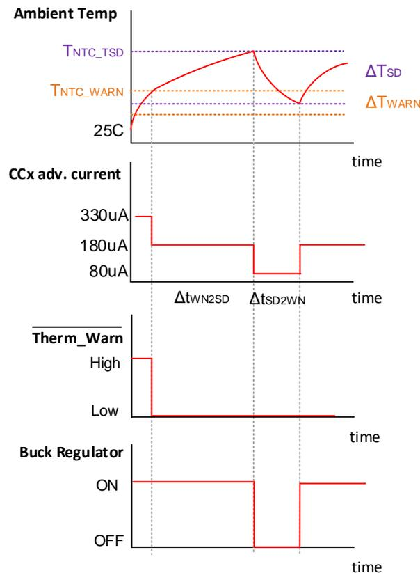
**Figure 10. TPS25831-Q1 Behavior When Trigger NTC Threshold**
