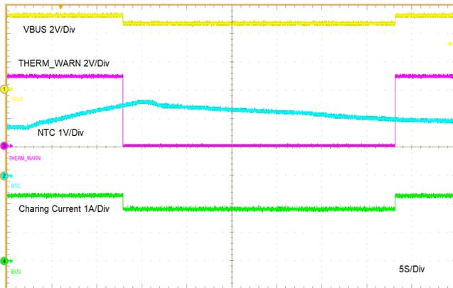
Figure 12. Active Current Limit In Type-A Port
