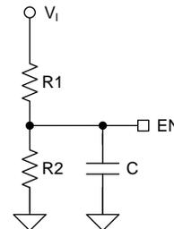
Figure 4. Setting Input Cutoff Voltage and Delayed Start-up
