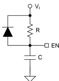
Figure 3. Adding Diode to Quickly Discharge C
