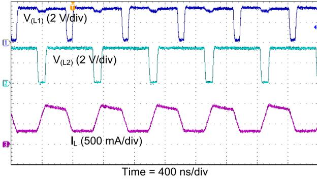
Figure 5. Typical Buck-Boost Mode Waveforms for the TPS63802 at  $V_i = V_o = 3.3\text{ V}$ ,  $I_o = 0.5\text{ A}$
