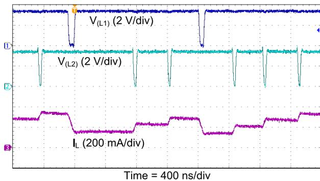
Figure 3. Typical Buck-Boost Mode Waveforms for the TPS63020 at  $V_i = V_o = 3.3\text{ V}$ ,  $I_o = 0.5\text{ A}$
