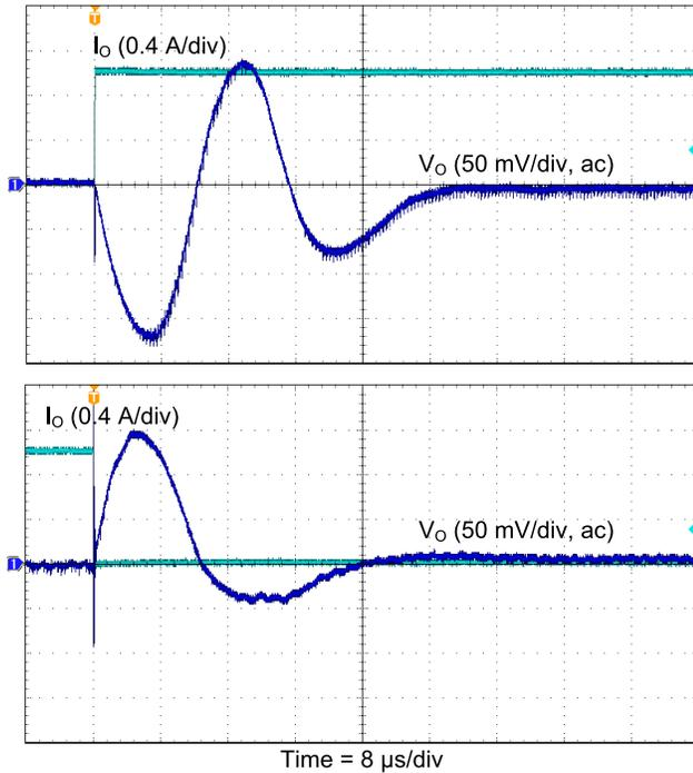
Figure 9. Load Transient Response for the TPS63020 at  $V_i = V_o = 3.3\text{ V}$ ,  $\Delta I_o = \pm 1\text{ A}$
