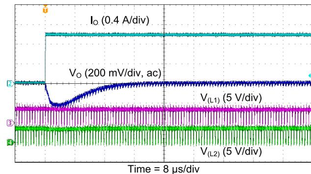
Figure 12. Mode Change Due to Load Transient for the TPS63802 at  $V_i = V_o = 3.3\text{ V}$ ,  $\Delta I_o = 1\text{ A}$
