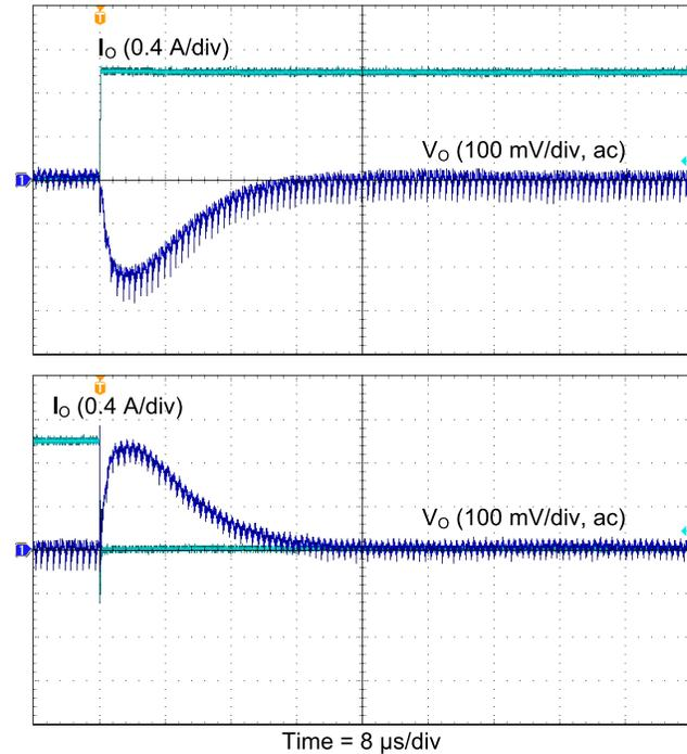
Figure 10. Load Transient Response for the TPS63802 at  $V_i = V_o = 3.3\text{ V}$ ,  $\Delta I_o = \pm 1\text{ A}$
