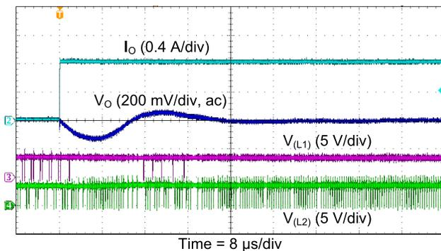
Figure 11. Mode Change Due to Load Transient for the TPS63020 at  $V_i = V_o = 3.3\text{ V}$ ,  $\Delta I_o = 1\text{ A}$
