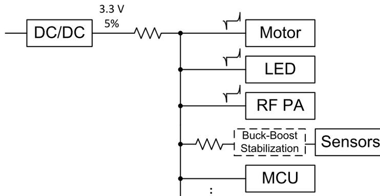
Figure 1. An Example of a Power Branch
