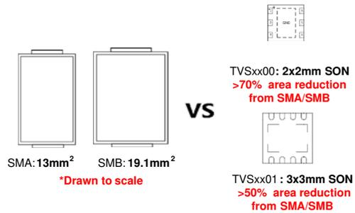
**Figure 4. Flat Clamp Package Size Comparison**
