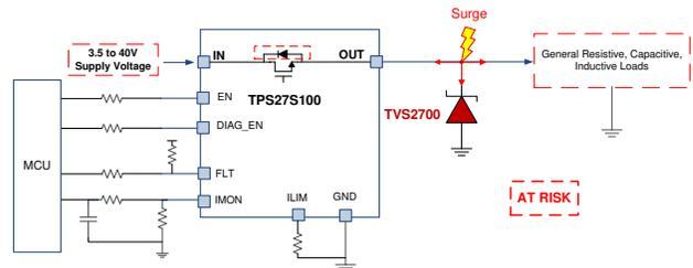
Figure 2. Digital Output Module Components
