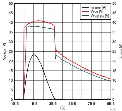
**Figure 3. Surge Waveform for TVS3300 vs Conventional TVS**
