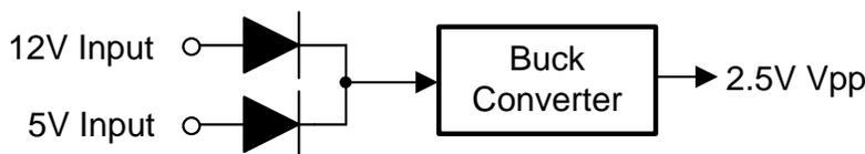
**Figure 2. Simplified Schematic of DDR Vpp Supply**
