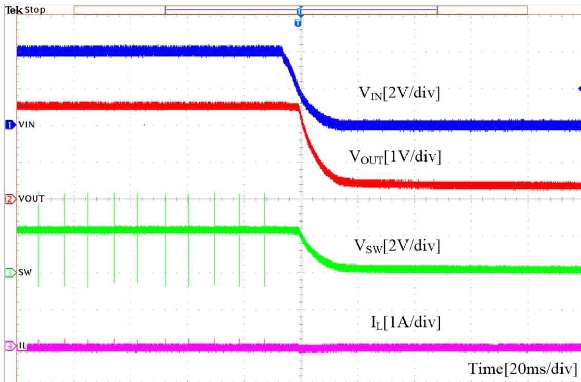
Figure 9. Shut Down, V<sub>IN</sub> = 4 V, I<sub>OUT</sub> = 0 A
