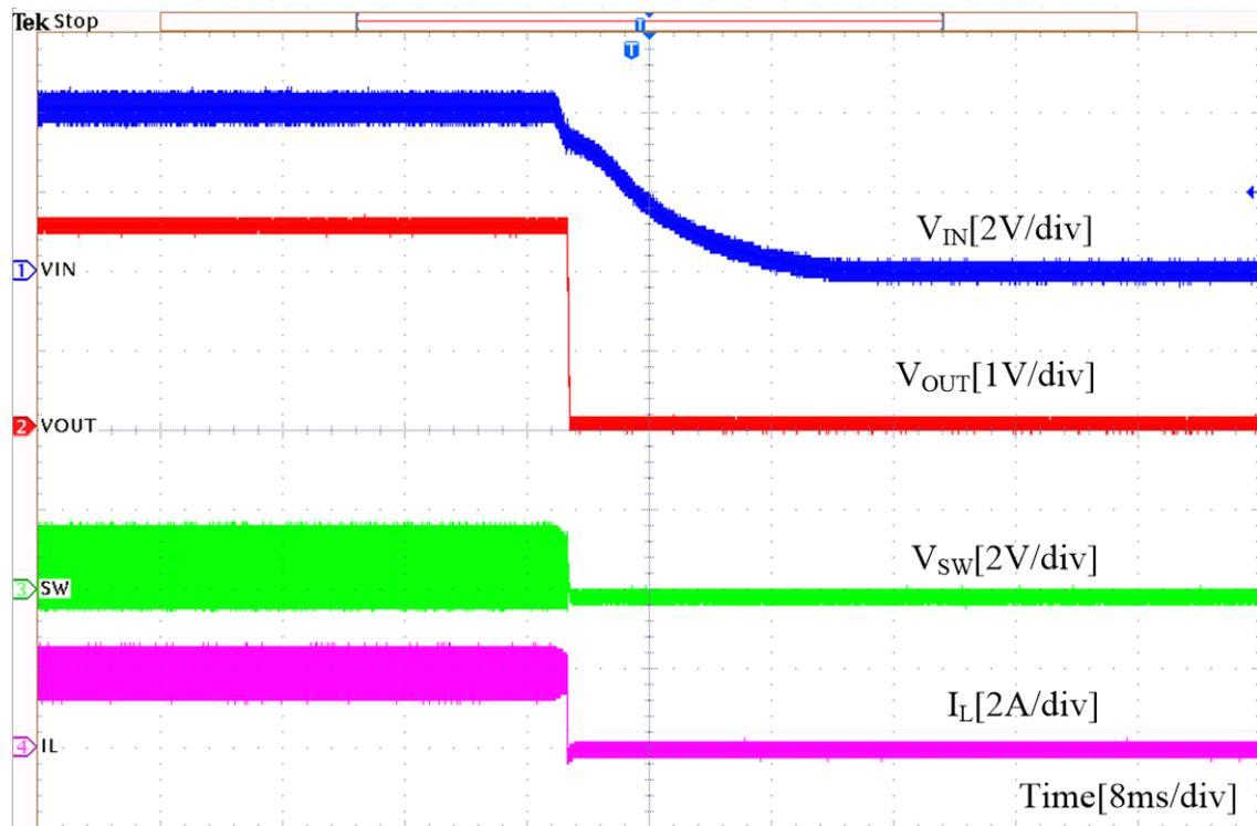
Figure 11. Shut Down, V<sub>IN</sub> = 4 V, I<sub>OUT</sub> = 2 A
