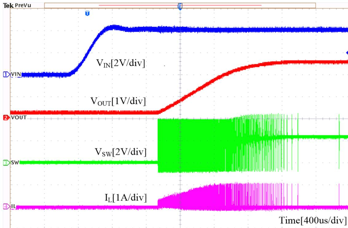
Figure 8. Start Up, V<sub>IN</sub> = 4 V, I<sub>OUT</sub> = 0 A
