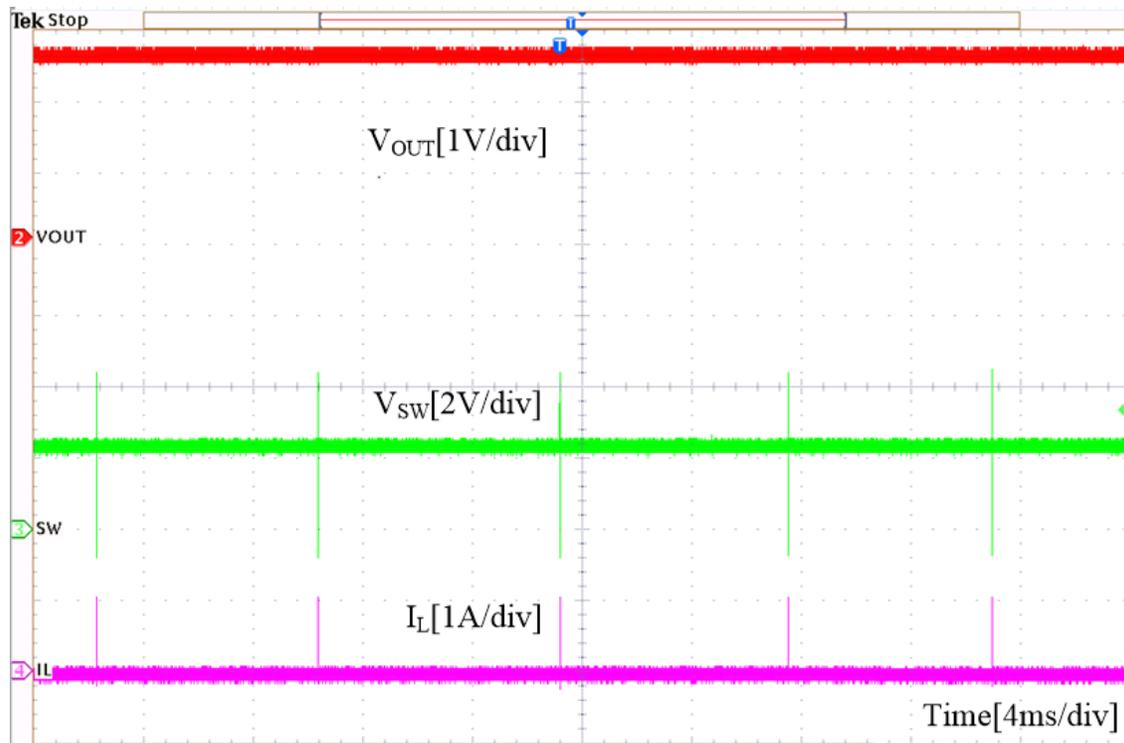
Figure 6. Steady State,  $V_{IN} = 4\text{ V}$ ,  $I_{OUT} = 0\text{ A}$
