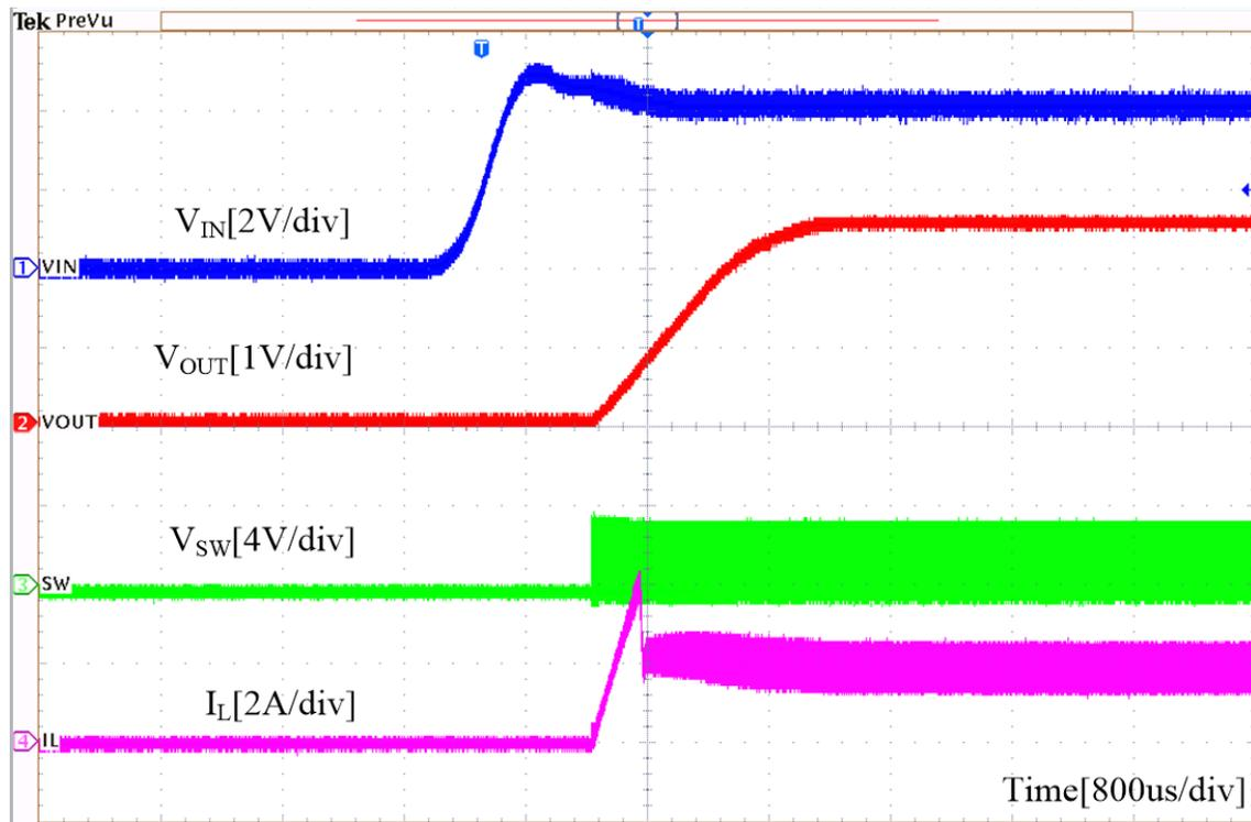
Figure 10. Start Up, V<sub>IN</sub> = 4 V, I<sub>OUT</sub> = 2 A
