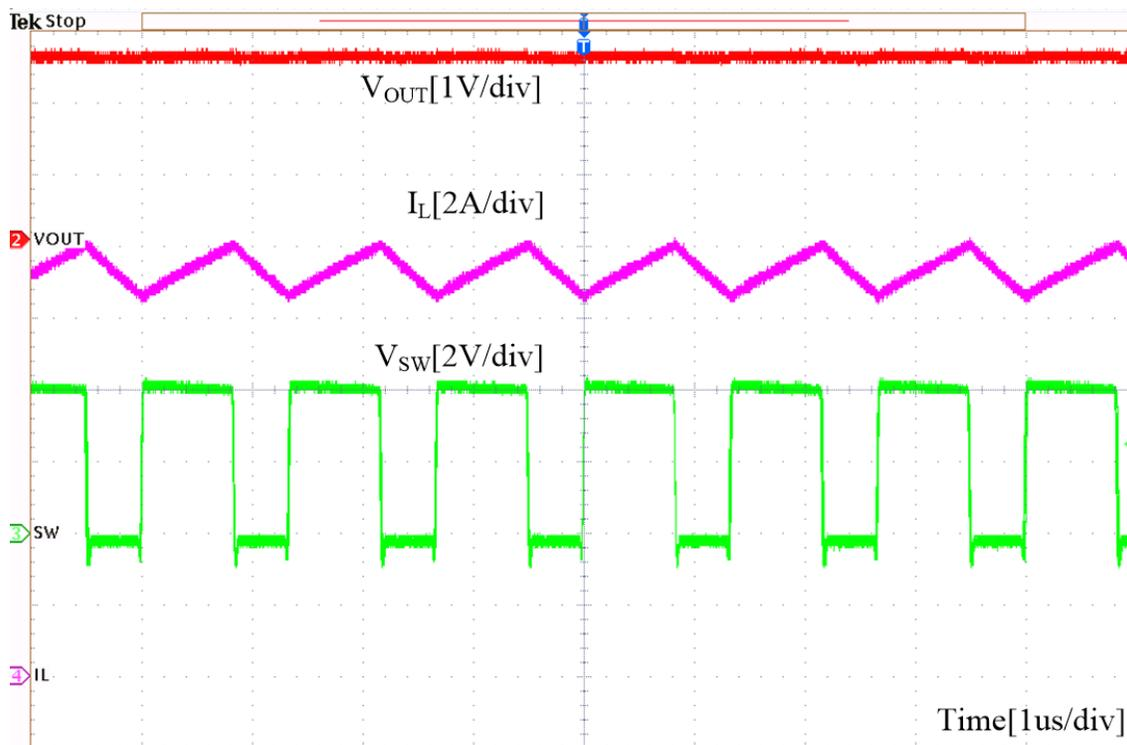
Figure 7. Steady State,  $V_{IN} = 4\text{ V}$ ,  $I_{OUT} = 12\text{ A}$
