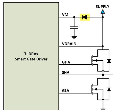
Figure 1. Modified Circuit with Diode
