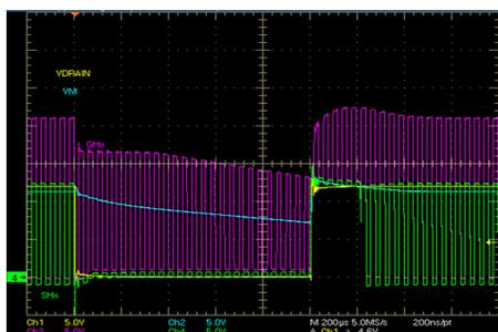
**Figure 3. Momentary Turn Off With Diode**
