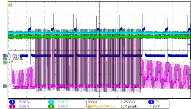
**Figure 4. Recurring Voltage Drops with Diode**
