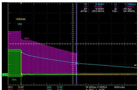
**Figure 2. Complete Turn Off With Diode**
