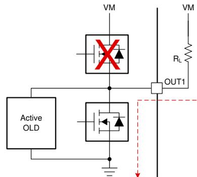
Figure 1-2. Active OLD for Load Connected to VM
