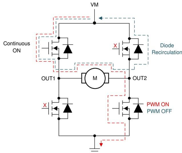
Figure 3-2. Forward Drive and Braking in Asynchronous Rectification
