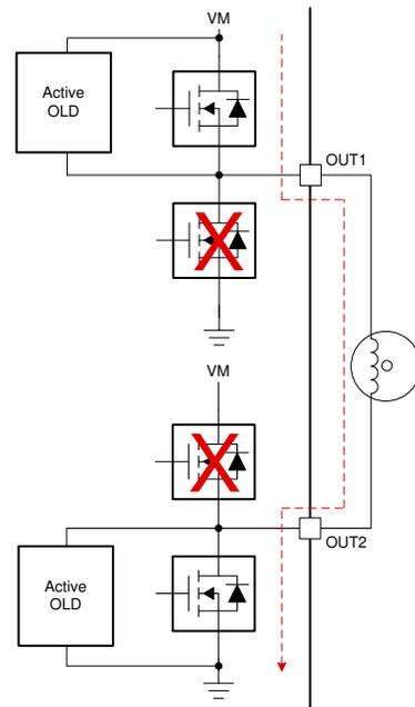
**Figure 1-6. Active OLD for Load Connected in H-Bridge Configuration**
