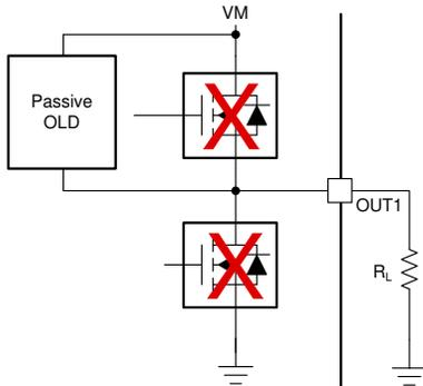
**Figure 1-3. Passive OLD for Load Connected to GND**
