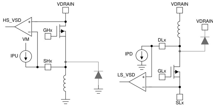
**Figure 2-4. Passive OLD Load Configurations not supported in a Brushless DC Gate Driver**
