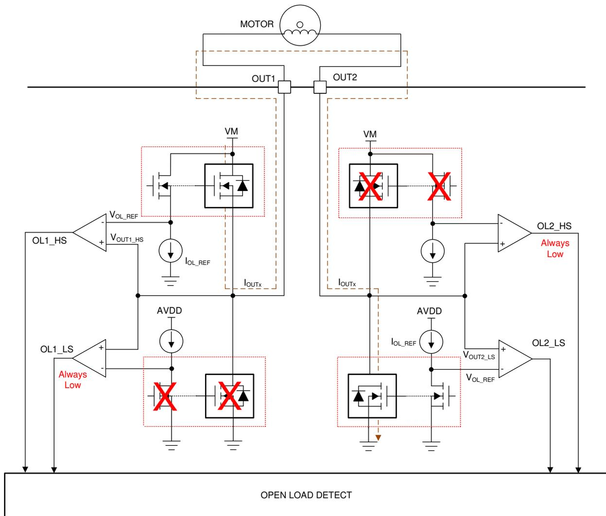
**Figure 3-3. Active OLD Circuit in Brushed DC Motor Integrated Drivers**
