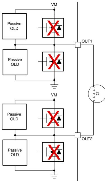
**Figure 1-5. Passive OLD for Load Connected in H-Bridge Configuration**
