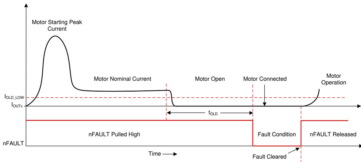
Figure 4-1. Low-Current Active OLD Operation
