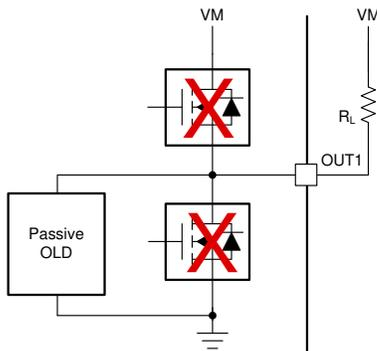
Figure 1-1. Passive OLD for Load Connected to VM
