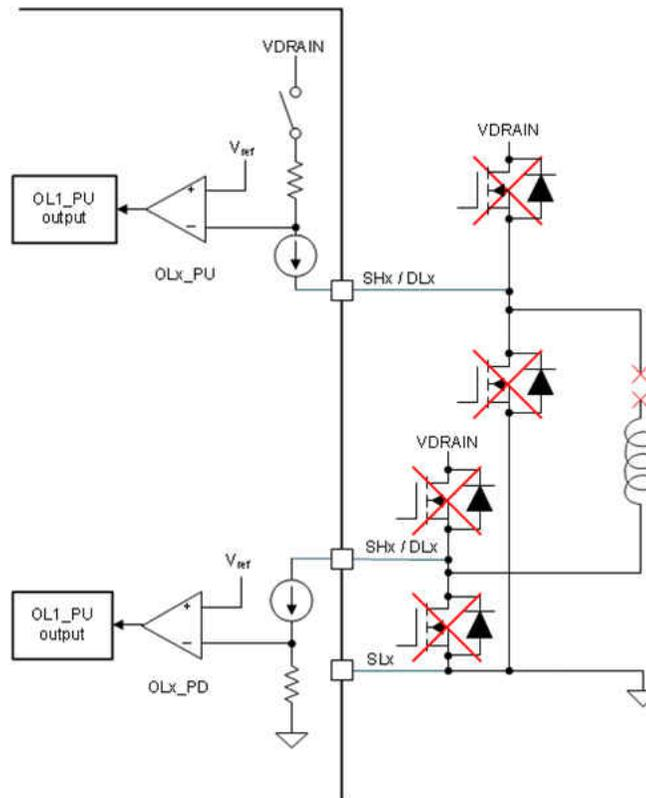
**Figure 2-3. Passive OLD Circuit in a Brushless DC Gate Driver**
