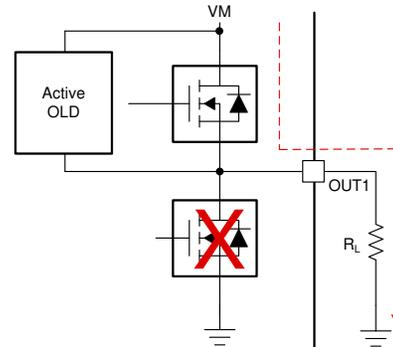
**Figure 1-4. Active OLD for Load Connected to GND**
