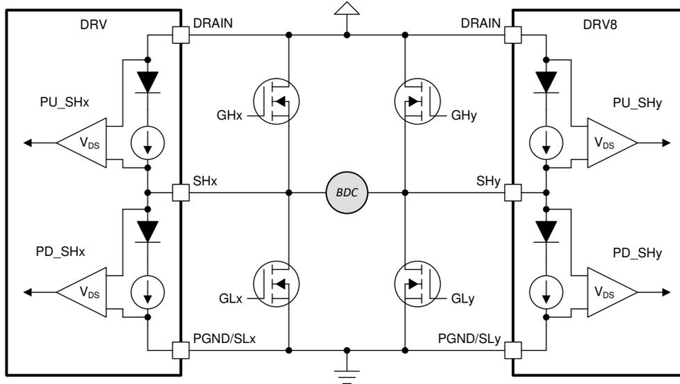
**Figure 2-2. Passive OLD Circuit in a Brushed DC Gate Driver**
